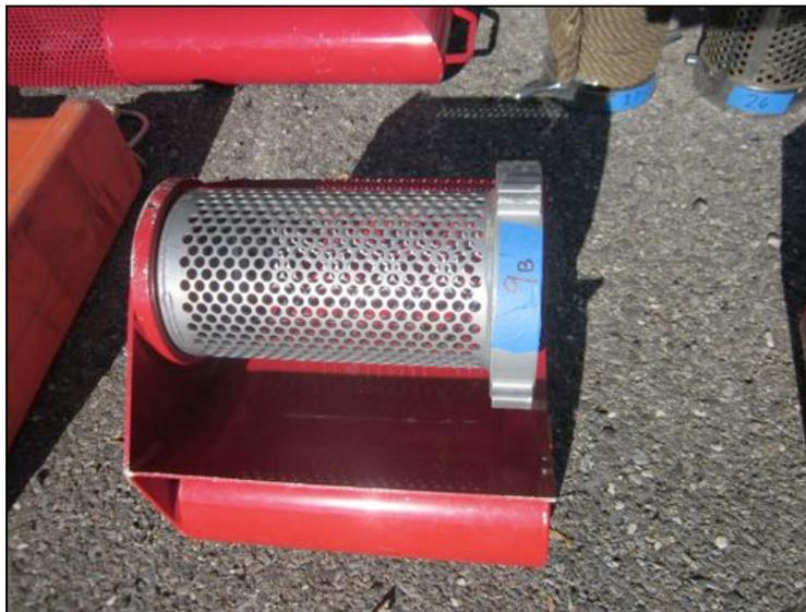
Figure 20: Kochek Self-Leveling Floating Strainer (FBS60). The strainer used a 6-inch barrel with nine hundred and fifty, 3/8-inch holes.
