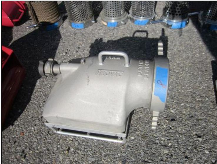
Figure 18: Firovac Low Level Strainer with 1.5-inch jet siphon (HVLL). The strainer had a cast housing; no tubing was used in the design.
