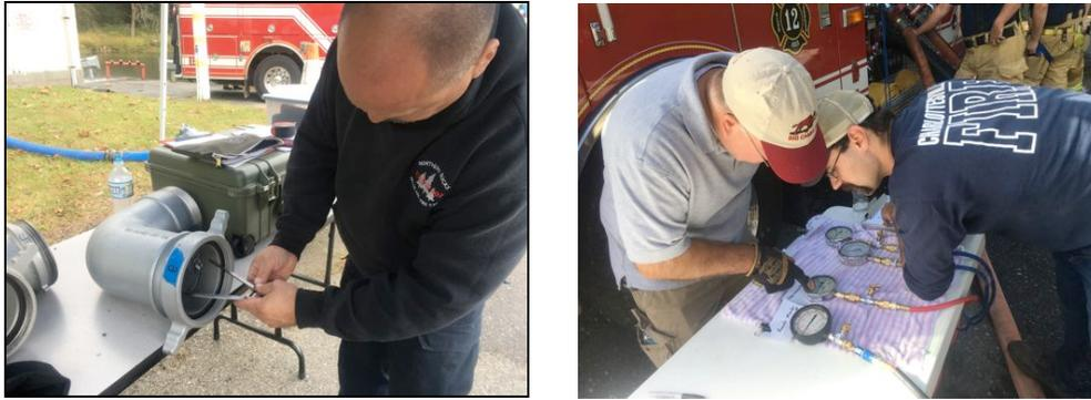
Figure 41: Henry Lovett, Jr. (left) collects physical data on a suction device while Alan Butsch and Andy Soccodato (right) record flow data.
