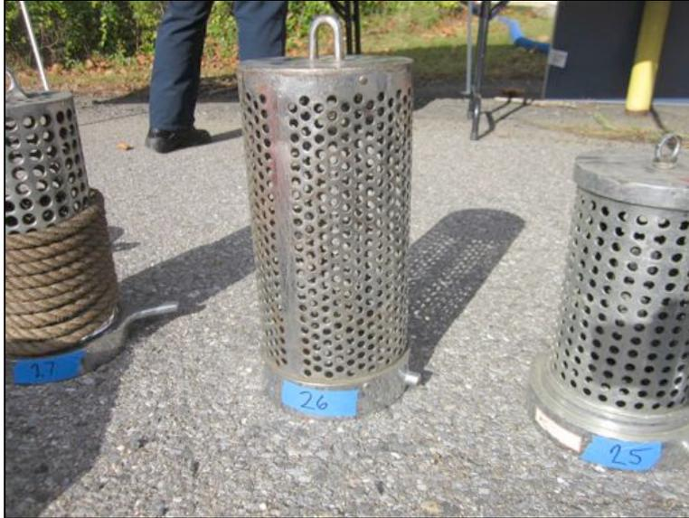
Figure 38: Barrel Strainer (Manufacturer and model unknown). The strainer had an outside diameter slightly greater than 7-inches and had approximately nine hundred sixty-eight, 5/16-inch holes. There were no holes on the end of the strainer. The holes all had sharp edges.
