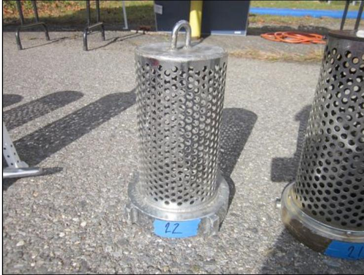
Figure 34: Kocheck Barrel Strainer (BS60). The strainer used 6-inch tubing with approximately seven hundred ninety-eight, 3/8-inch holes. There were no holes in the end of the strainer. The holes all had sharp edges.
