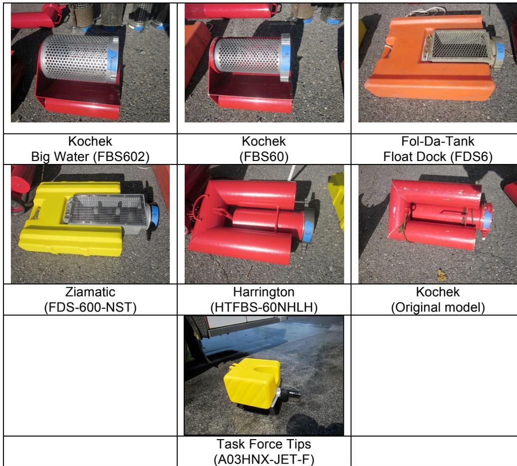
Figure 43: Seven different floating strainers were flow tested.
