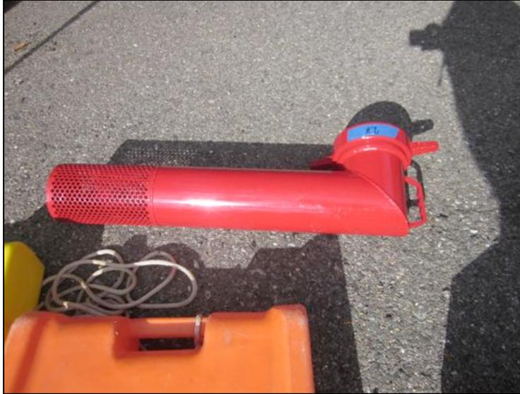
Figure 40: Kocek Ice Strainer (IS60). The strainer used 6-inch tubing and had approximately nine hundred fifty, 3/8-inch holes.
