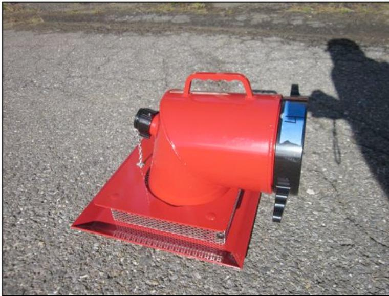
Figure 14: Kohek Big Water Low Level Strainer with 1.5-inch jet siphon (LL602). This strainer used an 8-inch tube.
