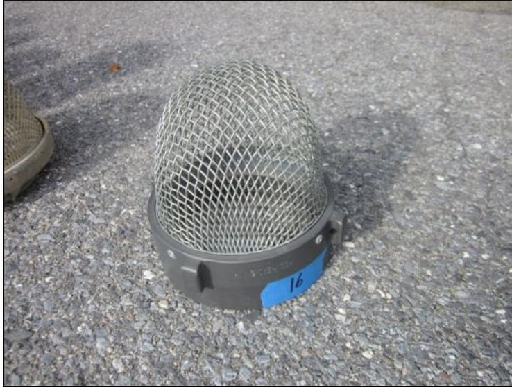
Figure 28: Red Head Style 139 Basket Strainer. The strainer used 1/4-inch wire mesh. Due to the design of the basket, there was limited uniformity in the mesh's hole size. The base of the screen had a 22-1/4-inch circumference.
