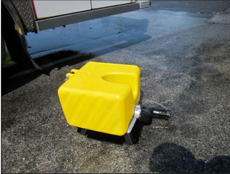
*Figure 25: Task Force Tips Floating Low Level Strainer Jet Siphon (A03HNX-JET-F). This is the same strainer as used in the low level strainer flow test. The strainer had a cast housing; no tubing was used in the design.*
