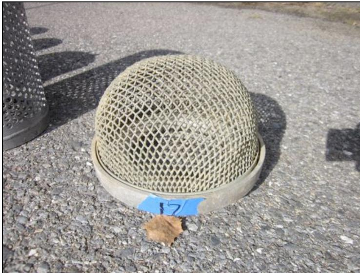
Figure 29: Basket Strainer (Unknown Manufacturer). The maker of this strainer was unknown, although the design resembles an Akron basket strainer. The strainer used 1/4-inch wire mesh. Due to the design of the basket, there was limited uniformity in the mesh's hole size. The base of the screen had a 29-inch circumference.
