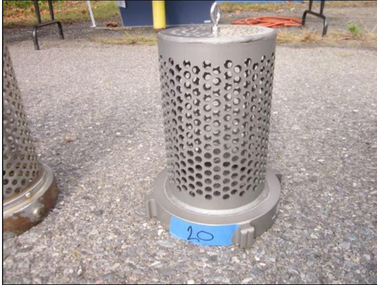
Figure 32: Harrington Barrel Strainer (HTBS-60NH). The strainer used 6-inch diameter tubing with approximately six hundred forty, 3/8-inch holes – some of which were in the end of the strainer. The holes all had sharp edges.
