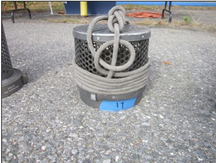
Figure 31: Akron Barrel Strainer Style 340. The strainer used a short, 8-inch diameter tube with approximately six hundred twenty-eight, 3/8-inch holes – some of which were in the closed end of the strainer. The holes all had sharp edges.
