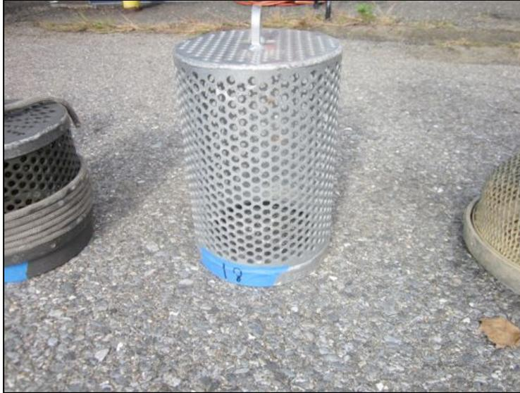
Figure 30: Kocheck Big Water Barrel Strainer (BS60-2). The strainer used an 8-inch diameter tube with approximately twelve hundred sixteen, 5/16-inch holes – some of which were in the closed end of the strainer. The holes all had sharp edges.
