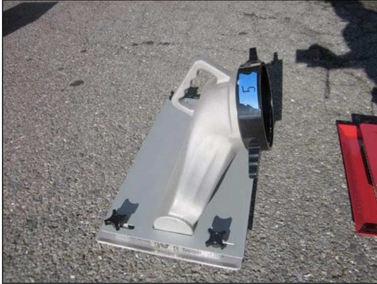
Figure 15: Ziamatic Low Level Strainer (QD-600-NST). The strainer had a cast housing; no tubing was used in the design.
