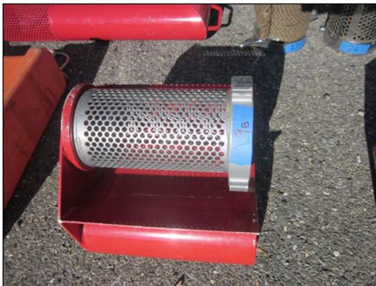
Figure 20: Kocheck Self-Leveling Floating Strainer (FBS60). The strainer used a 6-inch barrel with nine hundred and fifty, 3/8-inch holes.
