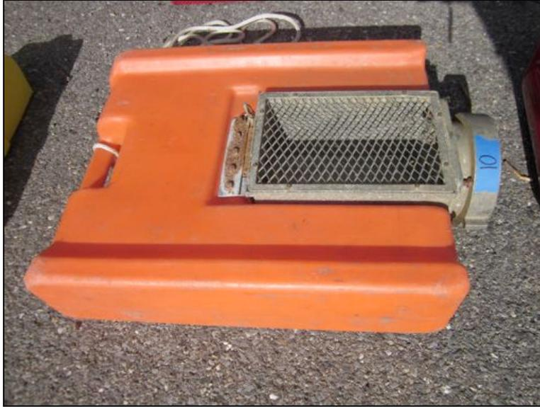
Figure 21: Fol-Da-Tank Float Dock floating strainer (FDS6). The strainer had a removable float that allows the strainer to be used as a box strainer. The strainer had approximately 90 square inches of open space in the expanded metal mesh.
