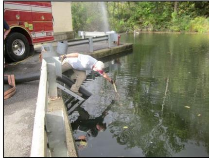
Figure 9: With the exception of the floating strainer tests, each strainer was deployed to a depth of 25-inches – meaning the top of the strainer was 25-inches below the surface of the water. A yardstick was used for measurement verification each time a strainer was deployed.
