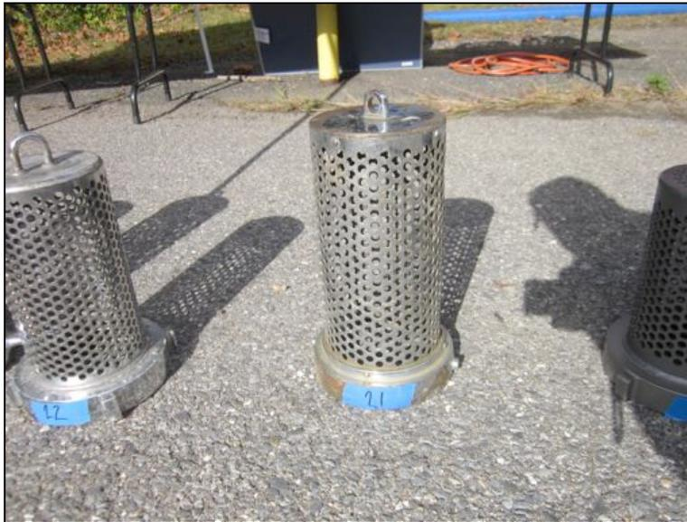
Figure 33: Barrel Strainer (Manufacturer and Model unknown – possible American LaFrance). The strainer came from a 1960's era American LaFrance pumper and had approximately seven hundred sixty, 3/8-inch holes. There were no holes in the end of the strainer. The holes all had sharp edges.
