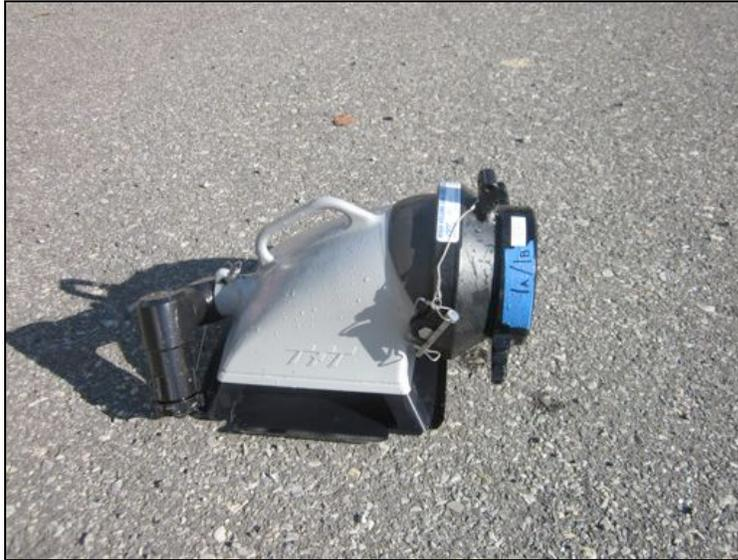
*Figure 11: Task Force Tips Low Level Strainer with 1.5-inch Jet Siphon (A03HNX-JET-F). This strainer came with a float attachment that was removed for the “low level” suction strainer test. The strainer had a cast housing; no tubing was used in the design.*
