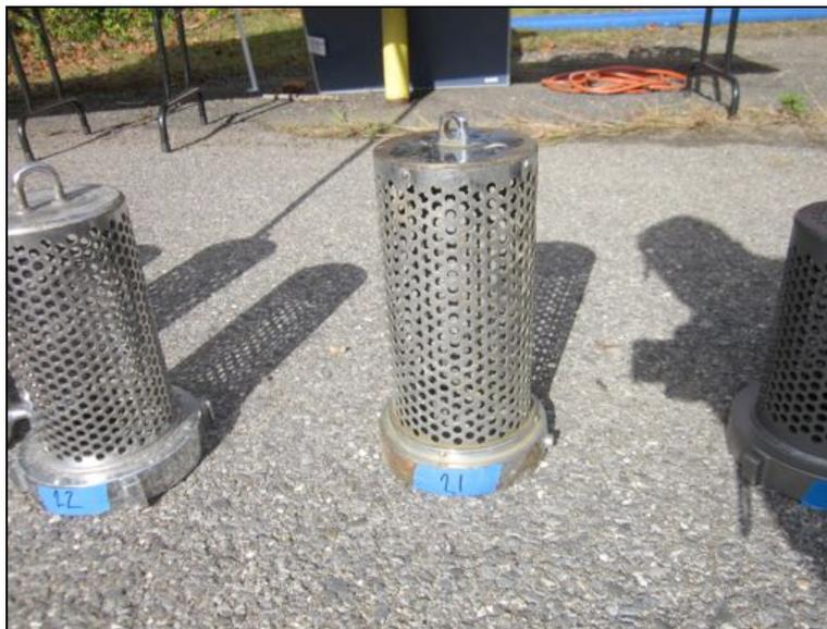
Figure 33: Barrel Strainer (Manufacturer and Model unknown – possible American LaFrance). The strainer came from a 1960's era American LaFrance pumper and had approximately seven hundred sixty, 3/8-inch holes. There were no holes in the end of the strainer. The holes all had sharp edges.
