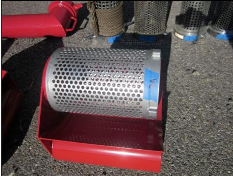
Figure 19: Kocheck Big Water Self-Leveling Floating Strainer (FBS602). The strainer used an 8-inch barrel with more than one thousand, 3/8-inch holes.
