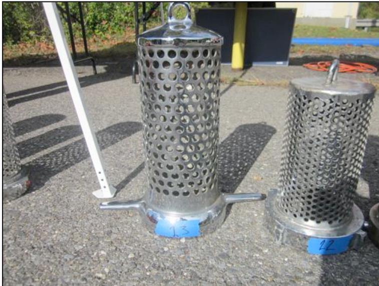
Figure 35: Barrel Strainer (Manufacturer and model unknown – possible Seagrave). The strainer came from a 1959 Seagrave pumper and had approximately three hundred sixty, 1/2-inch holes. There were no holes in the end of the strainer. The holes all had smooth edges.
