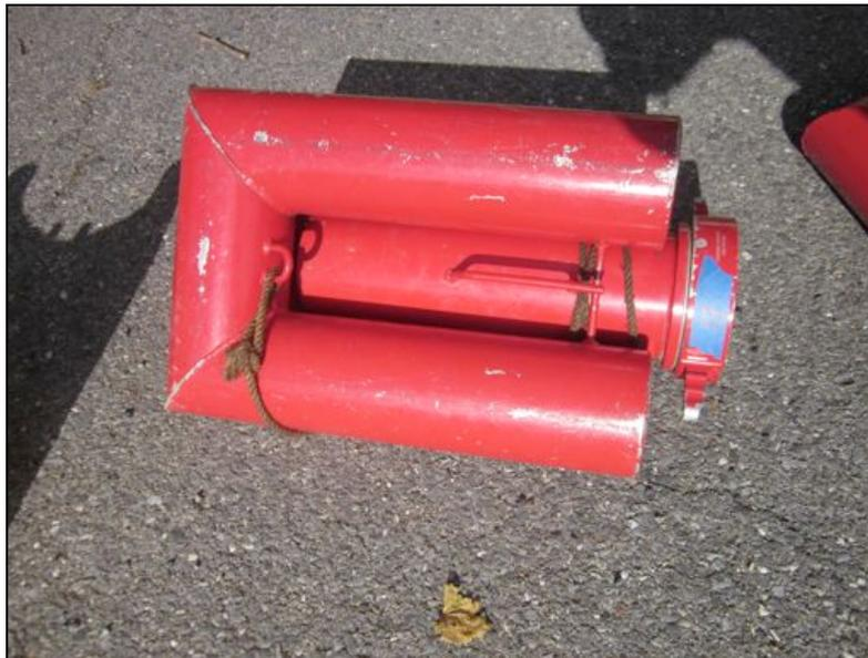
Figure 24: Kocheck Floating Strainer (original model). The strainer used 6-inch tubing with approximately four hundred forty-four, 1/2-inch holes.
