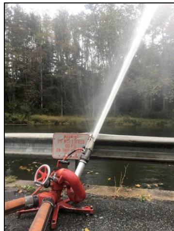
Figure 7: The Hose Monster was outfitted with a 2-1/2-inch orifice. The portable monitor was outfitted with an Akron flow test kit and 1-3/4-inch orifice.
