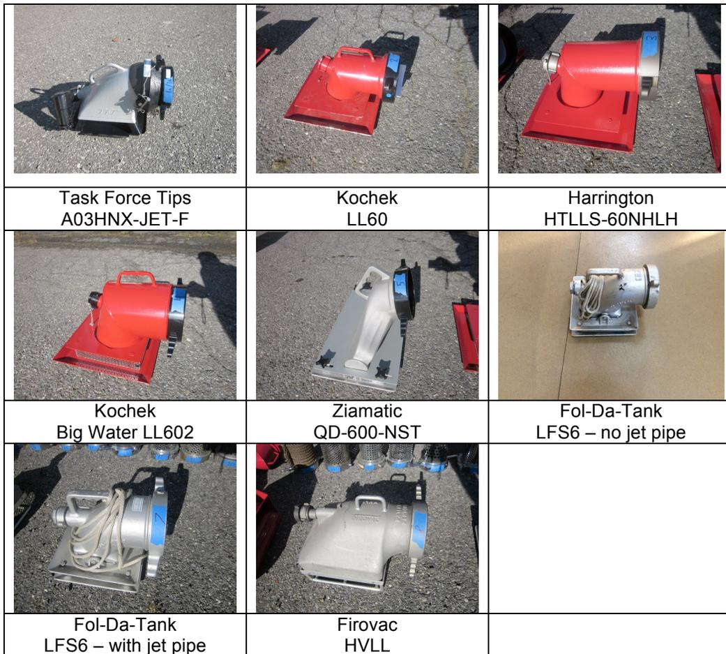
Figure 42: Eight low-level suction strainers were flow tested.
