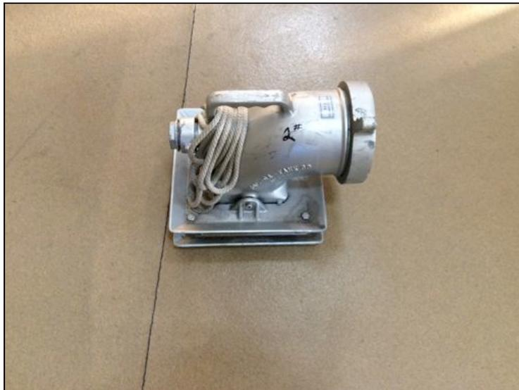
Figure 16: Fol-Da-Tank Low Flow Strainer (LFS6). This strainer had a fitting for a jet siphon connection, but no jet siphon pipe inside the strainer. The strainer had a cast housing; no tubing was used in the design.
