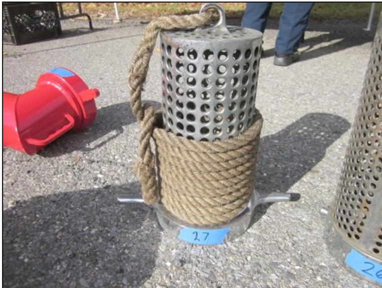
Figure 39: Barrel Strainer (Manufacturer and model unknown – possible Seagrave). The strainer came from a 1959 Seagrave pumper and had approximately three hundred ninety-two, 1/2-inch holes – some of those holes were in the end of the strainer. The holes all had smooth edges.
