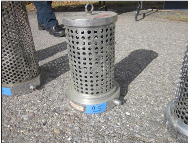
Figure 37: Powhatan Barrel Strainer (Model unknown). The strainer had approximately three hundred ninety-two, 3/8-inch holes. There were no holes in the end of the strainer. The holes had sharp edges and were not uniform in distribution.
