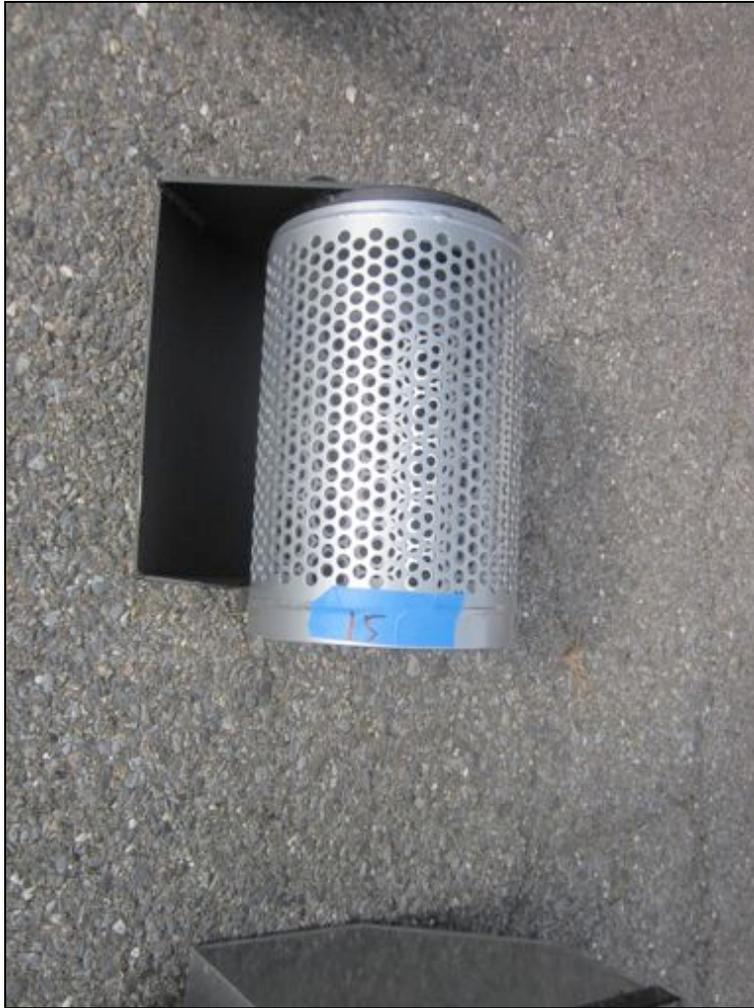
Figure 27: Kocheck Big Water Barrel Bottom Guard Strainer (BS602BG). The strainer used an 8-inch barrel with more than one thousand 3/8-inch holes. This is the same barrel as was used on the Big Water Self-Leveling Strainer.
