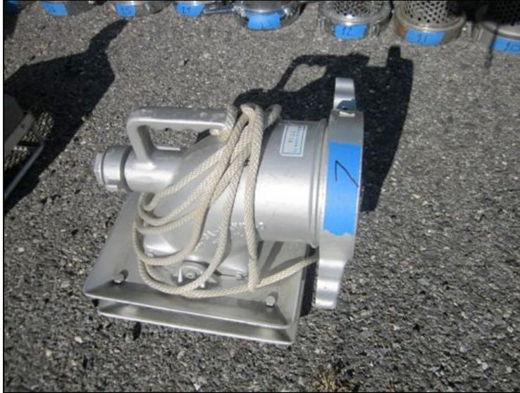
Figure 17: Fol-Da-Tank Low Flow Strainer with Jet Boost (LFS6). This strainer had a fitting for a jet siphon connection and also had a jet siphon pipe inside the strainer. The strainer had a cast housing; no tubing was used in the design.
