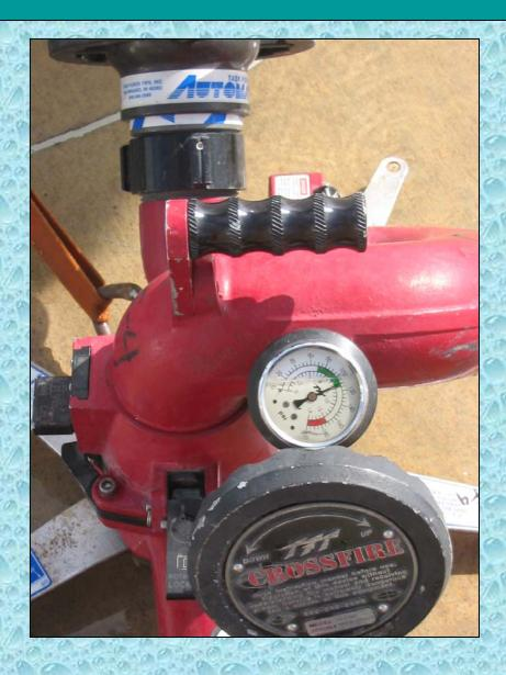
The pressure gauge reads above 100 psi, thus we know that the automatic nozzle is fully-open and flow has been maximized at 1250 gpm.
