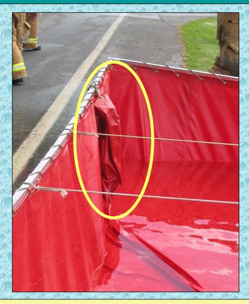
This is the correct position of the drain when tied up for storage. When filled with water, the water pressure will help keep the drain closed.
