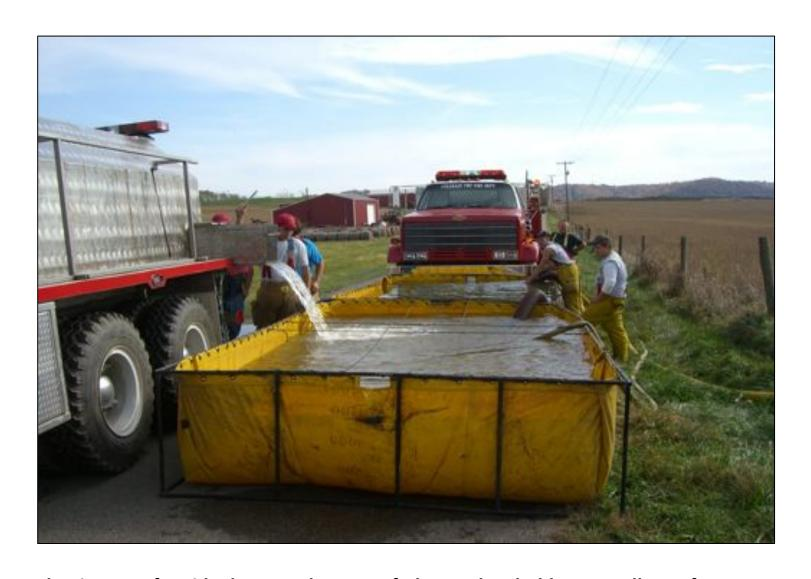
Colerain FDs 8 ft. wide dump tanks are 14 ft. long. They hold 2,000 gallons of water. A more desirable size may be 3,000 gal. <u>but</u> if that 13 ft. X 13 ft. square tank hangs down in the ditch it may only hold 1/2 its capacity or 1,500 gallons of water! Notice the water level in these tanks shows the crown or drainage slope in the road pavement. Notice the stream of water from the tanker dump valve. Should they stop dumping and move on to fill site?
