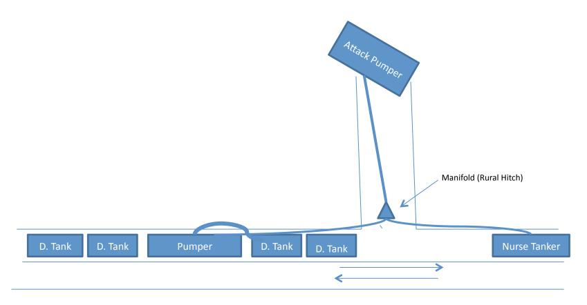
Rectangular dump tanks make it possible to keep the water supply set up in a single traffic lane. There can be floating pumps in the two rear dump tanks to push water to the drafting tank. There is only one section of jet siphon tube needed for this set up. Only one pumper needed at the dump site. Rear dump tankers can dump when coming from either direction without needing to turn around. **Water supply set up can be simple and standardized!** Can you think of other variations to this set up?
