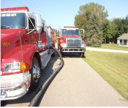
The Porter Kingston Fire District in Delaware County, Ohio uses dump tank flanges to draft water through the side of a dump tank instead of running suction hose up over the top.
