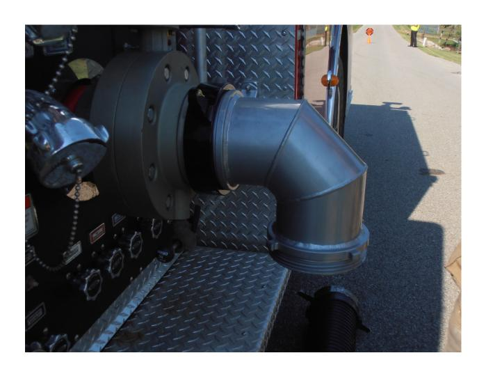
The 90 degree elbow guides the suction hose right down under the running boards and along the tires of the pumper right up to the corner of the dump tank.
