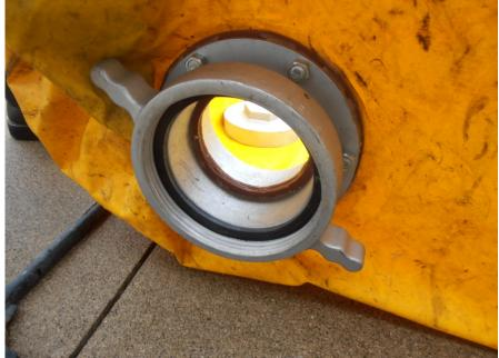
Notice the brown gasket material and silicon caulking which have not yet been trimmed flush to allow a smooth flow of water. This can be done with a razor blade knife.
