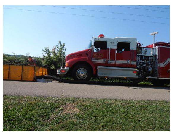
A support was needed for the suction hose to prevent the low level strainer from tilting up in the dump tank. This also helped in turning the female swivel fitting when hooking up the suction hose.
