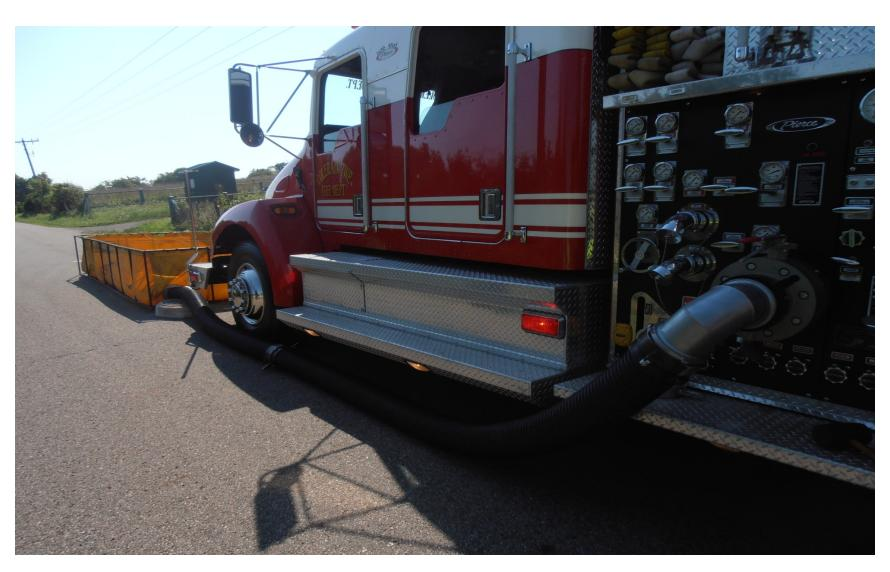
Even though this pumper is longer than average (17 ft. from suction outlet to front bumper), two sections of suction hose can easily reach the dump tank in front of the pumper with safety space to spare. Two sections can also reach the back of the truck (14 ft.) It is easy to see when water from the dump tank seeks its own level in the suction hose that there is only 2-3 ft. from the water level to the pump inlet. It takes less than 5 seconds to prime the pump
