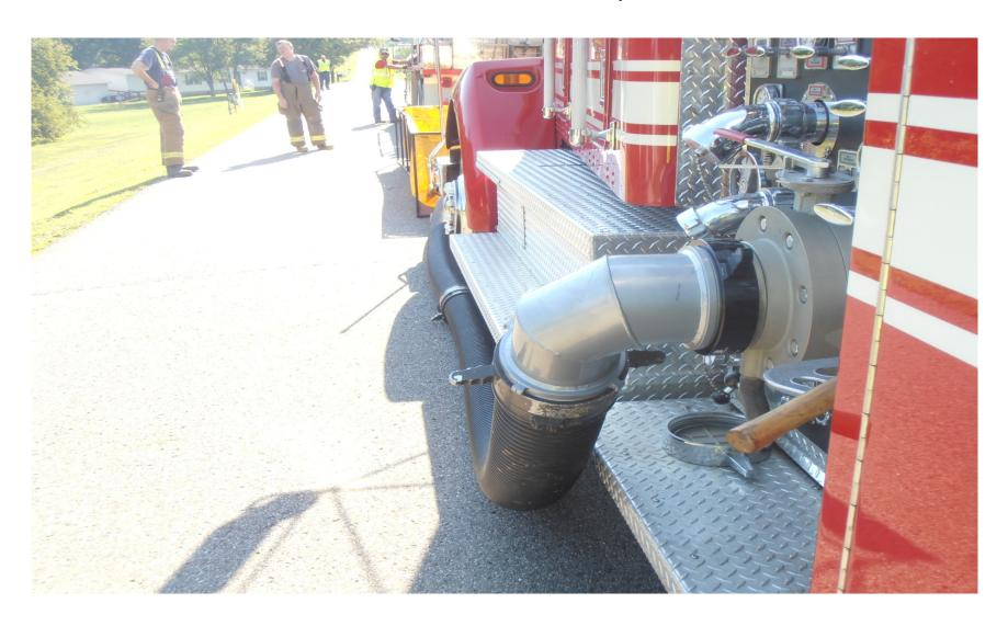
The 90 degree elbow holds the suction hose next to the pumper to allow tankers to pass by when using the single lane water supply setup on narrow roads.
