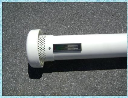
First up was the installation of the site vent unit. We like to use these assemblies on underground tanks because they provide a visual indicator above ground if the tank is full or not.
