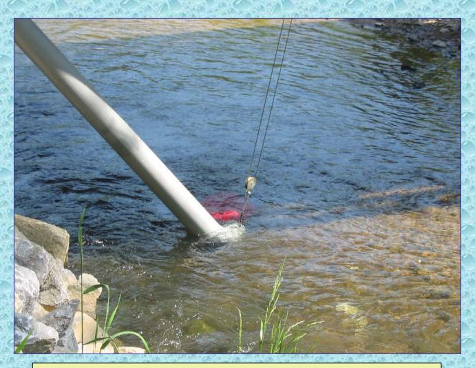
When lowered, the hoisting system places the strainer into the water at just the right depth for drafting. The teardrop strainer is designed for taking suction in moving water.
