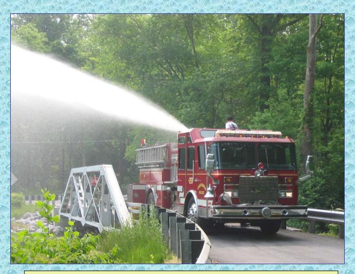
The flow test confirms the working condition of the DFH installation and should be required of every installation before acceptance of the work.
