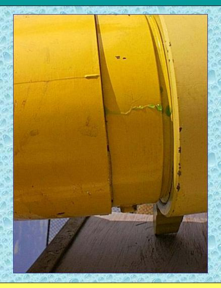
The air leak in the original head occurred at the interface between the metal and the PVC. Basically, the PVC cracked and could not be repaired.
