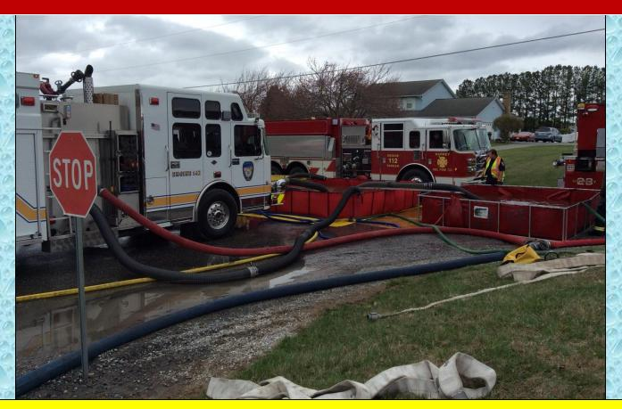
At the 90-minute mark flow was moved to 1500 gpm, where it remained for the remainder of the drill. Engine 142 used multiple suction lines to support the 3-dump tank operation.
