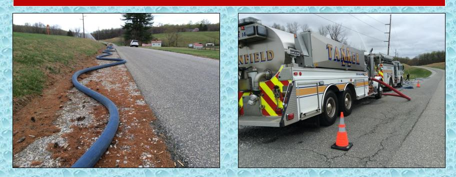
When Tanker 14 arrived on the scene the rig positioned near Engine 141 and supplied tank water using the "attack tanker" concept. The tanker driver then took the supply line from the rural hitch into Tanker 14's pump to complete the evolution.
