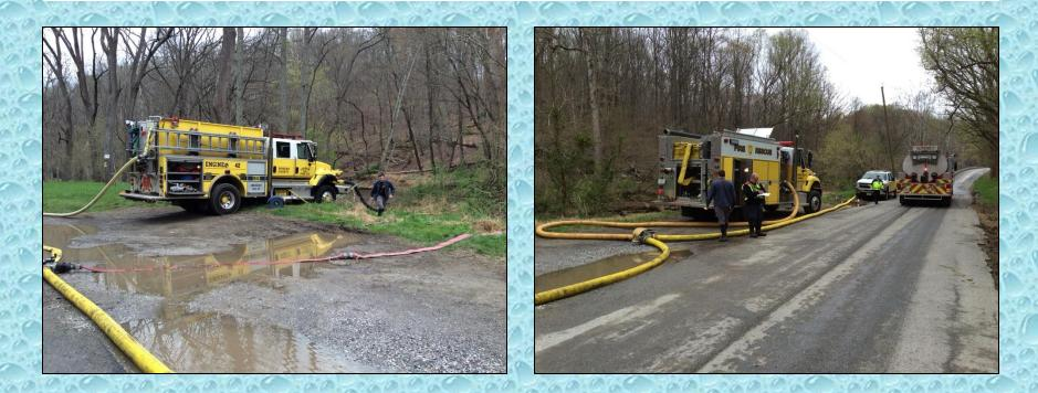
Lisbon Water Supply 42 (1250 gpm) [left] and Pleasant Valley Special Unit 6 (1500 gpm) [right] drafted from the river and operated independent tanker loading stations.
