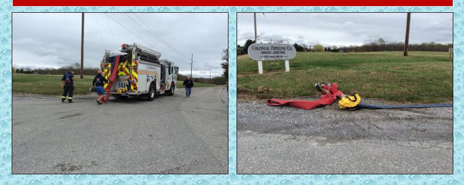
The drill started with crews executing a rural hitch operation using a 5" doubleclappered siamese. Winfield Engine 141 arrived on the scene and laid out several hundred feet of of 5-inch supply line before going to work as the attack pumper.
