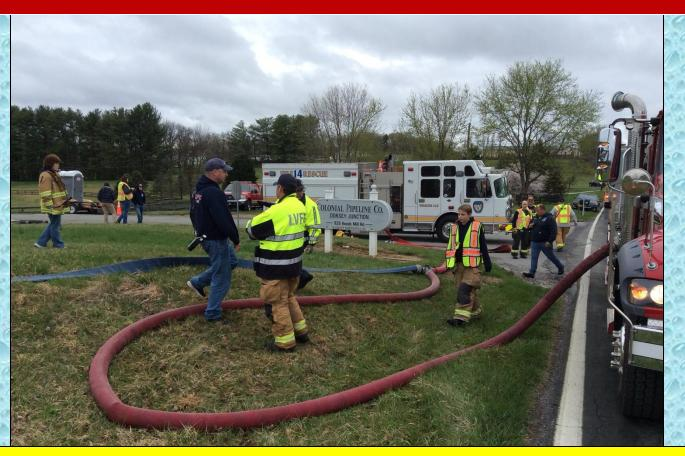
Around the 8-1/2-minute mark, the rural hitch was operational at 500 gpm. Crews then worked to expand the ability to have multiple tankers support the operation.
