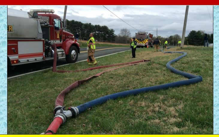
Additional arriving tankers supported the rural hitch and crews set up additional clappered Siamese devices.
