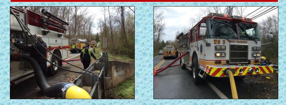
The pumper also drafted from the bridge-mount dry fire hydrant and was able to load tankers at the 1000 gpm target rate.
