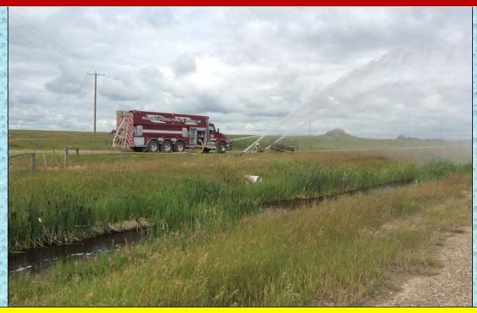
At the peak flow of the operation, two, TFT Blitzfires and one, 125 gpm TFT bumper turret were used at Tender 58.
