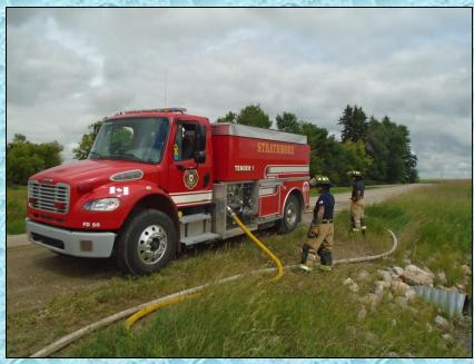
Tenders were loaded in a variety of ways with some taking in additional water through their fire pump.
