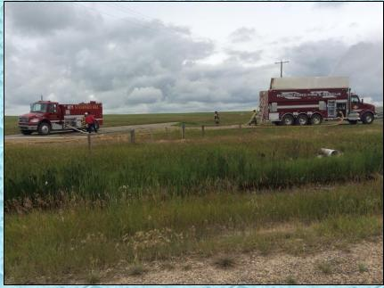
Siksika Tender 1 (left) and Strathmore Tender 1 (right) continue to support the rural hitch operation at 625 gpm while work continues on the dump site.
