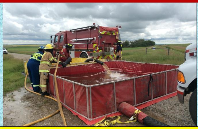
Around the 60-minute mark, a second dump tank (2500 gal) is operational and water transfer operations are underway.
