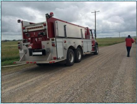
Standard Tender 77 arrived around the 7-minute mark and supplied water to Tender 58 using the rural hitch and some 65 mm (2-1/2") hose.
