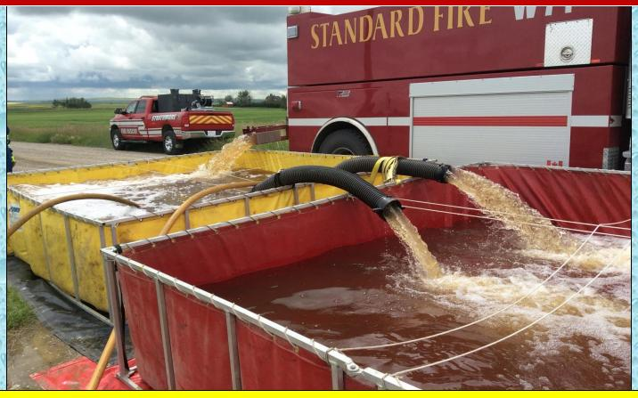
Twin, 5-inch jet siphon water transfer devices were used to support the drill. The devices were both powered by Engine 34.
