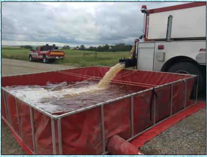
Around the 55-minute mark, the first load of water is dumped in the dump tank and the transition from rural hitch to dump tanks ops is completed.
