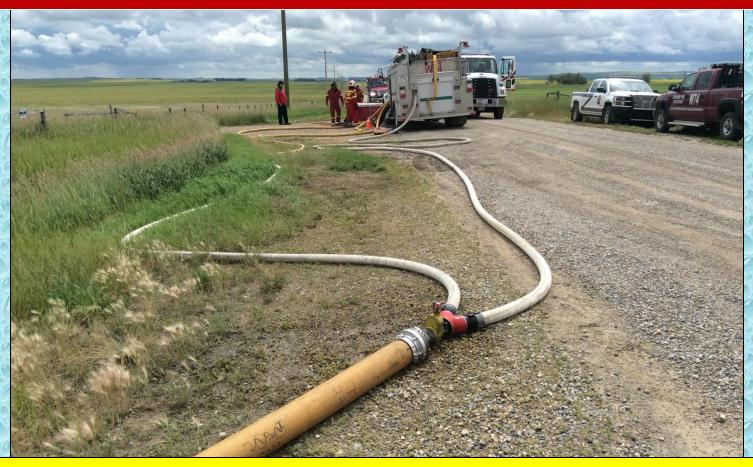
Around the 90-minute mark, Engine 34 supplied a second line to the rural hitch appliance and flow was pushed to over 1000 gpm.
