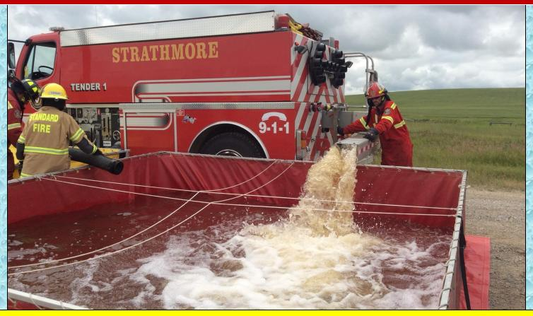
Dump tank operations continue and crews work to expand the site to include a second dump tank.
