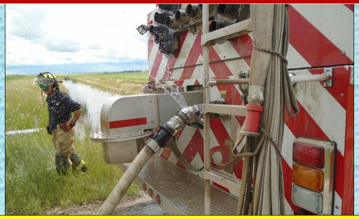
3-inch cam lock style fittings were used on all the tenders that were equipped with threaded fill connections.
