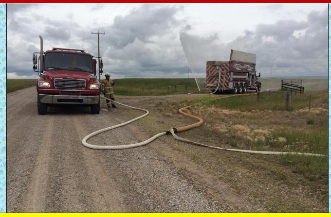
As Tender 71 takes over the rural hitch, flow is moved to 500 gpm. Two more tenders are enroute and a dump tank operation is being built.
