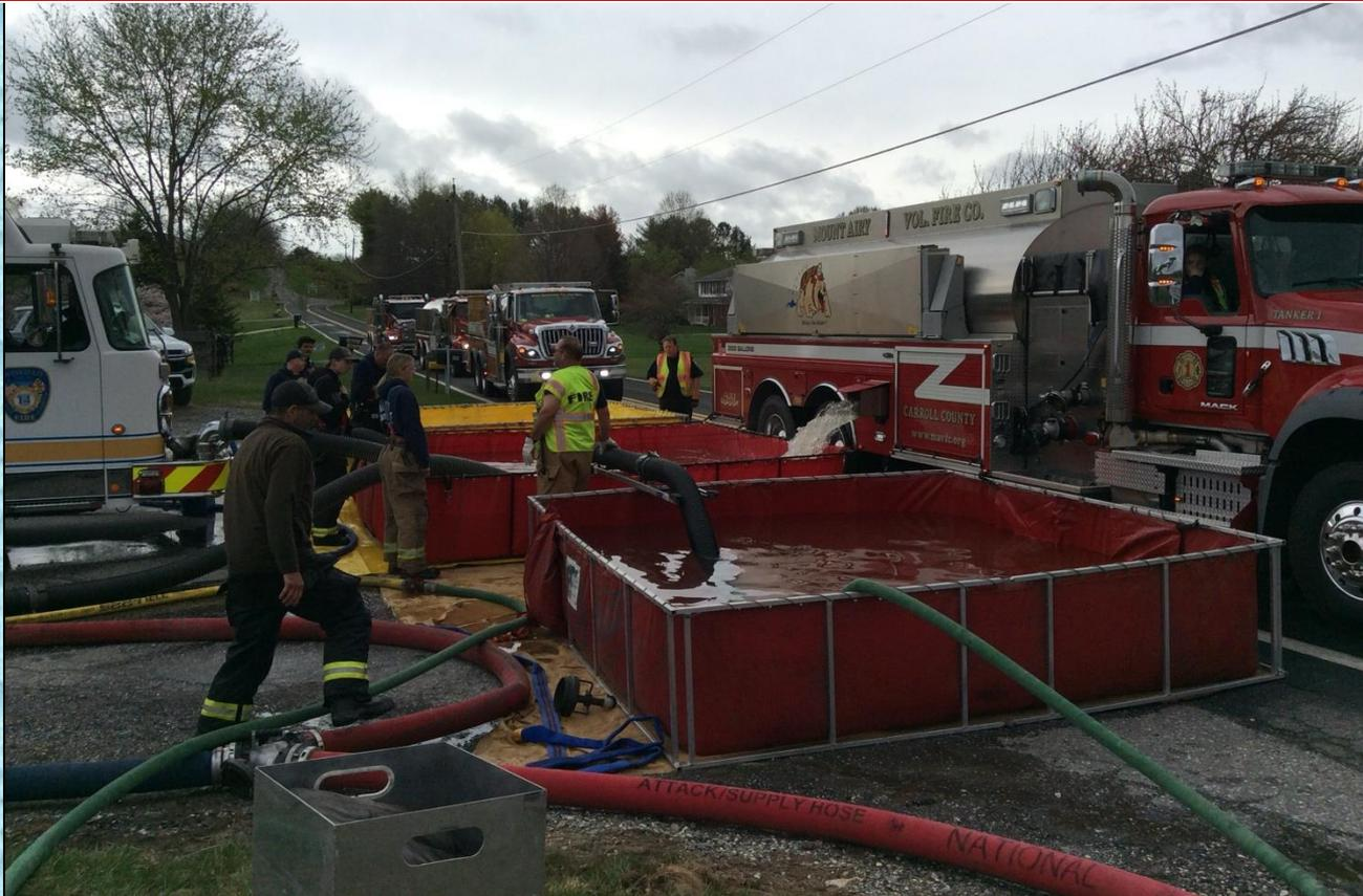
At the 51-minute mark, the operation transitioned to a dump tank operation.
