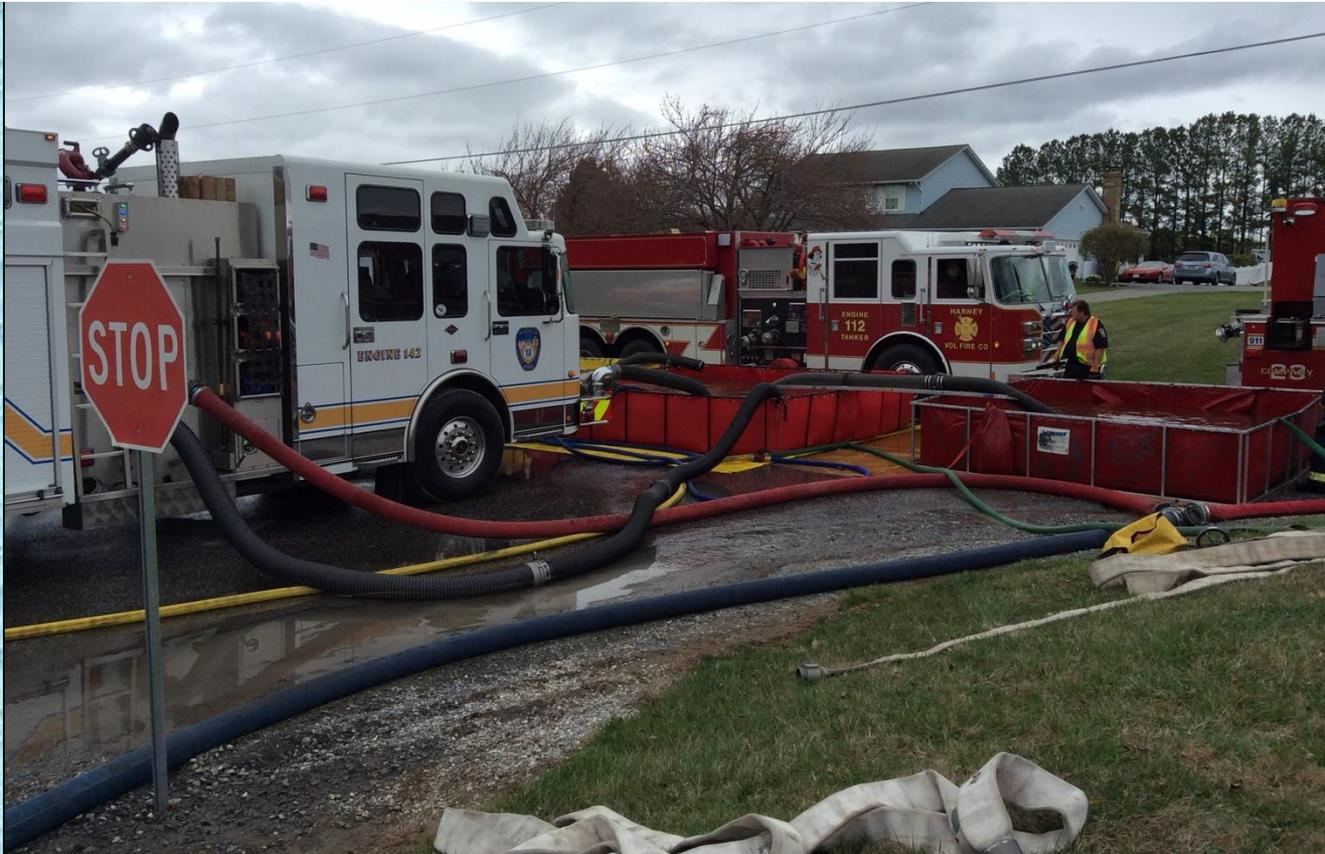
At the 90-minute mark flow was moved to 1500 gpm, where it remained for the remainder of the drill. Engine 142 used multiple suction lines to support the 3-dump tank operation.
