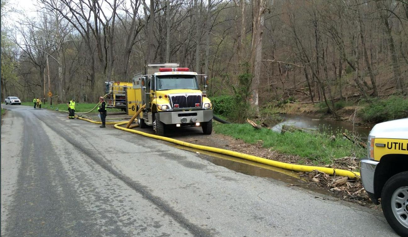
The river fill site provided plenty of water and access for two pumpers to set up and load tankers.
