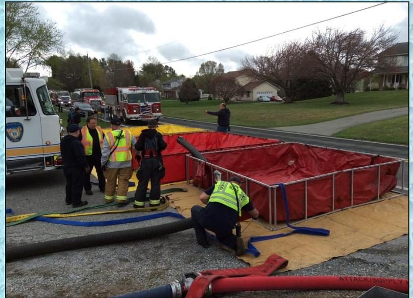
Meanwhile, back out at the rural hitch, tankers continued to pump off their water while crews worked to get a dump tank operation up and running. Around the 45-minute mark flow was moved to 1000 gpm using the rural hitch.
