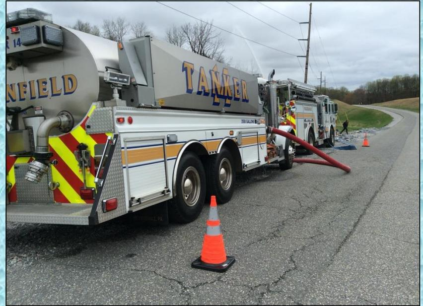
When Tanker 14 arrived on the scene the rig positioned near Engine 141 and supplied tank water using the “attack tanker” concept. The tanker driver then took the supply line from the rural hitch into Tanker 14’s pump to complete the evolution.
