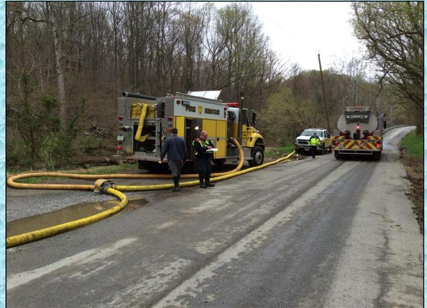
Lisbon Water Supply 42 (1250 gpm) [left] and Pleasant Valley Special Unit 6 (1500 gpm) [right] drafted from the river and operated independent tanker loading stations.
