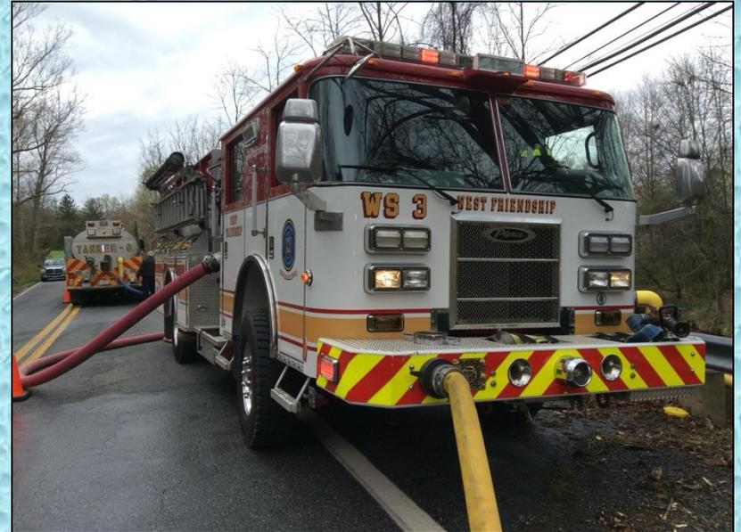
The pumper also drafted from the bridge-mount dry fire hydrant and was able to load tankers at the 1000 gpm target rate.
