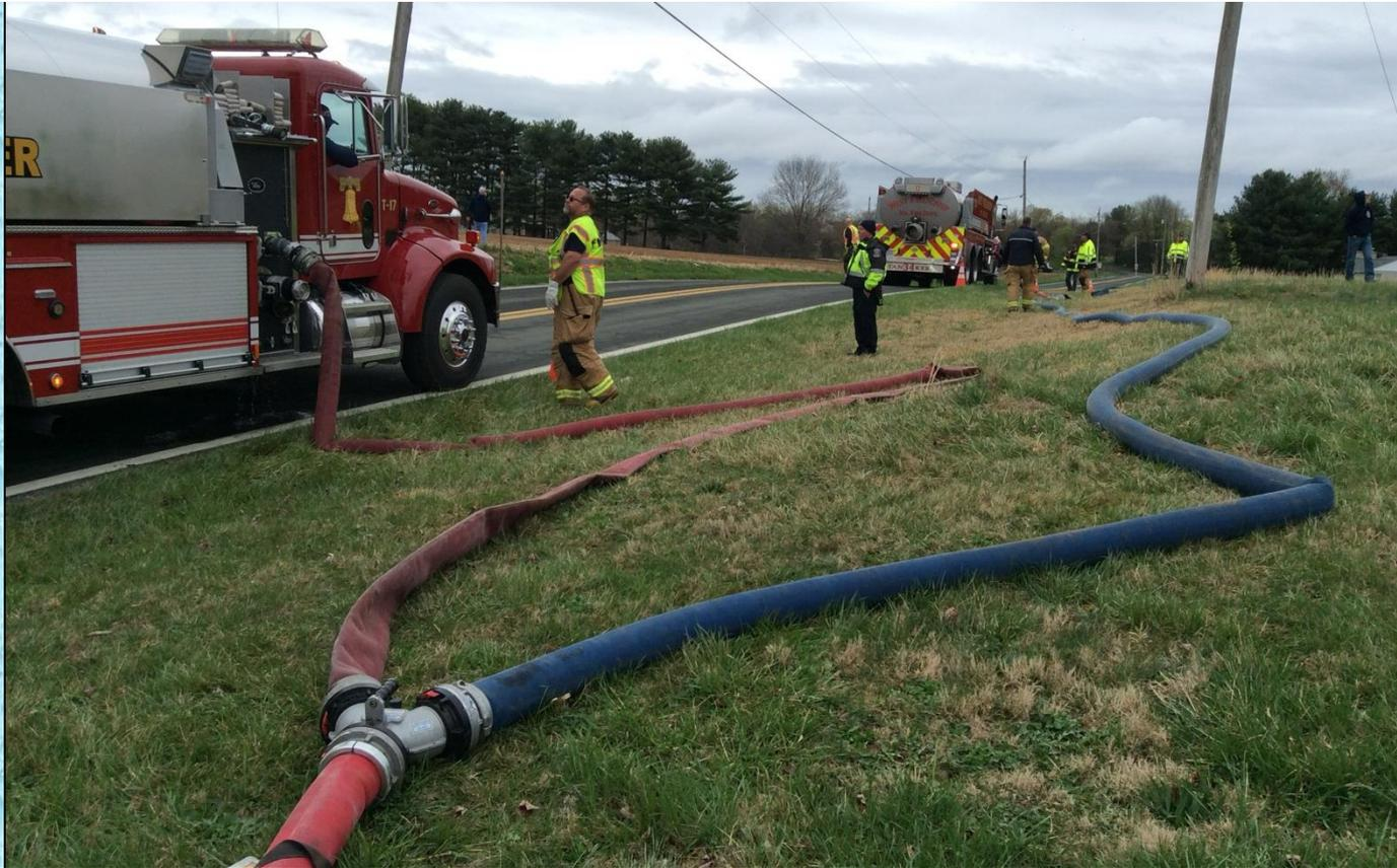
Additional arriving tankers supported the rural hitch and crews set up additional clapped Siamese devices.
