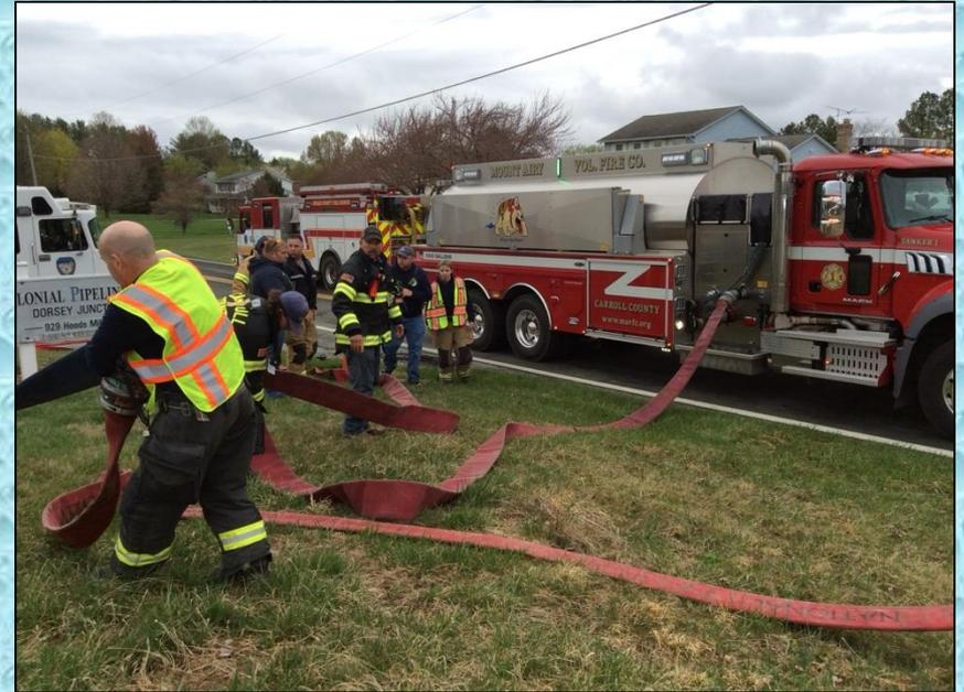
Tanker 14 (left) arrived next and proceeded back the lane to co-locate with Engine 141 and go to work as the “attack tanker.” Tanker 1 (right) arrived next and went to work supplying the rural hitch.
