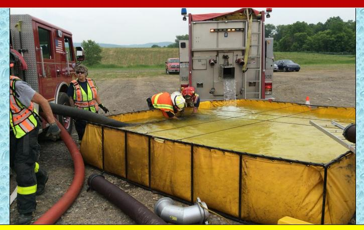
Shortly after dump site operations began the folks changed out an underperforming suction strainer and put a 6-inch TFT low-level strainer in its place. They did this without ever shutting down the flow.
