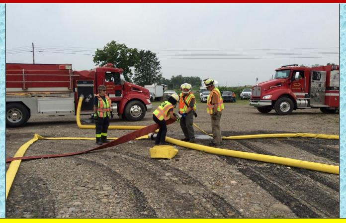
The dump site crew is shown here around the 12-minute mark connecting the pumper's supply line (red) to the Siamese in preparation for the transition.
