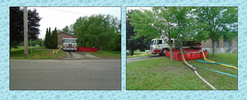
Athens Twp 24E1 (1500 gpm) was used at the creek fill site. Three portable pumps were used to support and "open relay" operation where water was pumped from the creek into a dump tank and then drafted and loaded into tankers.
