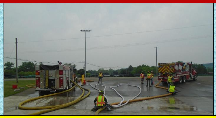
Sayre Engine 2 (1750 gpm) took in 5-inch supply lines from the fire hydrant and was able to support two loading stations on the firehouse apron. The fire hydrant provided over 2000 gpm which allowed Engine 2 to then load two tankers at a time when the need arose.
