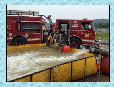
About 20-minutes later the crew was able to add a second, 6-inch suction line; it was outfitted with a barrel strainer. The additional suction line allowed the pumper to move to a 1500 gpm flow and run three jet siphon devices.
