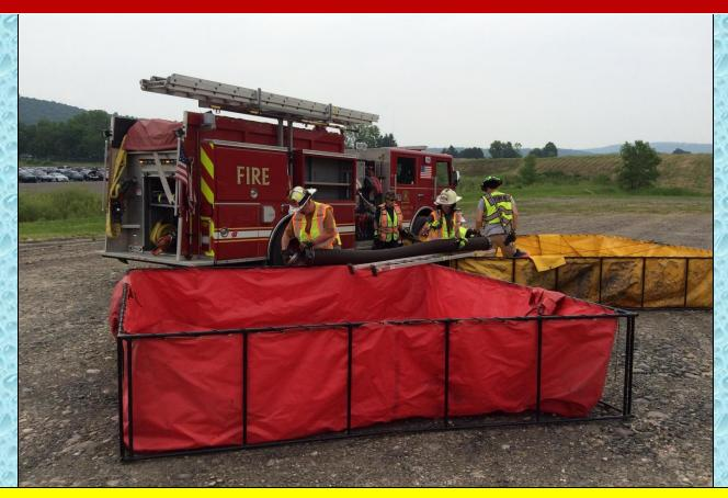
The dump site crew went to work collecting equipment and building out a 2dump tank arrangement in preparation for transitioning over from the rural hitch operation.
