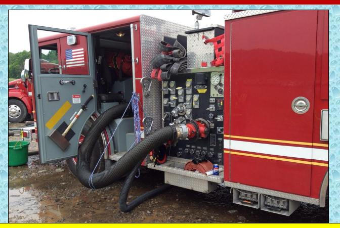
The three suction lines were a big improvement to the overall performance for this 25-year old 1500 gpm pumper.
