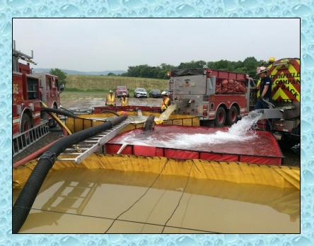
By the one-hour mark flow was at 1000 gpm and jet siphon control was removed from the pump operator and placed next to the dump tanks.
