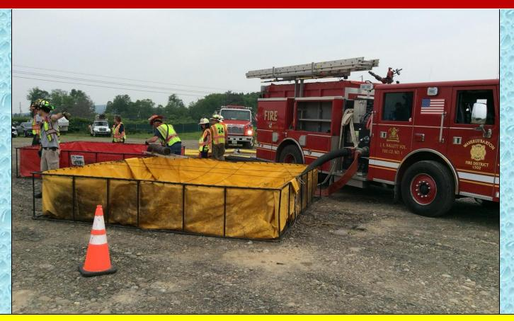
With two dump tanks set and the pumper ready to draft, all that is needed is a load of water.
