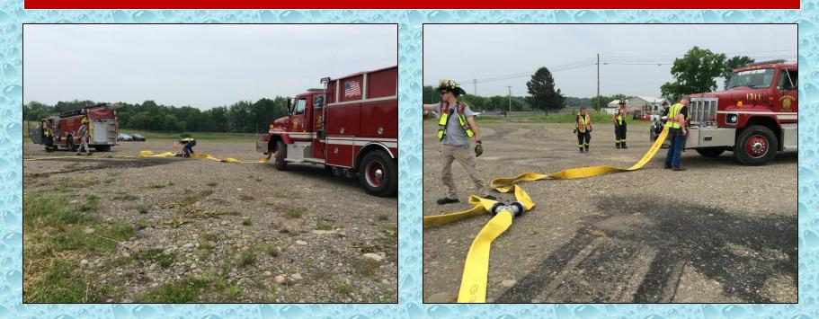
The drill started with crews executing a rural hitch operation using a 5" doubleclappered siamese. Tanker 1311 arrived on the scene and went to work supporting the siamese that was already in place simulating an attack pumper that had laid out 5-inch supply hose. At the 2-minute mark, Tanker 1311 started water flow at around 500 gpm.
