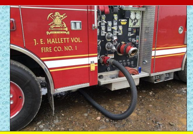
Also around the one-hour mark a 2-1/2-inch suction line (with a low-level strainer) was added to the operation from the driver's side of the rig.
