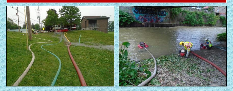
The combined flow of the portable pumps was enough to allow the fill-site pumper to load tankers at a rate of just under 1000 gpm.
