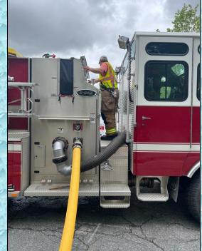
Lyme Engine 1 (1500 gpm) drafted from the dry fire hydrant and the lake and then supplied an LDH manifold which in turn supported the loading station.
