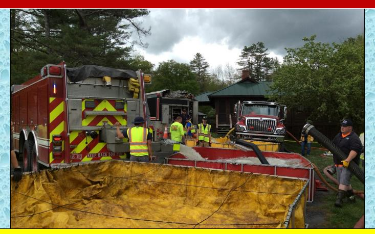
Around the 22-minute mark, operations transitioned to a dump tank operation. Orford Tanker 2 (1500 gpm/1500 gal) served as the dump site pumper.
