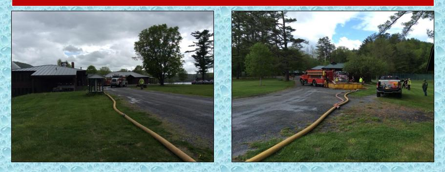
The dump site pumper supplied the attack pumper (Fairlee Engine 5) through a few hundred feet of 4-inch supply hose.
