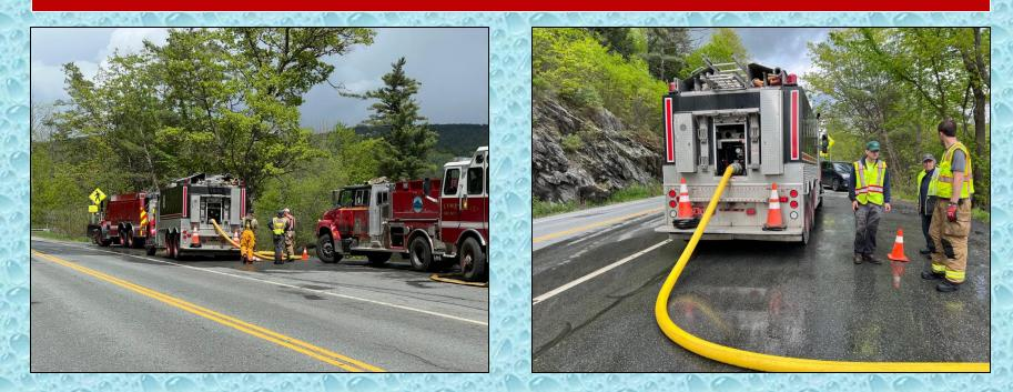
Tankers were loaded using 4-inch LDH and were loaded at the target rate of 1000 gpm.
