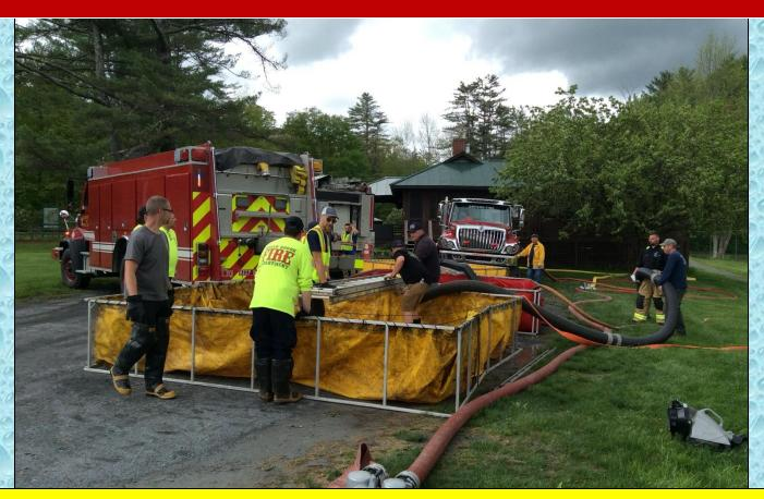
With the flow at 500 gpm, work gets underway around the 50-minute mark to move to a 3-dump tank operation.
