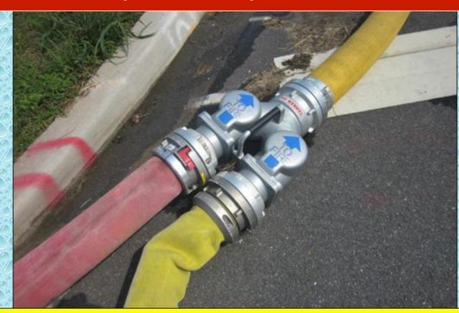
Once again, the use of a double-clappered siamese proved successful during the early minutes of a water supply drill involving tankers. The device allowed continuous flow to the attack piece while the dump tanks were set up.
