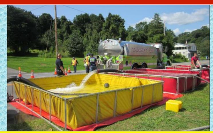
At the 17-minute mark, flow was moved to 500 gpm and the second dump tank was brought on-line. Tankers on the first, tanker task force began to arrive.
