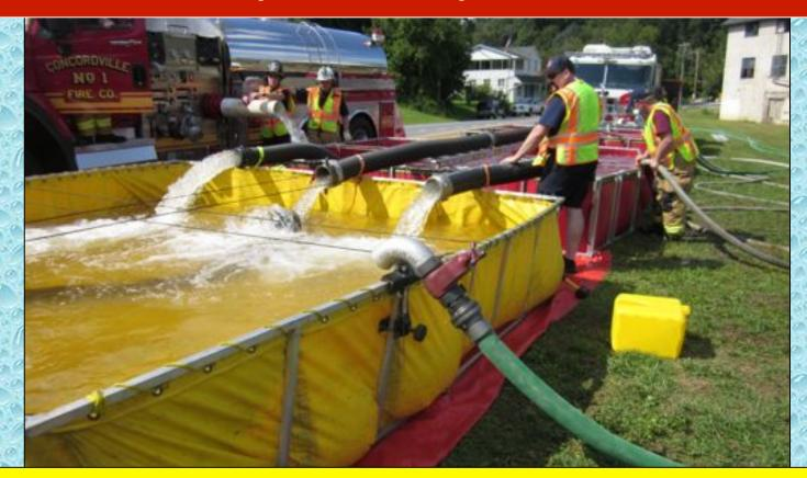
The operation peaked at 1100 gpm using three dump tanks. The single-lane arrangement seemed to work well and kept an entire lane of traffic open on the main road. The two supply lines seen in this photo are coming from the 7800-gallon tanker.
