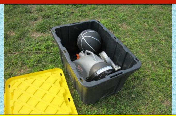
The Oxford tanker carried a nice "dump site" kit which included a TFT low level suction strainer, a standard jet siphon, a ball (for vortex control) and some tie-down straps.
