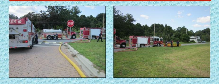
The first two arriving tankers operated in the nurse tanker mode as water flow operations commenced at 250 gpm at the quint. The quint was fed by a 5-inch supply line that was outfitted with a double-clappered siamese which allowed the tankers to pump off water until the dump tanks were ready.
