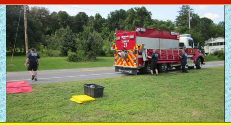
Oxford Tanker 21 (3,000-gallons) carries dual dump tanks. So their arrival on the scene proved very beneficial in helping to set up the site. The two-person crew hustled to deploy both dump tanks as well as provide additional support equipment – and of course, 3000 gallons of water.
