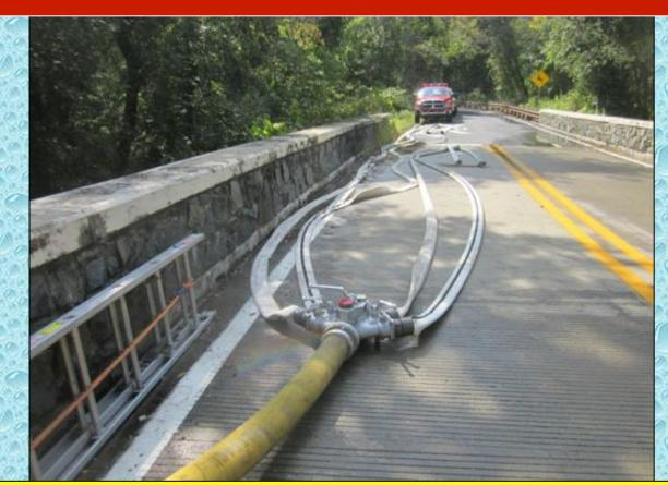
This loading station was supported by Longwood's Engine 25-1 – a 2,000 gpm pumper. The bridge was somewhat narrow, so fill site crews had to be careful not to block out units.
