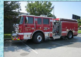
Longwood Tanker 25-3 – 1000 gpm pump w/7800 gal tank
