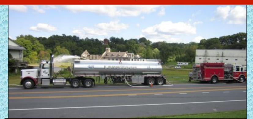
The use of the tractor trailer tanker simulated a real-life mutual aid response time for the area. With its 1,000 gpm pump, the rig is quite capable of supporting a large scale water supply operation once it gets there. In addition, rigs that could not dump water pumped off their water into this big tanker, which really was a 7800-gallon reservoir.
