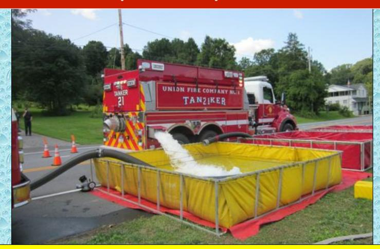
Tanker 21 dumps the first load of water and the operation is moved to a dump tank operation. Nurse tanker operations are stopped.
