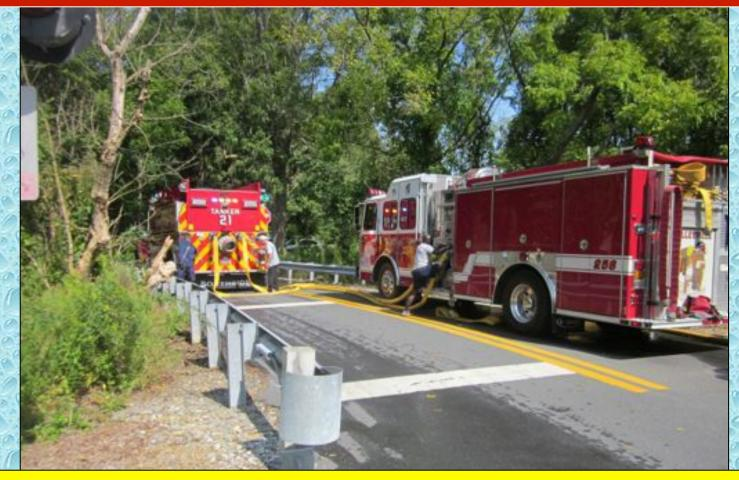
Talleyville Engine 25-6 (1,750 gpm) drafts off a bridge and loads Oxford Tanker 21 using dual, 3-inch fill lines.
