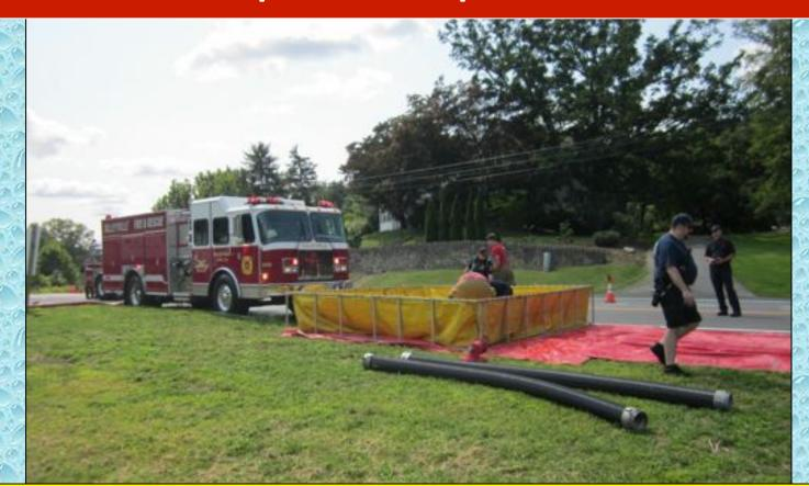
The plan was to try the "single-lane" arrangement of dump tanks so folks worked to place dump tanks in front of Engine 25-5.
