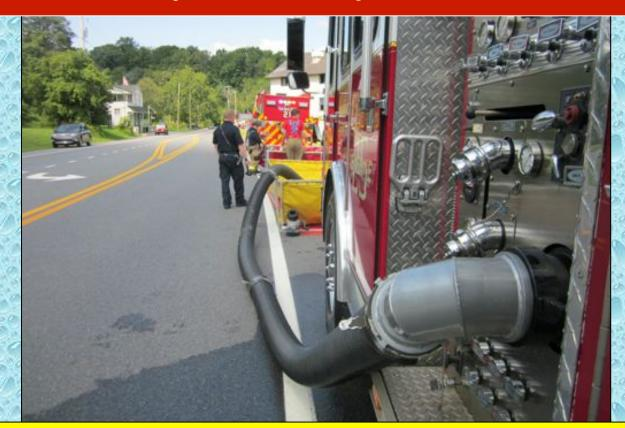
A suction elbow was used on Engine 25-5 in order to keep the suction hose closer to the rig and to gain distance. The elbow is a "best practice" when looking to use the single-lane concept. And of course, it allows for improved flow because a main suction inlet is used in lieu of a front suction inlet.
