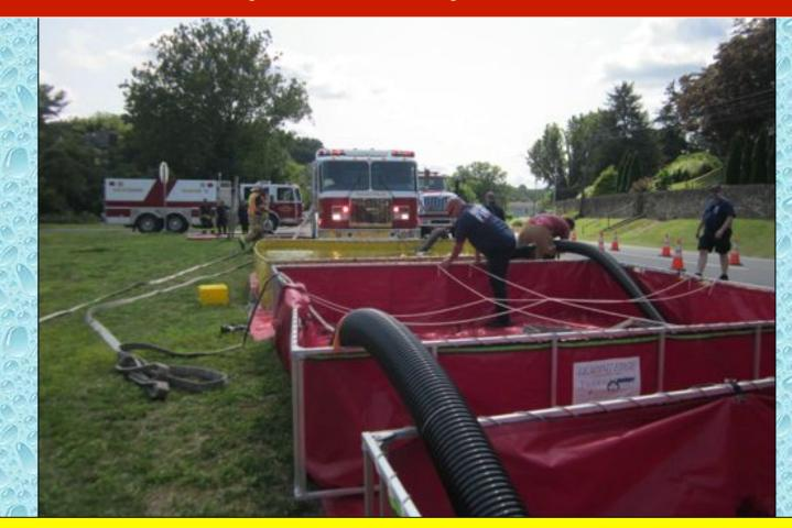
With the first dump tank in operation, work now begins to bring the second tank on line.
