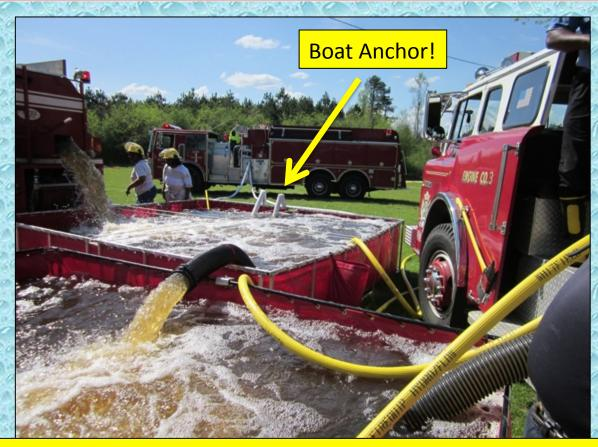
While not very "pretty," the heavy valve worked to hold down the discharge lines from the engine/tanker. Also – this kept the engine/tanker from blocking out tankers waiting to dump their water.
