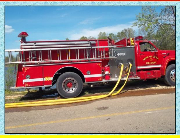
With no high-flow discharge, multiple hose lines were needed in order to support the 1,000 gpm fill rate goal.
