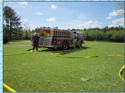
Water flow was started at the 7:50-minute mark after a little delay attaining a prime. A single, 100-ft, 2-1/2-inch hose line was used to support the 306 gpm flow at the portable monitor.
