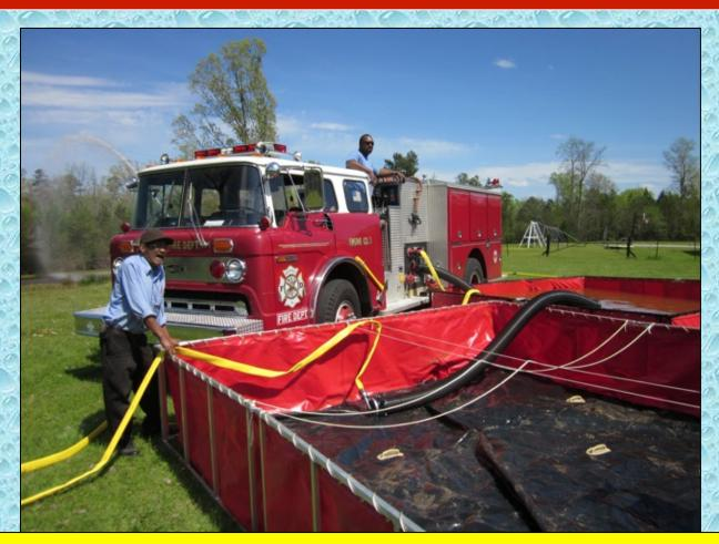
A jet siphon was set-up to transfer water from the second dump tank into the primary dump tank and now all that was needed was a load of water.
