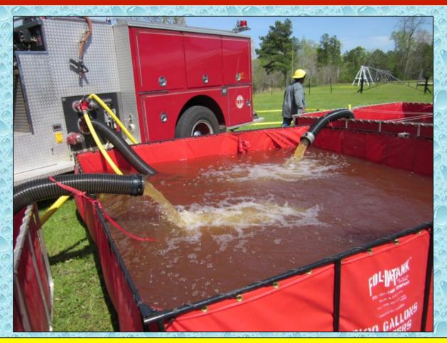
With three dump tanks in operation, water transfer capability became critical. The two jet siphons were able to keep up with the demand.
