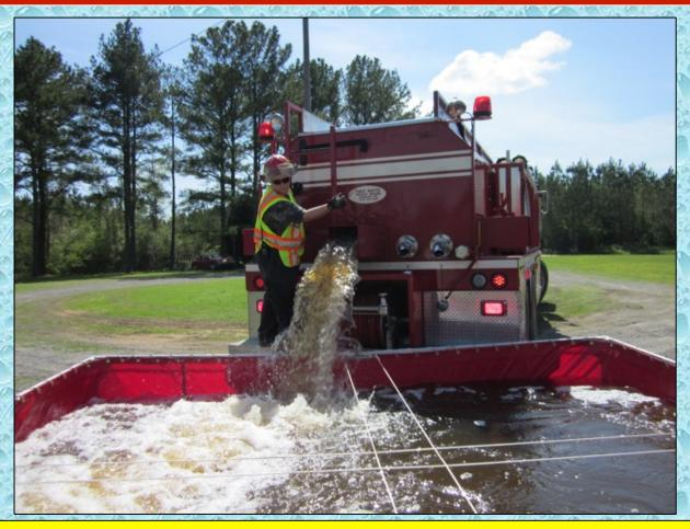
With the majority of the tankers being rear dumping units, the dump tanks were arranged to accommodate the rear dump capabilities.
