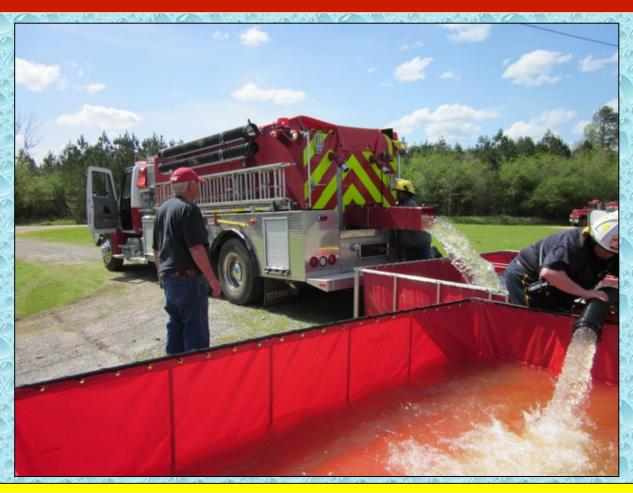
At the 15:38-minute mark, two dump tanks were in operation with a jet siphon in use for water transfer.
