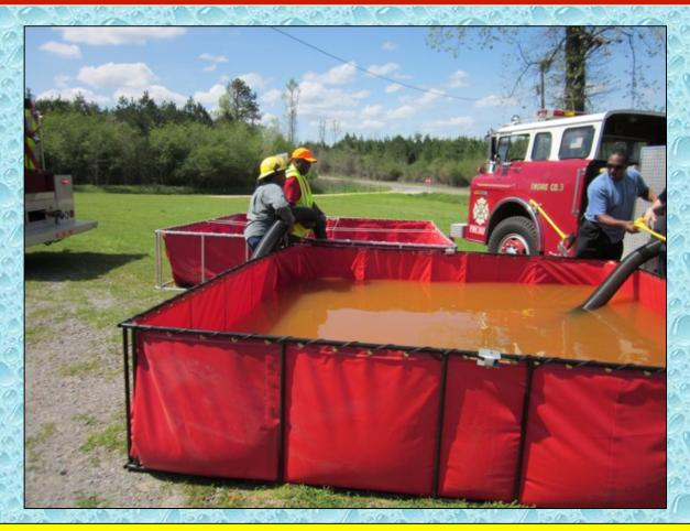
A second dump tank was deployed around the 12:03-minute mark and crews worked to set up a water transfer device.
