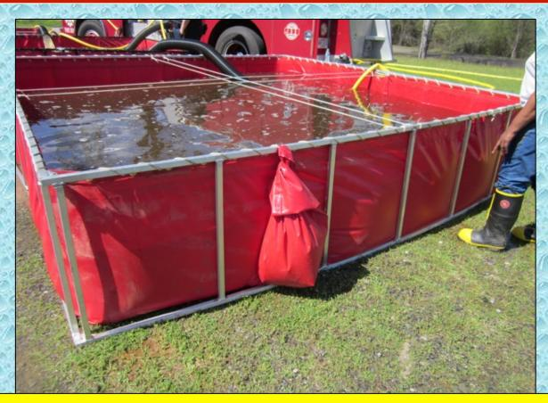
Dump tank drains can prove problematic if they are not secured properly. Any dump site is going to be a wet mess. A drain spilling its water is only going to make that worse.
