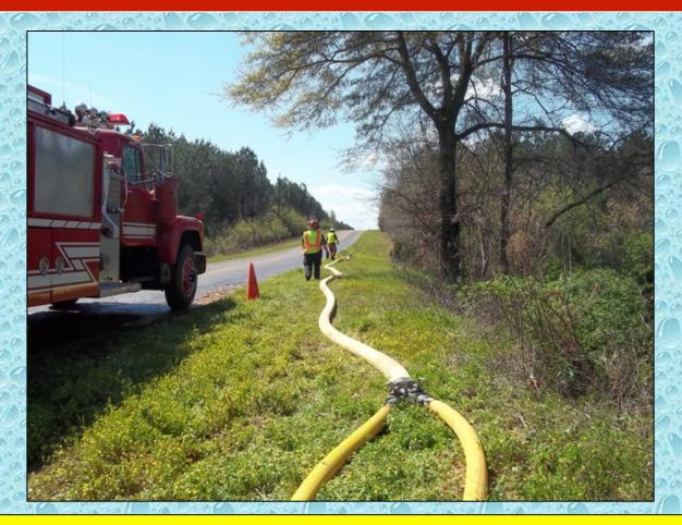
In order to set up a second fill station, 200 feet of 5-inch LDH was used. This setup greatly improved tanker fill times.
