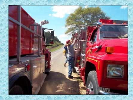
With Engine 51 only carrying 20-feet of suction hose, the suction hose on the tanker became very important.
