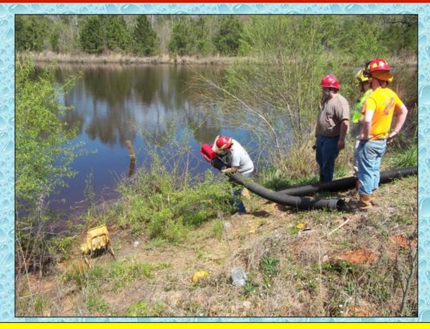
Forty feet of suction hose and a floating strainer were used to establish the draft.
