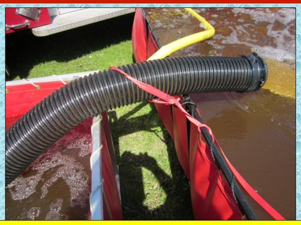
A tie-down strap was used to secure this 5-inch suction hose being used with a jet siphon. An important point is not to have the discharge end submersed – otherwise water can siphon back when the jet is turned off.
