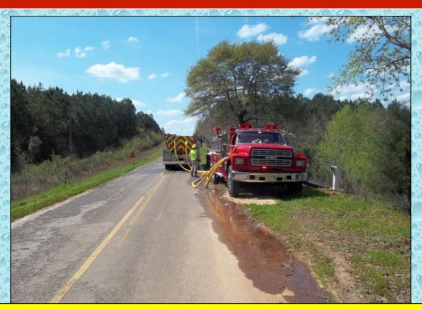
A tanker fill site needs to operate like a NASCAR pit stop. Time cannot be made up on the road, so anything that can be done to reduce fill times will enhance the overall shuttle operation.
