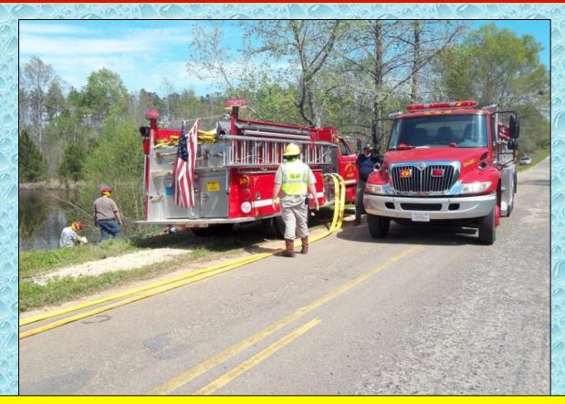
Two, 2-1/2-inch lines were stretched as fill lines. While not as efficient as LDH, by keeping the two lines under 100-ft, the pumper was able to fill tankers at around 1,000 gpm.
