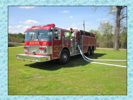
One "bump in the road" was this 2,500-gallon engine/tanker that had no dump capability. Nobody had any type of fitting that would connect to a dump tank to hold a discharge hose, so the crew rigged up a couple of 2-1/2" lines to a heavy valve. The valve became somewhat of a boat anchor in the middle of the dump tank and the engine/tanker was able to pump off its water and contribute to the success of the shuttle operation.
