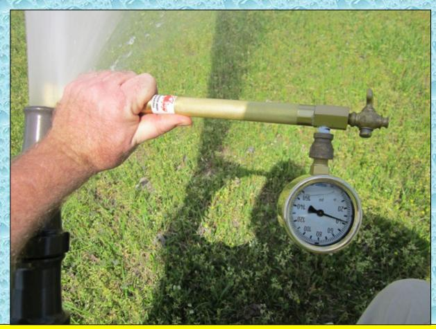
A hand-held pitot was used to verify the flow from the portable monitor. At the 21:30-minute mark, the flow was moved to 346 gpm.
