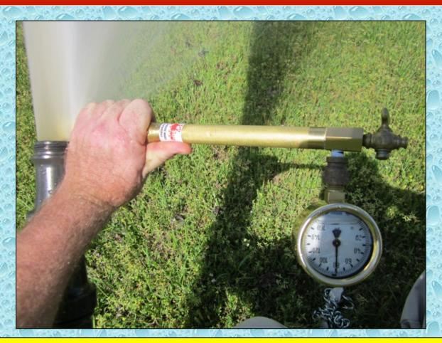
At the 67:00-minute mark, flow was increased one last time to 813 gpm where it was sustained through the remainder of the drill.
