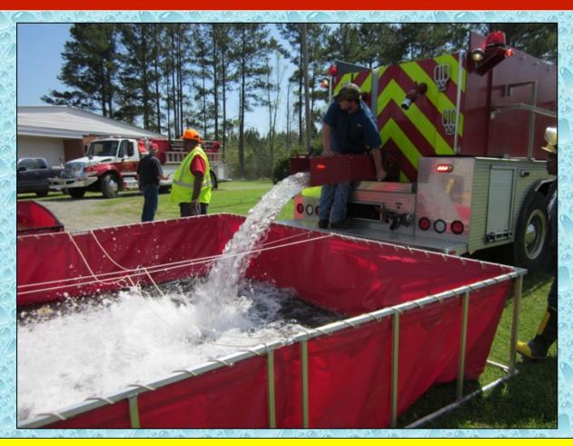
With the arrival of the next tanker, water could now be offloaded into the second dump tank.
