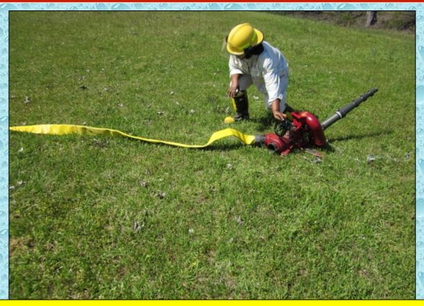
A portable monitor was deployed in order to flow water throughout the drill. The monitor was outfitted with a set of "stacked tips," with an 1-3/8-inch being the first tip size used.
