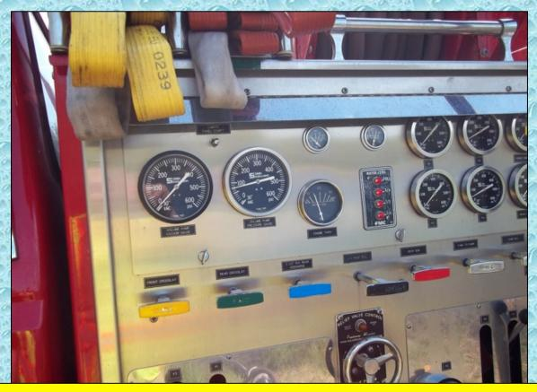
One of the challenges of filling tankers is managing the discharge pressure of the pump. When filling a large empty container like a tanker, pressure might be hard to develop until the tank is almost full. Then pressure develops all of a sudden!
