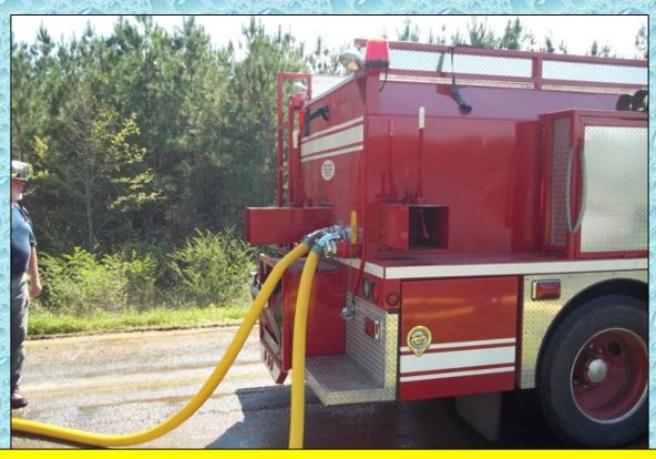
This tanker was equipped with two, "Fireman's Friend" valves which save time in terms of having to open and close a valve. However, too much time was still used threading and unthreading the hose lines. A couple of Storz or CamLok fittings would have proven very helpful in reducing the "pit stop" times!
