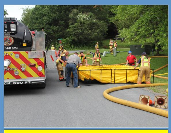
A folding tank was placed for use by a vacuum tanker and fed by a separate pump
