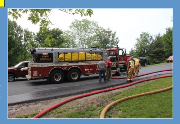
This site used portable pumps to feed a pumper.
