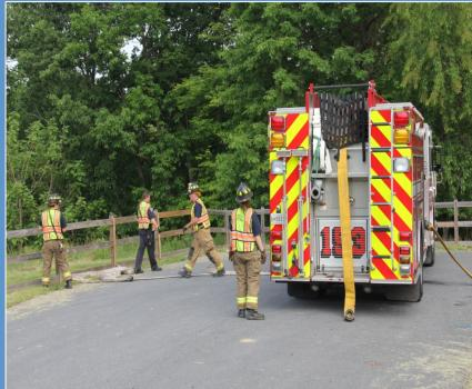
Relay pumper was placed between the fire ground and dump site
