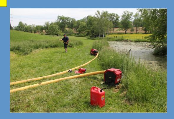
Shown is the pumper that was relaying the water from the portable pumps
