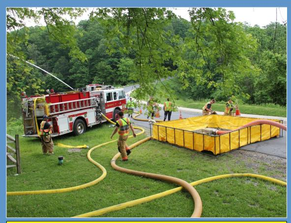
Fill site #2 Folding tank for vacuum tanker.
