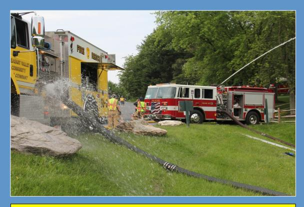
This fill site was on a roadway that ran past a lake. A fill for standard tankers was made on one end and a second fill for a vacuum tanker consisting of a folding tank and sleeve with strainer, on the other end.
