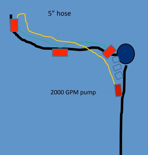
Larger capacity pumps are required to push water at long distances and higher elevations.
