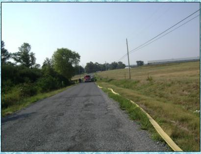
500-feet of 5-inch is laid out simulating the attack engine positioning up a farm lane or similar type of road.
