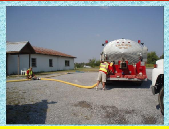
4-inch hose was used as the fill line. Here, the loader is shown manning the control valve while the other crew member manages making and breaking the connection to the tanker.
