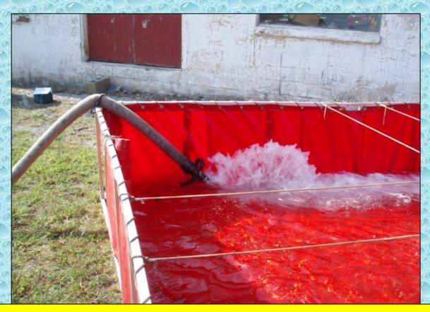
While the 3-inch hose with 2-1/2-inch nozzle worked, it could have been improved by using a larger hose line or better control valve. However, the concept implemented was okay.
