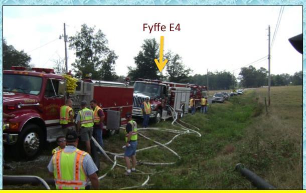
As the dump site grew, it became more difficult for the supply engine to support the attack engine AND run the four jet siphons. So the decision was made to use Fyffe Engine 4 to run jet siphons. The problem was getting water supply to the Fyffe engine – a separate dump tank could have been used but there was really nowhere to locate it. Thus – this option didn't work out so well.
