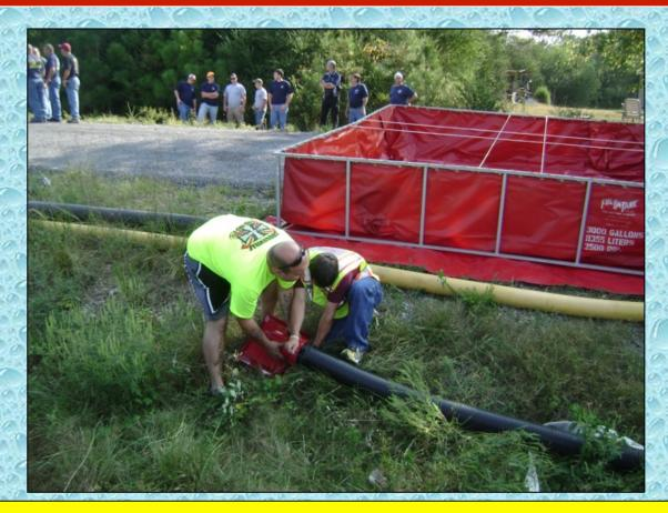
The crew works to connect a low level strainer to the suction hose so that maximum water can be reached while drafting.
