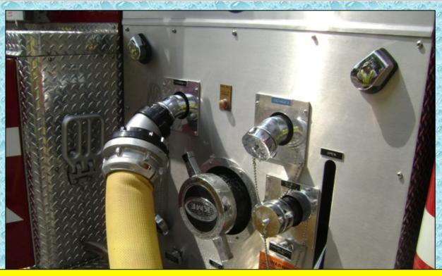
One issue not identified until late into the operation was the lack of a high-flow discharge on the supply engine. Just because a 5-inch hose line can be connected to a 2-1/2-inch discharge does NOT mean that 5-inch flows can be expected. In this drill, the 745 gpm flow was maximizing the single discharge. A better solution would have been to pump two, 3" lines into a 5" LDH manifold.
