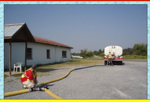
One person served as the "loader" and controlled the water flow into the tankers. Other crew members made and broke connections as needed. With almost all of the tankers arriving with a 4" Storz fill fitting, there was little need for adaptors - a grand improvement over the first year!
