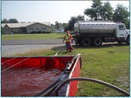
One problem that occurred was that the suction hose from the hydrant feed kept trying to float to the surface and spray water into the other suction hose's strainer area thus causing the possibility of cavitation.
