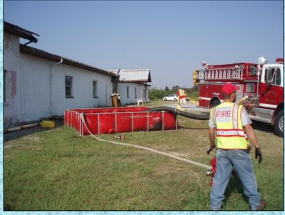
After a little while, the nozzle was changed out for a piece of suction hose equipped with an adaptor. This arrangement allowed for less restriction and better flow.
