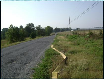
With the timer now running, crews work quickly to get a hose line in place to support a 250 gpm flow at the 5-minute mark. Meanwhile, Adamsburg's tanker gets into position to begin nurse tanker operations.
