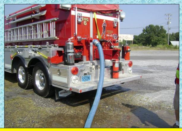
4-inch hose was used to fill each tanker that arrived at the lake fill site – this made a significant impact on reducing fill times.
