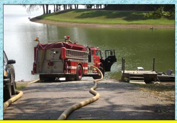
In order to maximize pump ability at the lake fill site, Dogtown's Engine 1 (1,250 gpm) was positioned on the boat ramp. Dual, 4-inch hoses lines were stretched back up the ramp to the parking lot where a tanker fill station was constructed.
