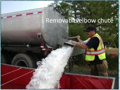
Rear off-loading tanks can prove troublesome sometimes when dealing with a multiple-dump tank arrangement on a limited space road. However, at this drill, a couple of quick-thinking dump site crew members improvised operations by using a dump chute from another tanker to convert the dump chute of a rear off-loading tanker – and it worked out just great.
