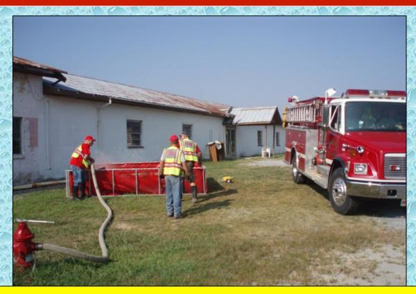
The theory behind this operation is that the dump tank gets filled using a control valve to control overflow and the pumper drafts from the tank. Some folks call this an "open" relay. The 1,250 gpm pumper can fill tankers at a rate much higher than what the hydrant could supply in a direct connection arrangement.
