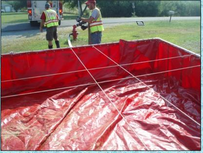
A 3,000 gallon dump tank was used and positioned near the hydrant. A hose line was stretched from the hydrant to the dump tank and outfitted with a 2-1/2-inch nozzle.
