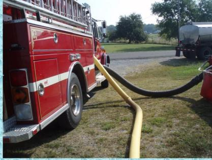
Pumper 1 then supplied a length of 5-inch hose which was wyed into two, 4-inch fill lines.
