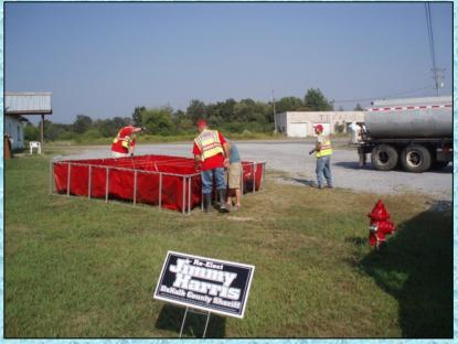
Since hooking the pumper up directly to the hydrant would have produced a less than desirable fill rate, the decision was made to fill a dump tank using the hydrant - and then draft from the dump tank and fill tankers at a higher flow rate.
