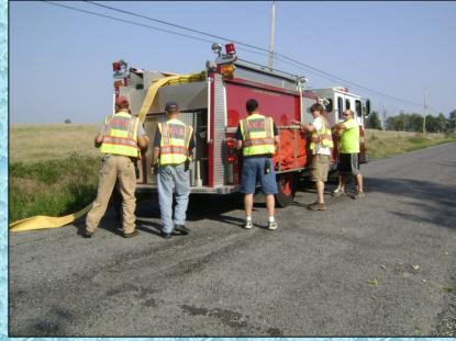
Engine 2's crew is shown above dropping off some equipment for the dump site and laying out a 5-inch supply line.
