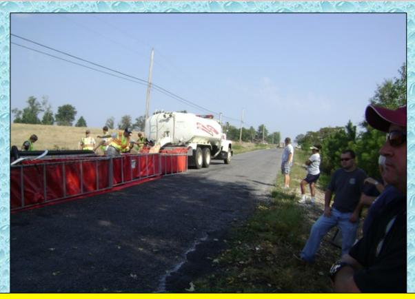
Around the 39:00 minute mark, three dump tanks were operational and rear off-loading tankers were directed to offload into the last tank thus keeping the roadway clear.
