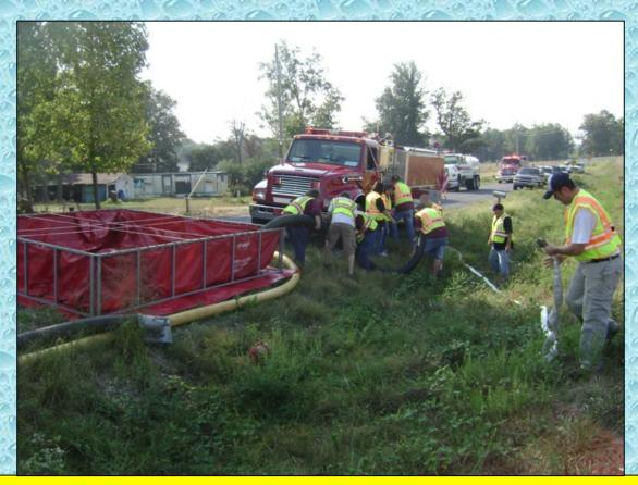
Because of the narrow road, the Henagar engine sets up to draft using 20-ft of suction hose connected to its driver side suction inlet. This frees up road space and still allows maximum intake capability.
