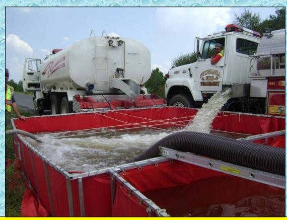
With five dump tanks now in operation, multiple tankers can dump at once. Around the 75-minute mark, the flow was moved to 745 gpm where it was sustained for about 15-minutes before being reduced back to 690 gpm.
