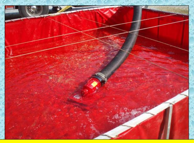
Pumper 1 used a low level strainer to ensure that as much water in the tank that could be reached was reached.
