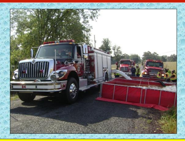
More tankers arrive as additional units are dispatched to assist on the call. Fyffe Engine 4 is shown above off-loading its water as flow is now at 500 gpm.
