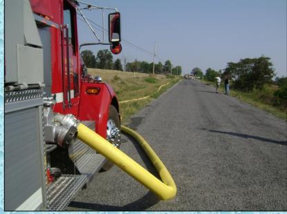
Adamsburg Tanker 1 supplies the 5-inch line using its LDH discharge – which is a good example of why a tanker equipped with a full-size pump and an LDH discharge is a valuable asset in rural water supply operations.
