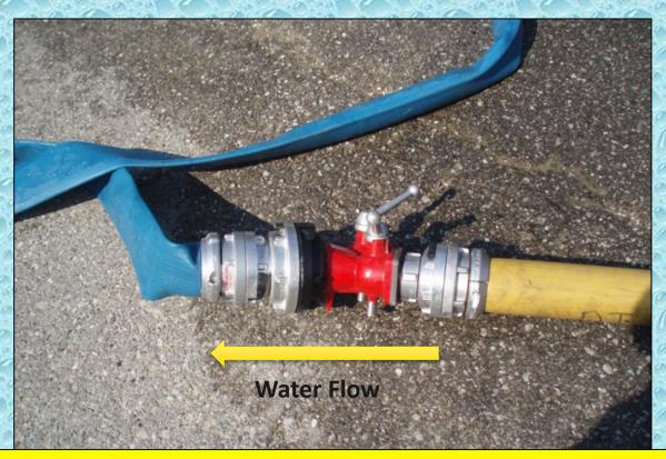
A 5"x 2-1/2"x2-1/2" wye was used as the in-line control valve for loading tankers. The valve was reversed so that one of the 2-1/2" outlets could function as a drain which made breaking the tanker connection much easier.
