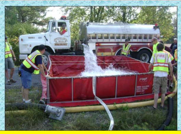
With the first tank in place, Sylvania's tanker offloads it water so that Henagar's engine can begin drafting operations. Meanwhile, nurse tanker operations continue.
