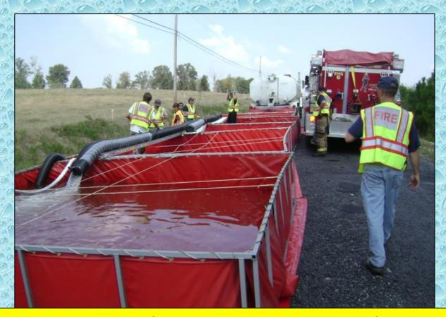
Near the 60-minute mark, four tanks are operating and the flow is pushed to 630 gpm. The challenge at the dump site became the ability to transfer water fast enough to accommodate the flow demand.
