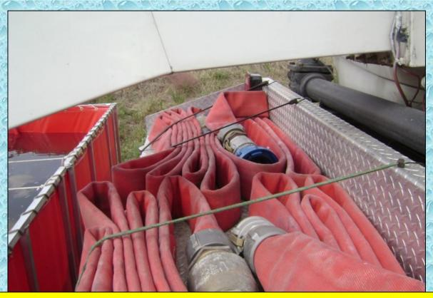
One thing learned from previous drills was the need for standardized adaptors at tanker fill sites. The photo above shows pre-rigged fill lines on Sylvania Tanker 2 that are set-up to quickly connect to the direct fills – the blue 4-inch Storz fitting is the agreed upon fitting for DeKalb County tanker fill operations.
