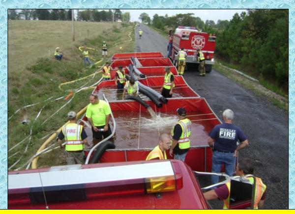
In the end, five dump tanks were used to support the operation and the operation topped out at 745 gpm for about 15 minutes. However, 690 gpm appears to be the flow sustainable by this operation.
