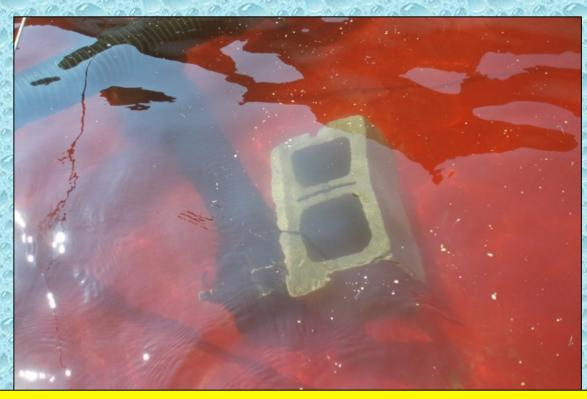
To remedy the floating problem, an "Alabama boat anchor" was used to help secure the suction hose to the bottom of the dump tank. Once in place, the concrete block did its job and floatation was never an issue again during the drill.
