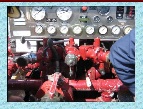
A single, 2-1/2-inch discharge cannot flow the rated capacity of the pump even when pumping into a 5-inch LDH line.
