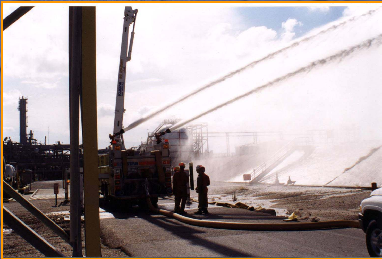
Figure 10. Equistar's Foam Tower 1 flowing through both deck guns for tests.
