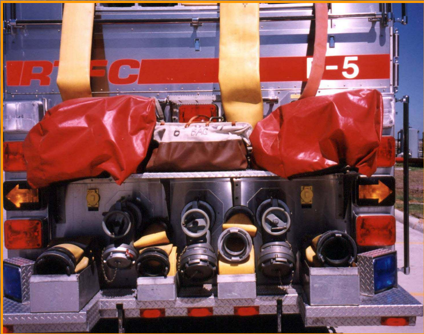
Figure 3. The three 6" pump intake with the original piston-intake valves. The red covers cover preconnected 1250-gpm TFT Crossfire portable monitors.
