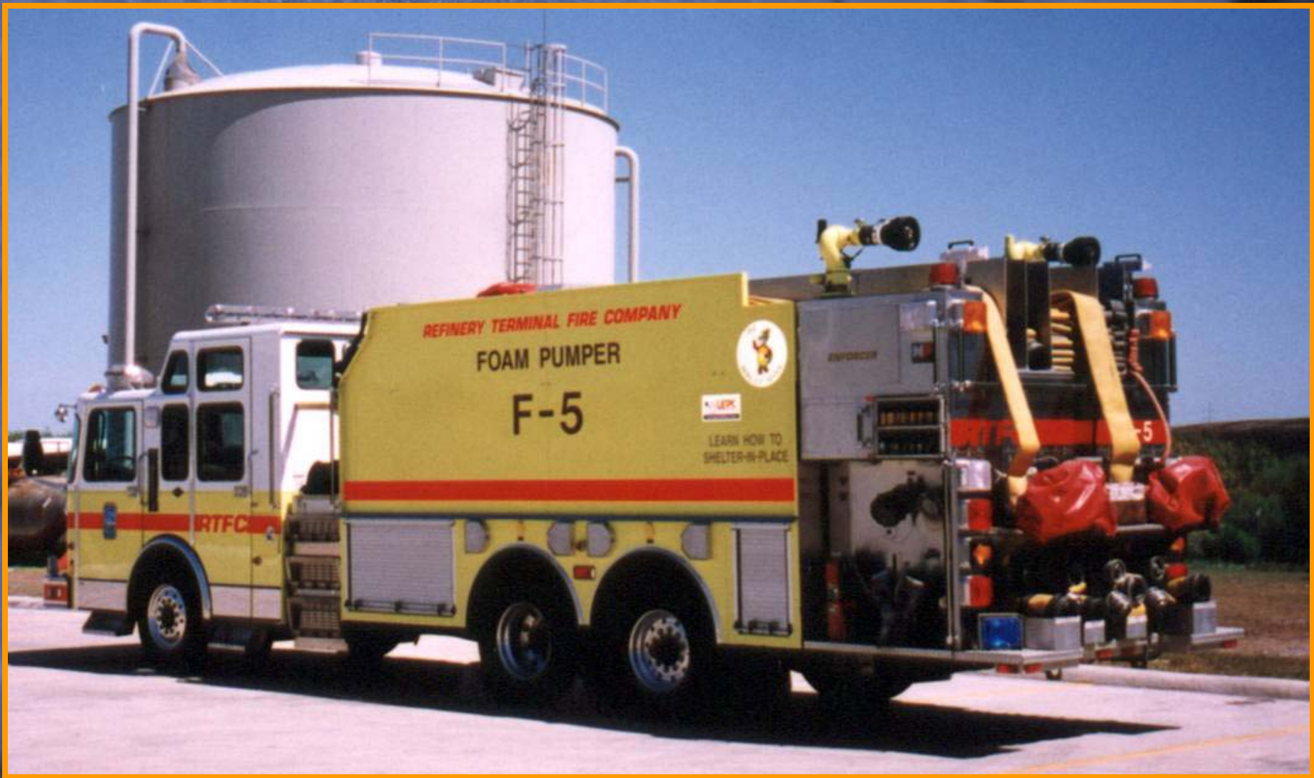
Figure 2. RTFC's Foam-5, a 3000-gpm pumper with rear-mounted pump and top-mount control panel.
