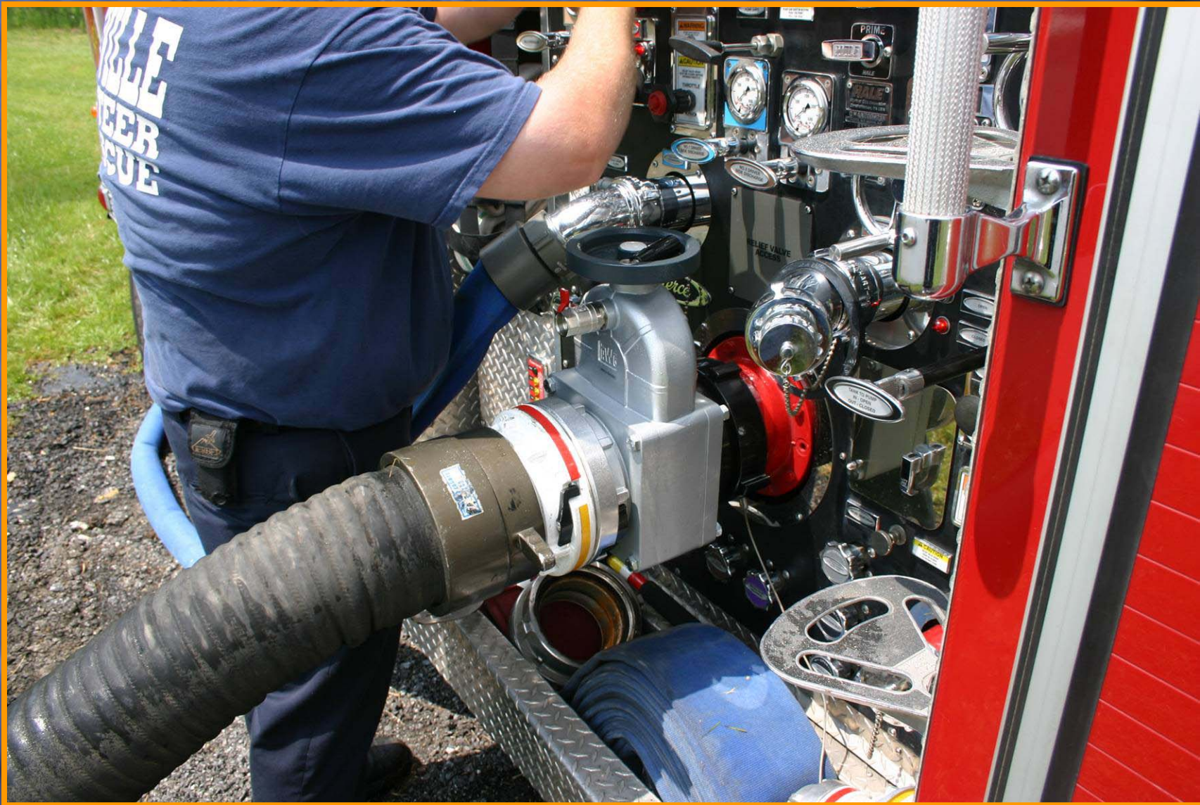
Figure 16. The test of the Kochek 5-1/4" Gate Intake Valve produced a flow of 2062 gpm, and a pump discharge pressure of 200 psi at a speed of 1635 rpm.
