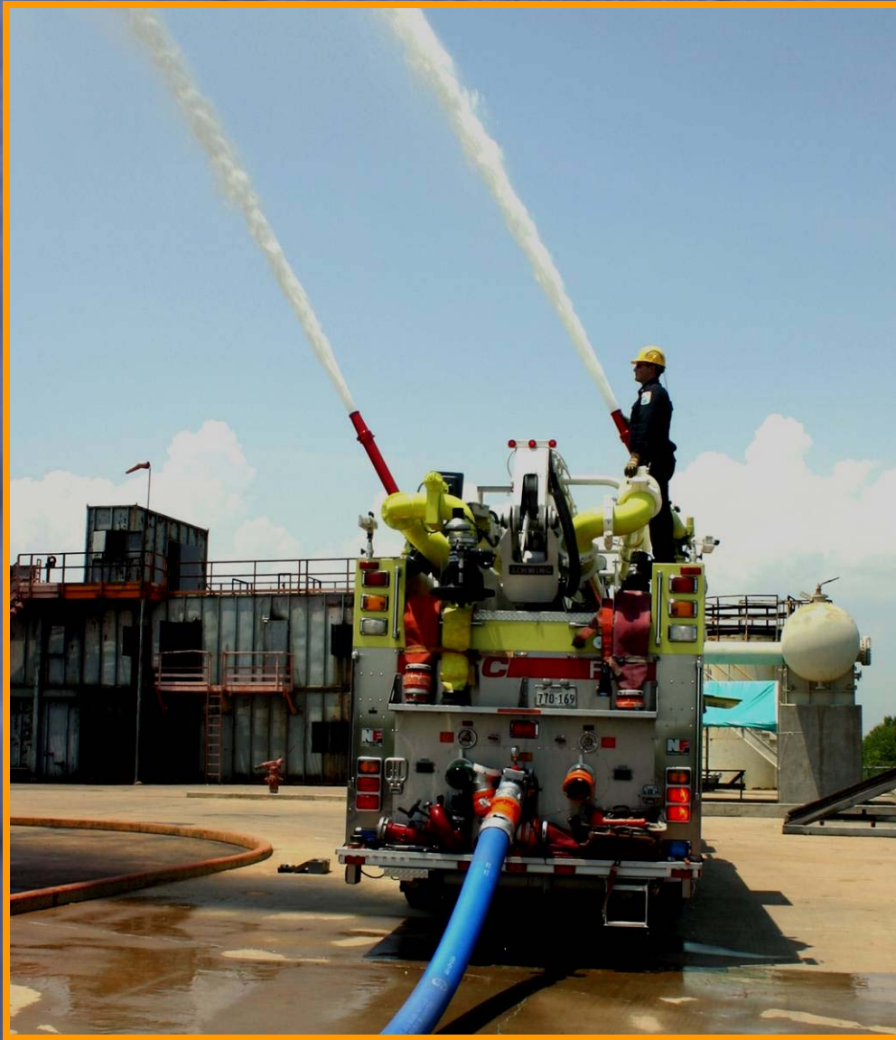
Figure 13. The deck guns on FT-2 were equipped with 3" smoothbore nozzles to measure flow. The supply line is 7-1/4" Williams hose.
