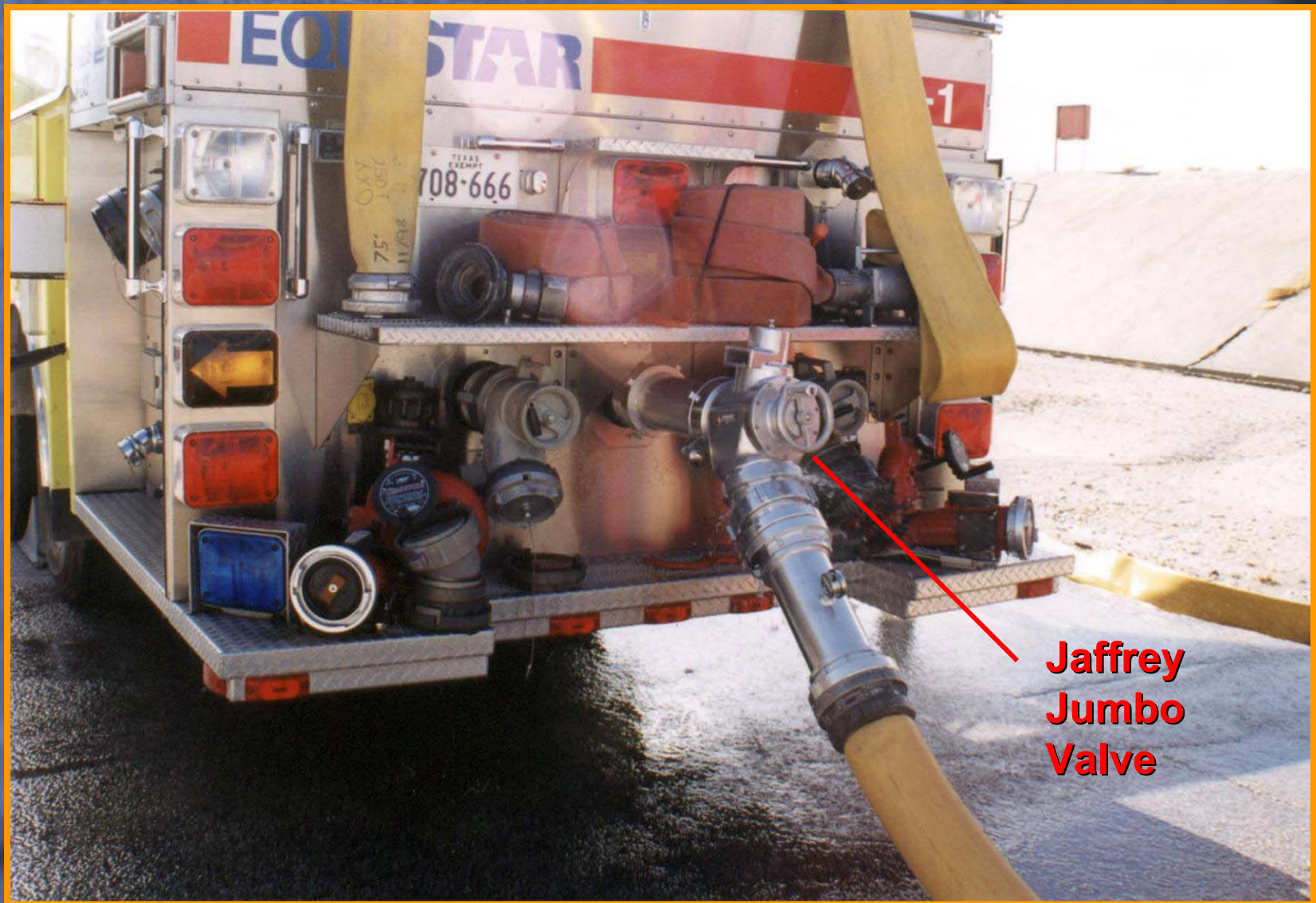
Figure 12. Test 2 used the Jaffrey jumbo piston intake valve. The test results were 35 psi friction loss at a flow of 4000 gpm. This resulted in a friction loss just slightly higher than Test 1 when no valve was installed.
