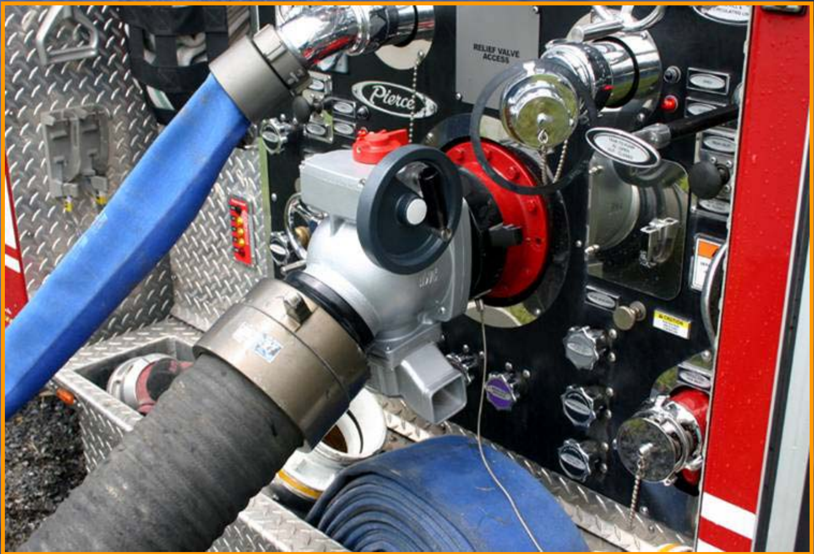
Figure 15. The test of the Kochek ball intake valve produced a flow of 1491 gpm and a pump discharge pressure of 130 psi, at 1500 rpm (the maximum speed attainable).
