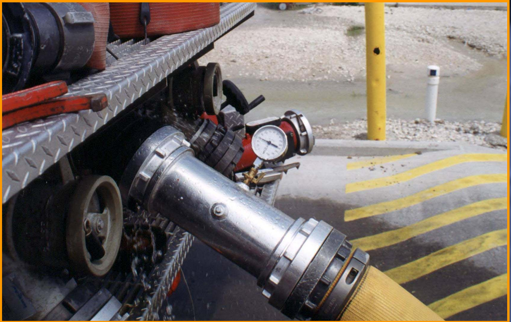
Figure 11. Test 1 was done with no valve installed. The friction loss was measured between the in-line shown and a master intake test gauge at the pump. In this test the friction loss was 35 psi at a flow of 4142 gpm.
