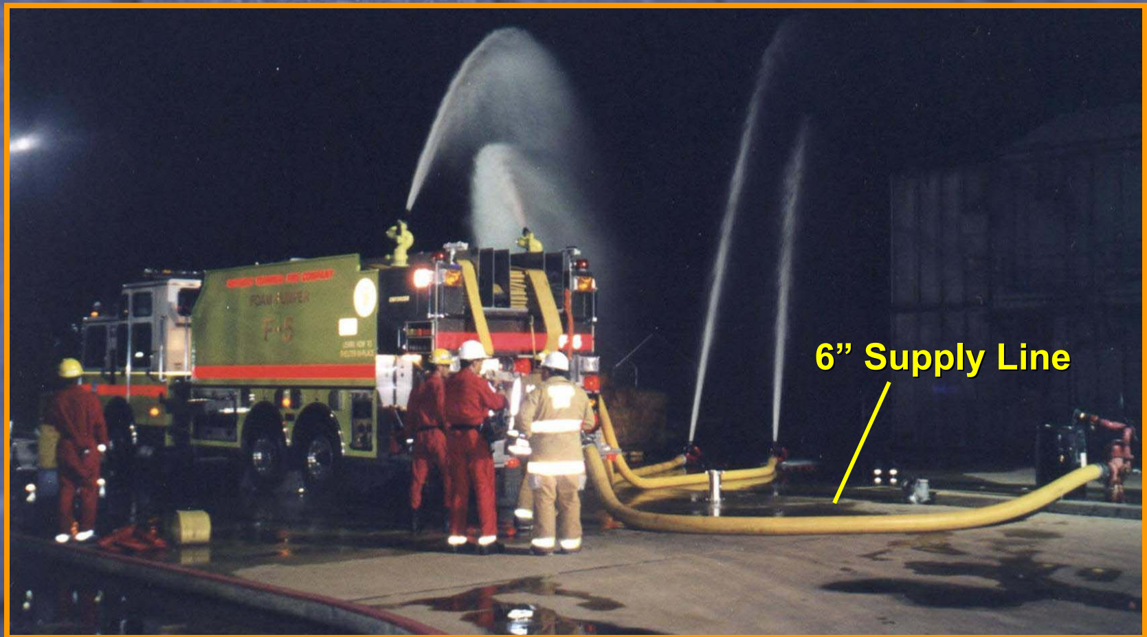
Figure 5. In the RTFC intake valve tests, two deck guns and 2 portable monitors with smoothbore nozzles were used so pressures could be measured with a pitot tube.
