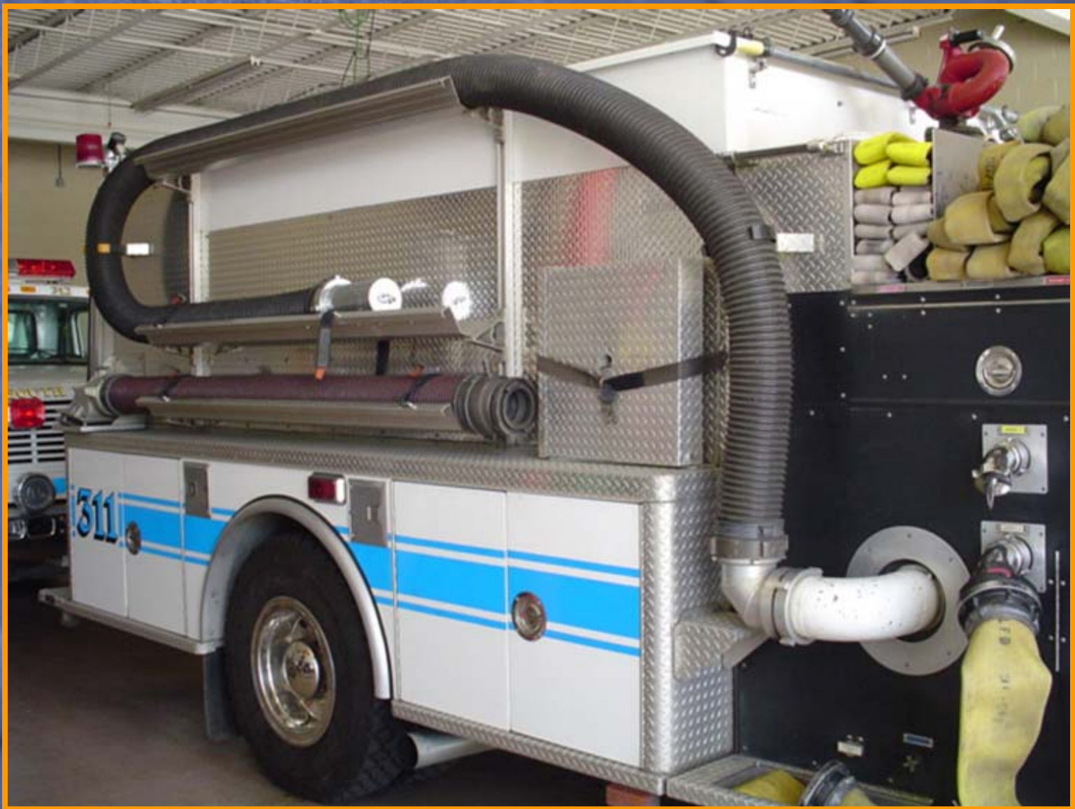
Figure 18. The department is a firm believer in squirrel tail suctions to make drafting set up easy.
