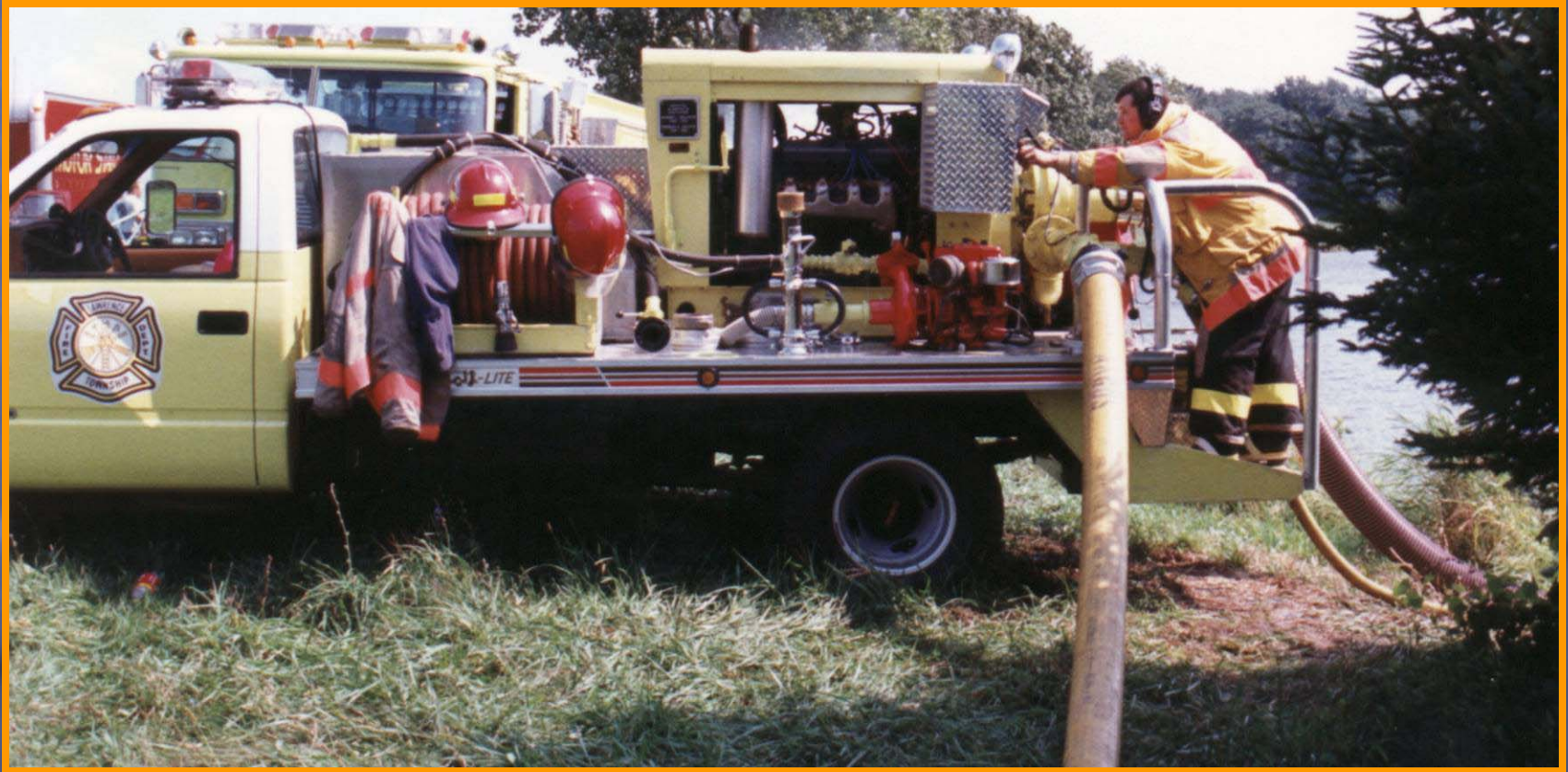
Figure 11. Once in position, the operator starts the engine and operates the pump from the rear.
