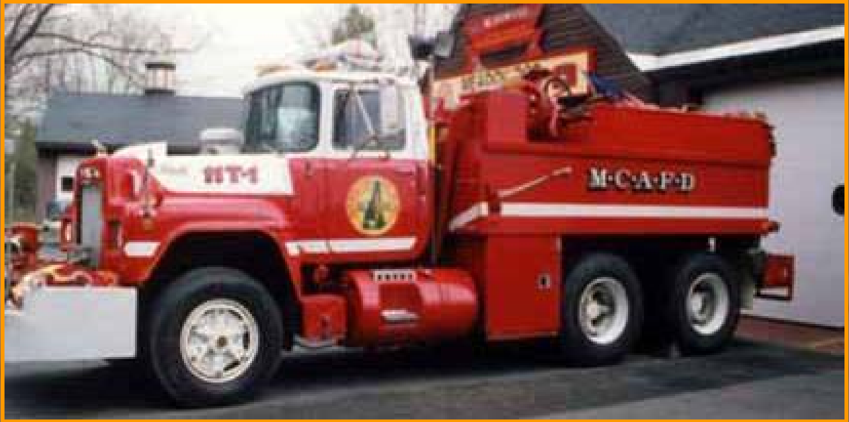
Figure 21. The attack unit is equipped with a large water tank and a 750-gpm front-mount pump
