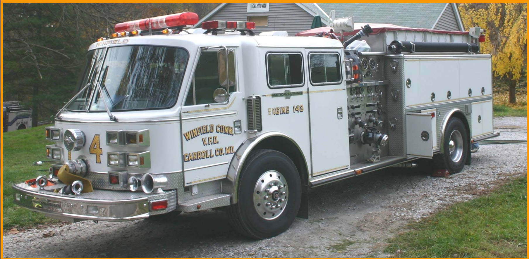
Figure 1. Winfield's 1500-gpm E-143 has been set up for rural firefighting and to simplify operation and getting big lines into service quick.
