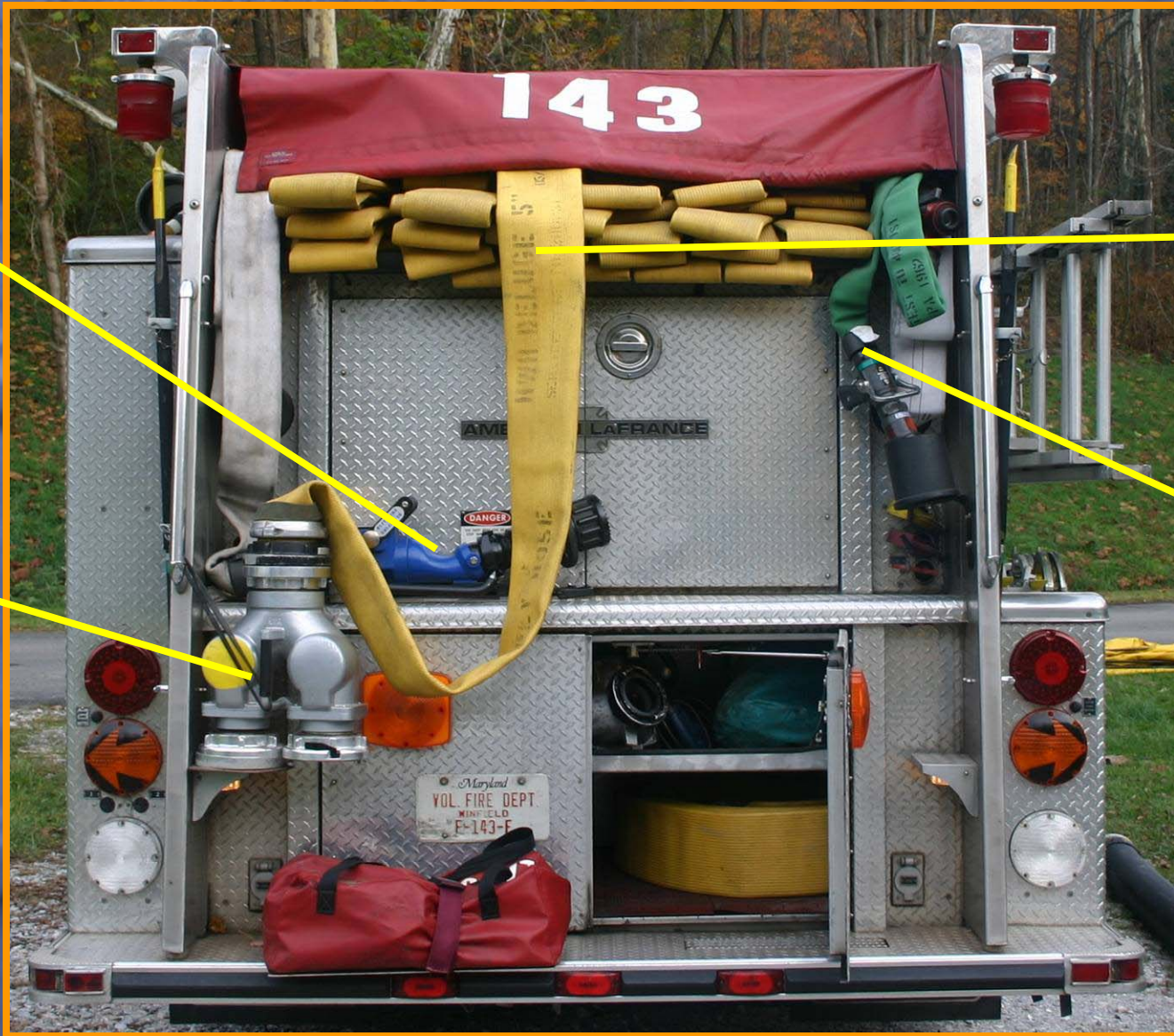
Figure 3. A busy back end! On the left is the 5" clappered siamese for the "rural hitch" for laying up long driveways, a bed of 5" hose, a preconnected 2-1/2" line, and a preconnected Blitzfire.
