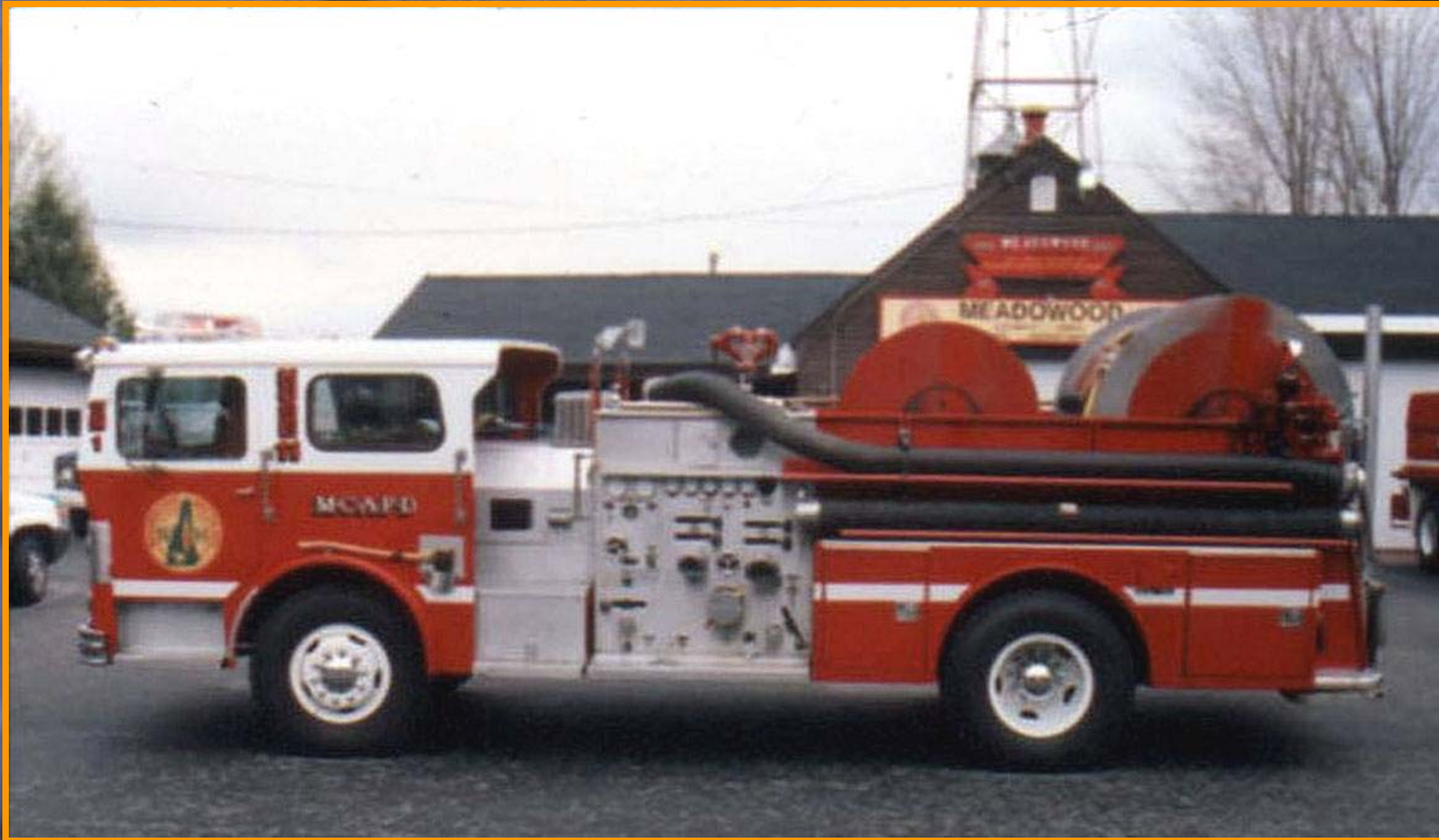
Figures 25. The Meadowood firefighters took a used 1000-gpm pumper and equipped it with two reels of 4" hose, extra suction hose, and all of the equipment used for drafting and relay pumping operations to supply water to attack apparatus.
