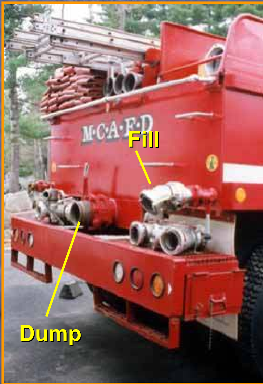
Figure 24. The rear shows the 4" hose bed, LDH fittings, and tank dump valve and direct tank fill for use when the unit is required to shuttle water.
