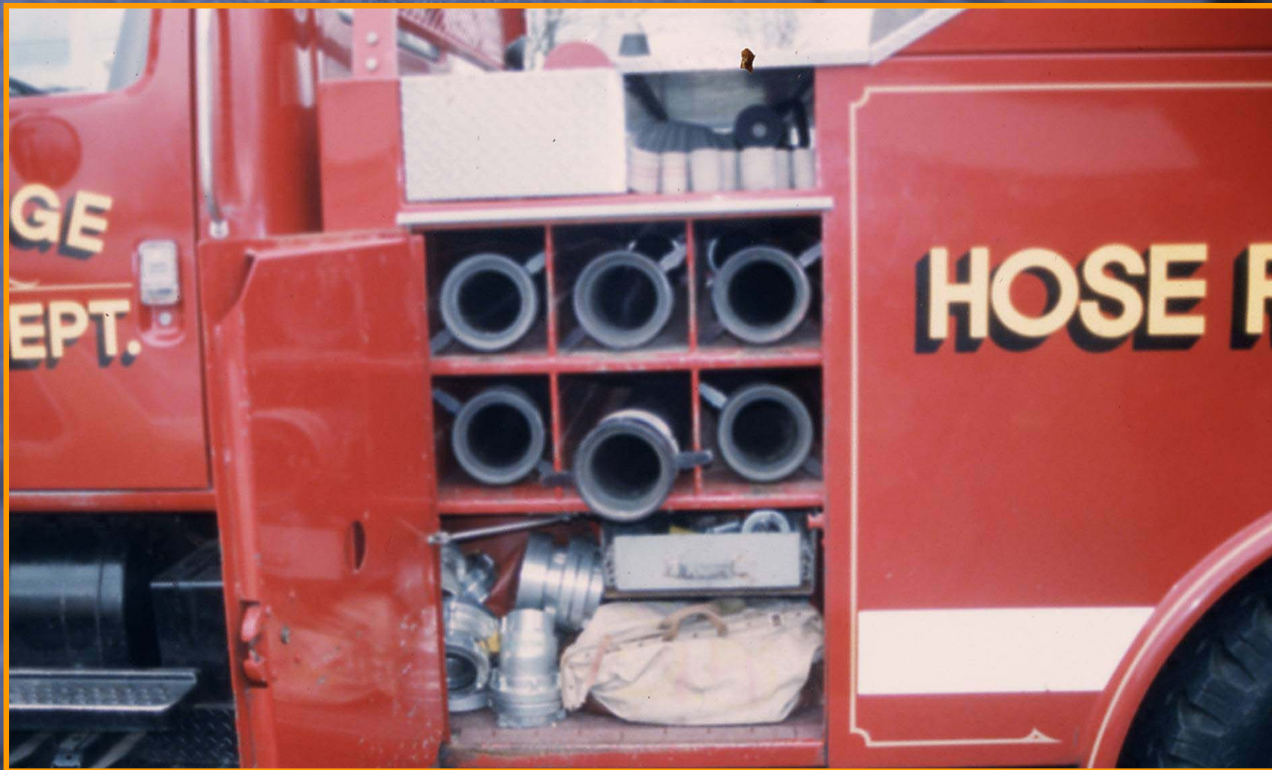
Figure 10. Six short lengths of suction hose are utilized so they can be carried in a compartment (accessible from both sides) that keeps the hose low for easy accessibility.
