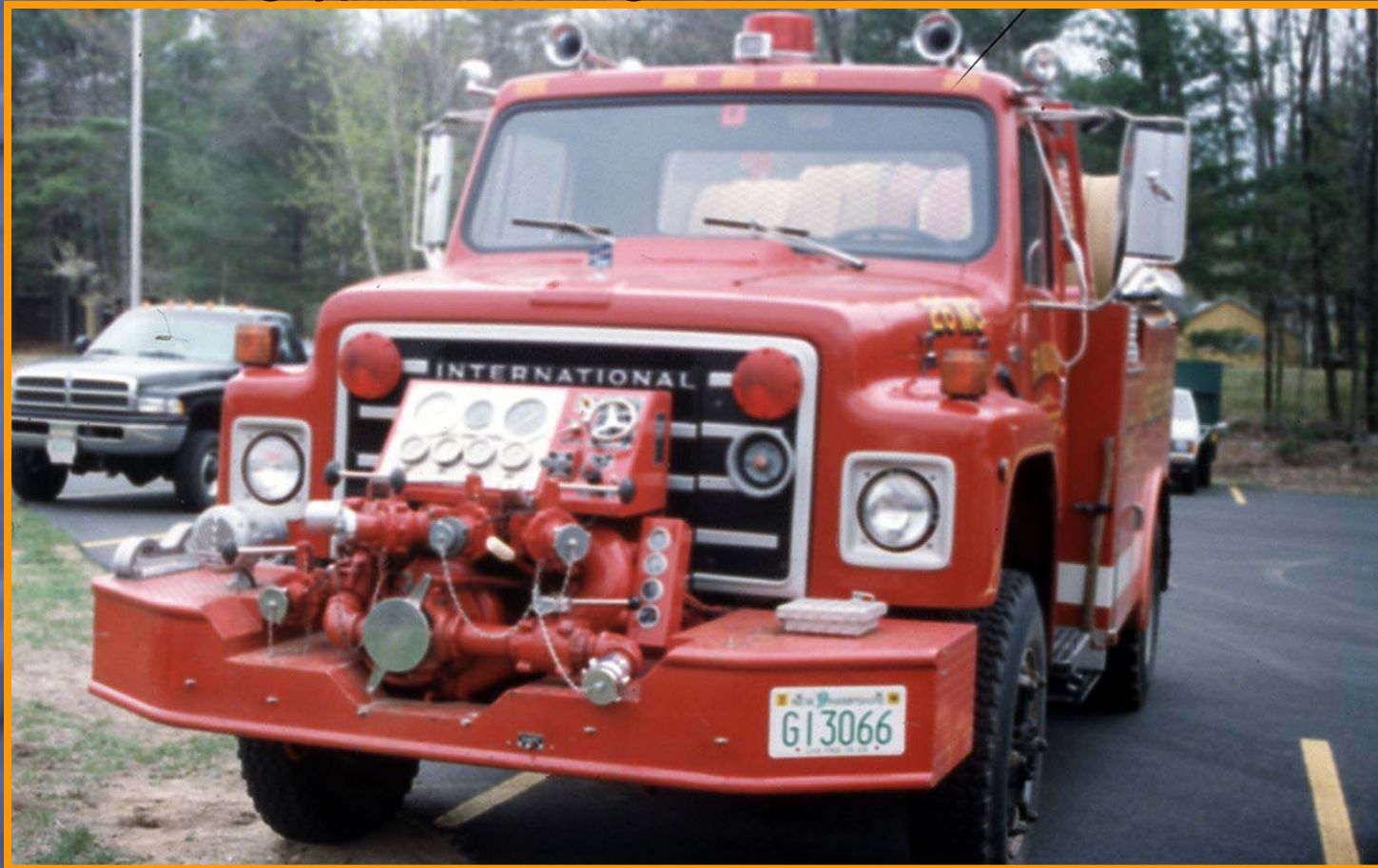
Figure 8. The unit is equipped with a 750-gpm front-mount pump to simplify drafting operations.
