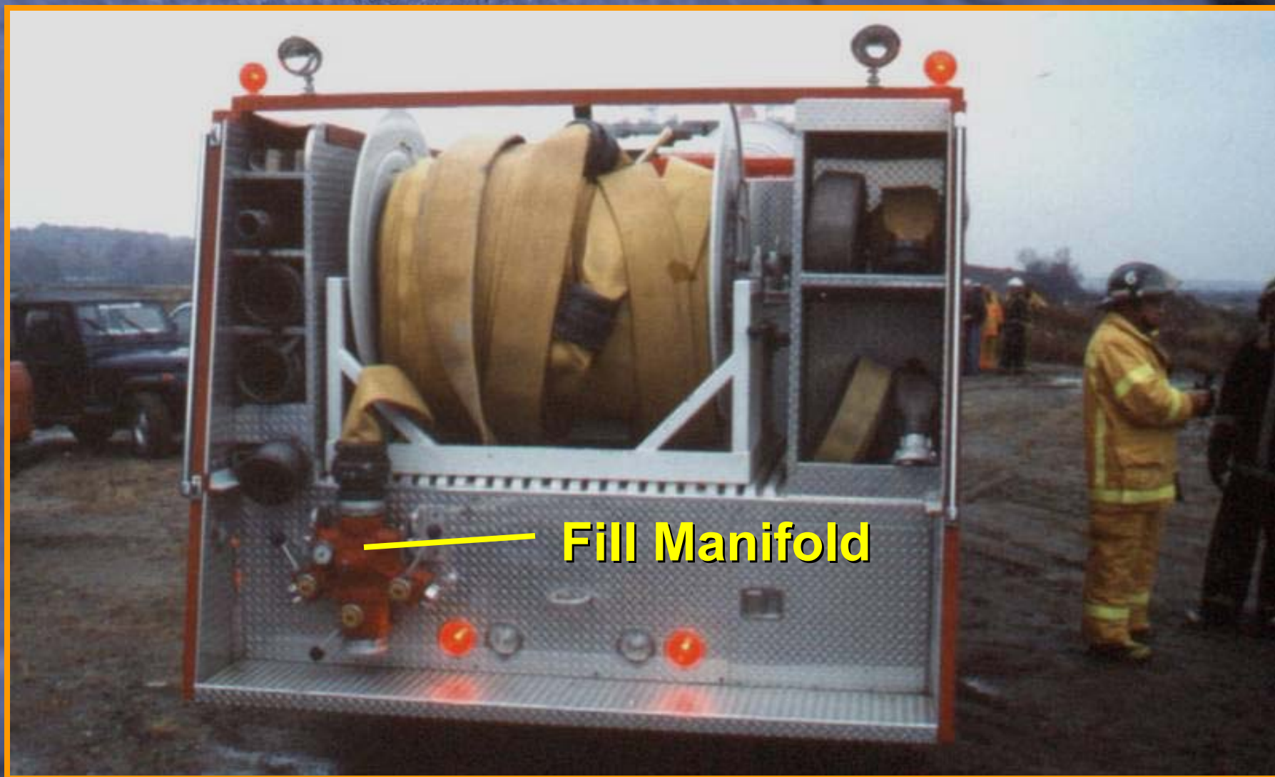
Figure 5. The fill manifold at the rear is preconnected to 600 feet of 5" hose carried on the reel. Suction hose is carried in the left compartment.
