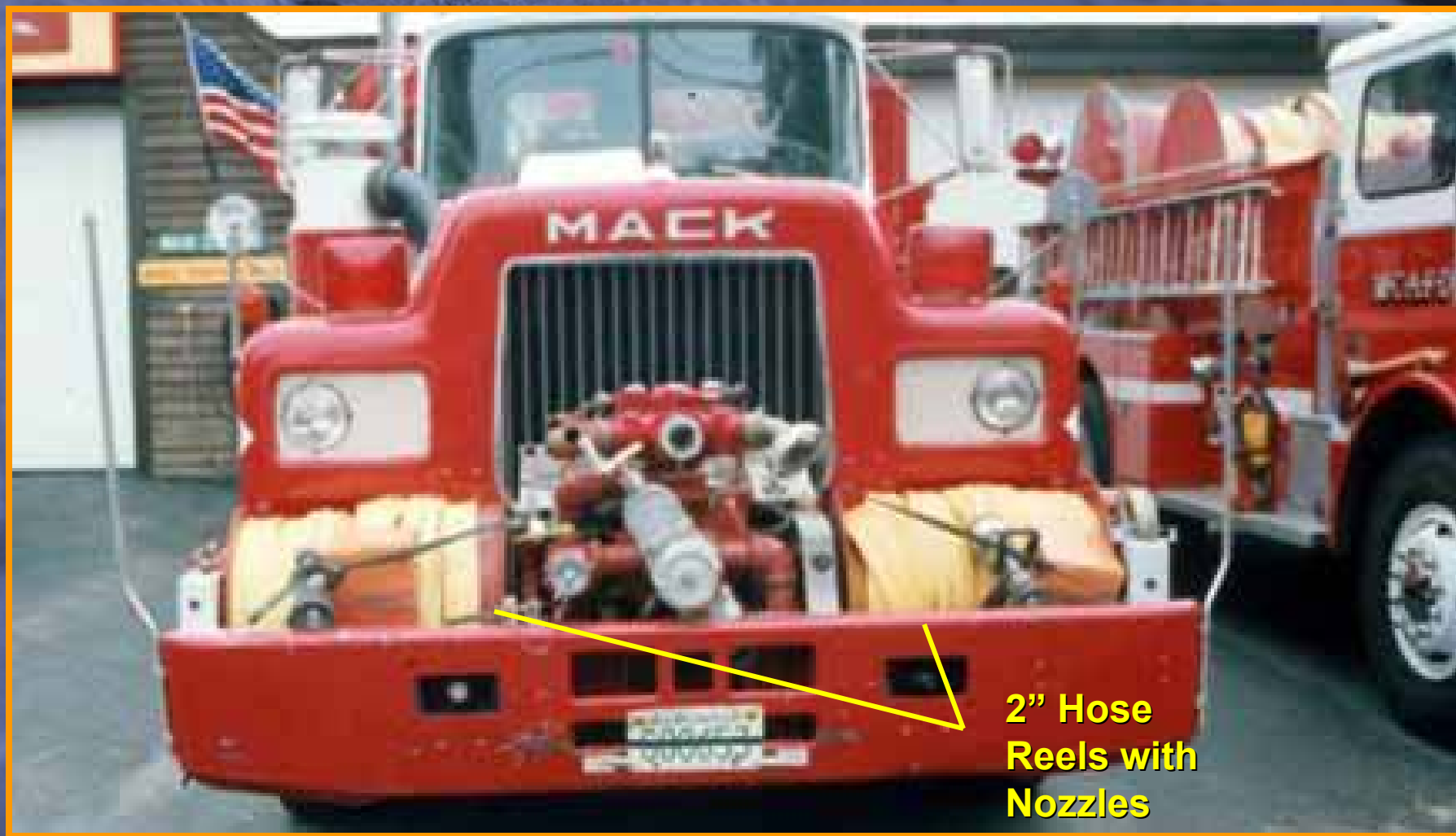
Figure 22. The attack unit features two reels that hold 2" hose with Storz couplings in the front bumper. These lines are not preconnected, but they are extended, disconnected from the reel, and attached to the pump outlets.
