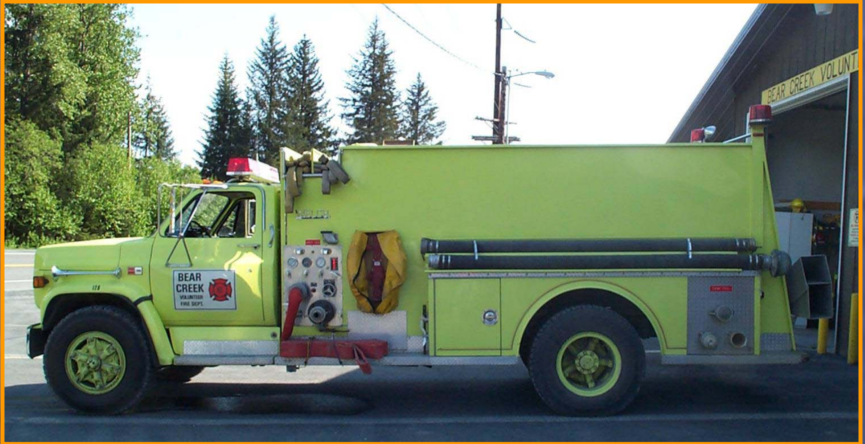
Figure 13. The tanker is primarily intended to transport water but can be used in initial fire attack operations if required.
