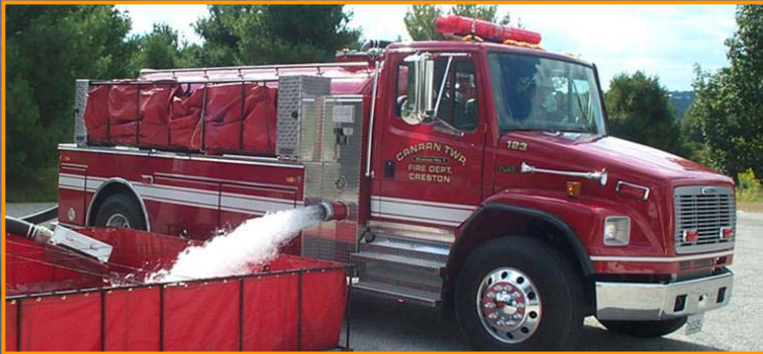
Figure 15. By using the pump's pressure mode to pressurize the tank, the tank can off-load at 1000+ gpm.
