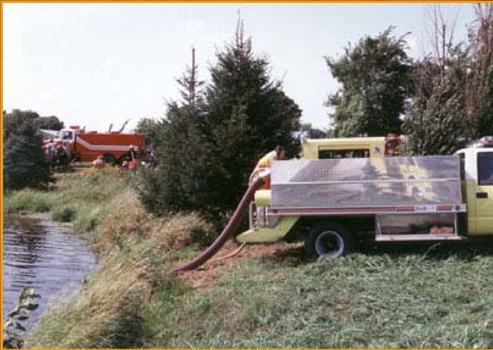
Figure 12. In this situation, the pump is supplying a 5" line to a manifold for tanker filling.
