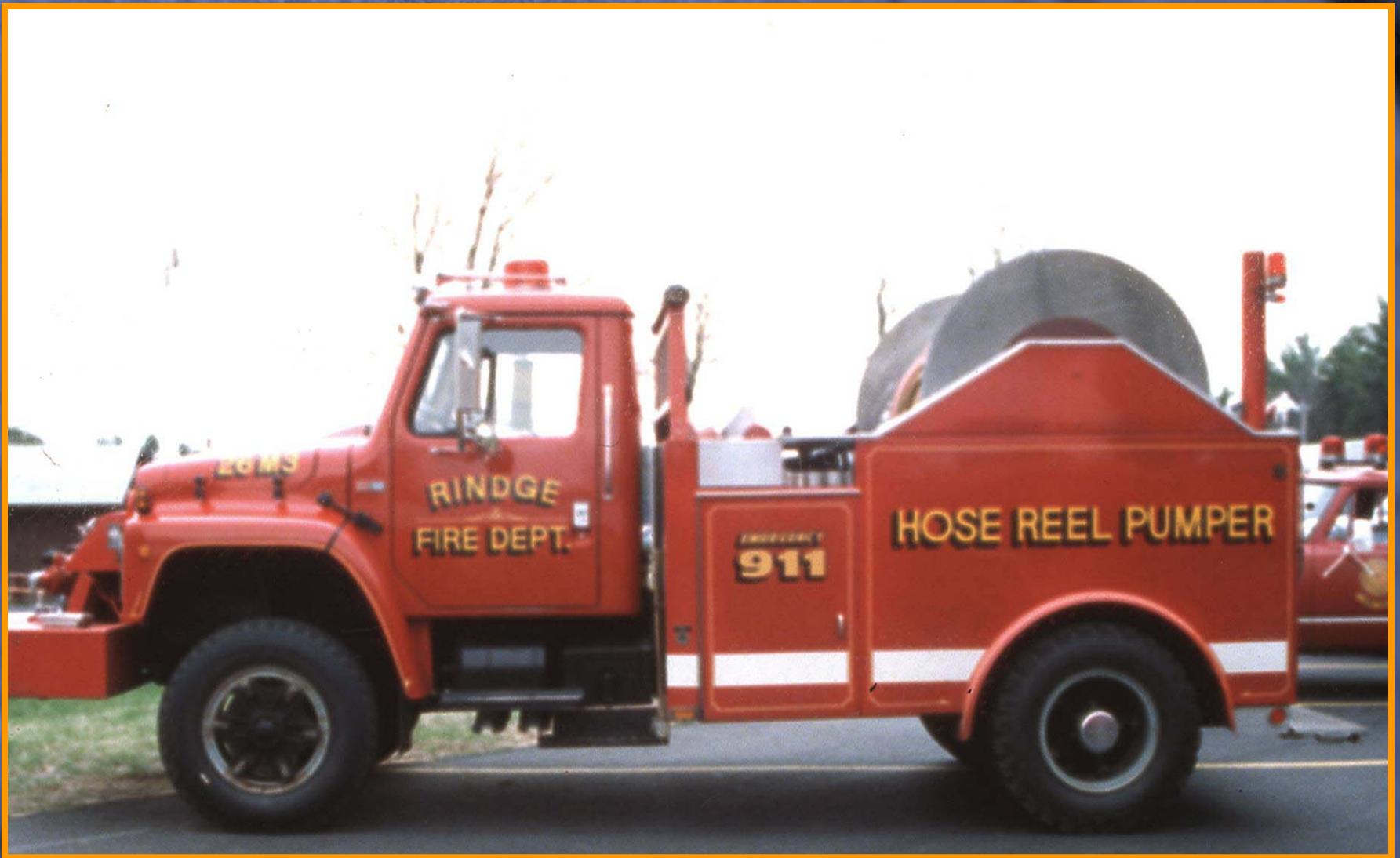
Figure 9. The hose reel pumper carries 4" hose on the reel. The unit's short overall length allows it to be easily maneuvered into tight spots.
