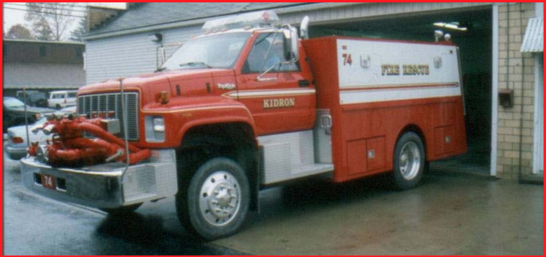
Figure 4. Other than having the front-mount pump mounted to the chassis, the volunteers completely built this unit.
