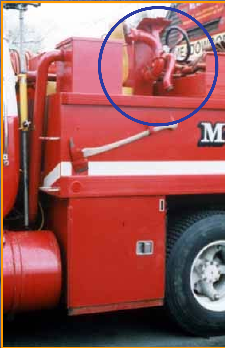
Figures 23. The portable monitor with preconnected hoses attached is carried for use in blitz attacks.
