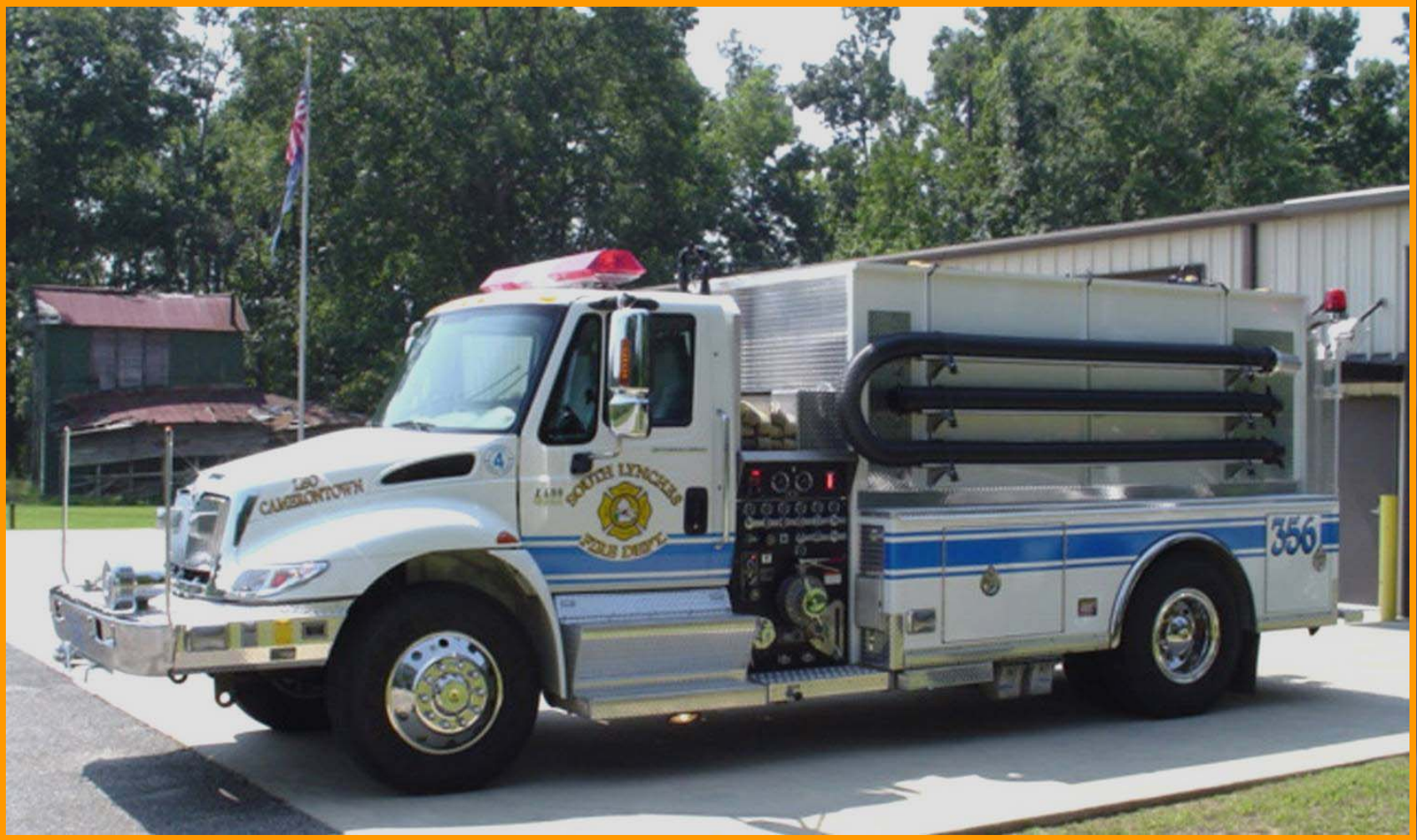
Figure 19. The tanker/pumpers are primarily designed to haul water to attack apparatus. However, they can also be used for fire attack if needed. Each unit is equipped with long suction hoses for drafting if needed, and a rear jet dump. A discharge in the front bumper can be used to nurse an engine using 3" hose.
