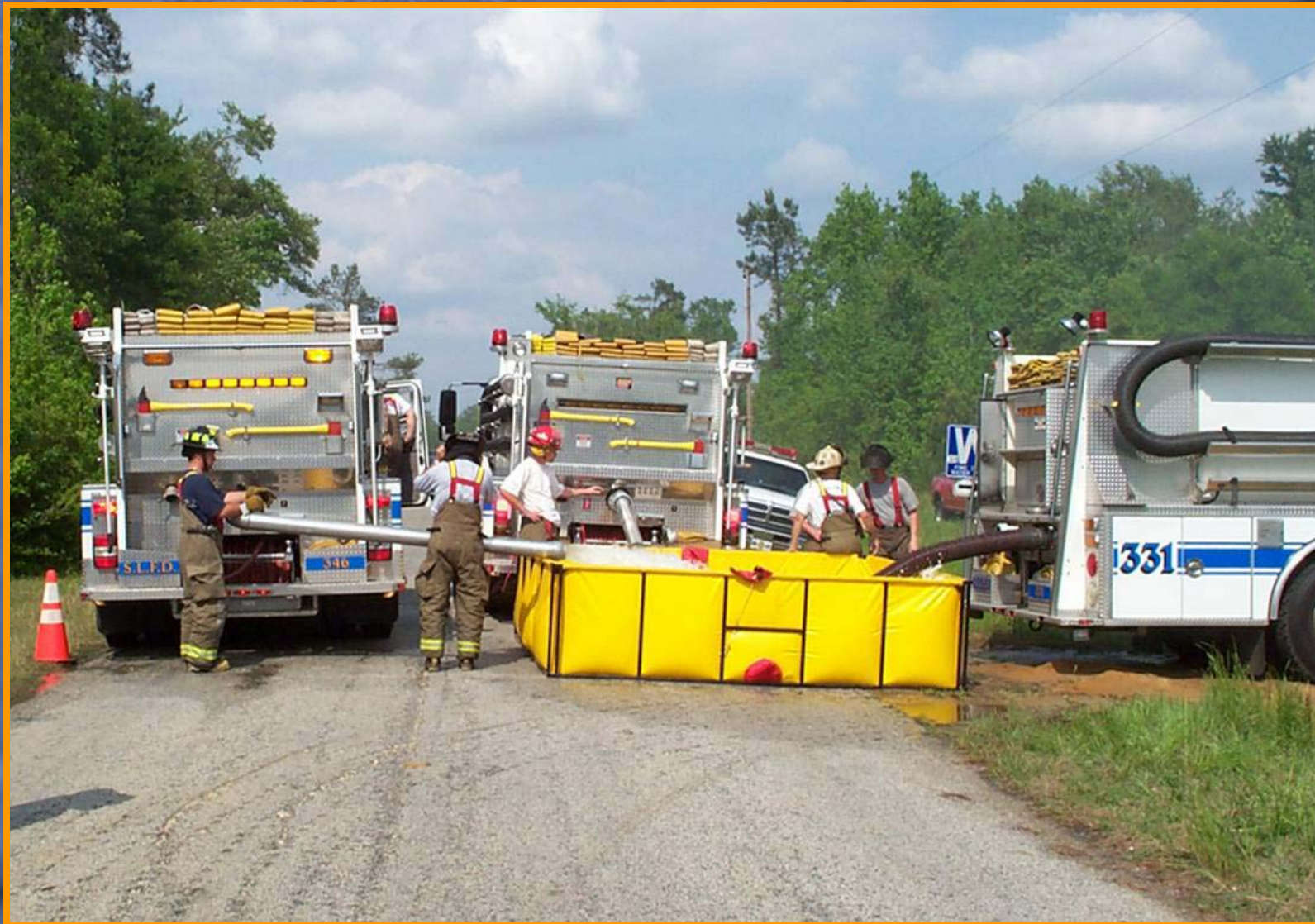
Figure 20. The South Lynches water shuttle in operation showing an engine using a rear suction to draft from a porta-tank while two tankers use their jet dumps and extensions to off-load into the porta-tank.
