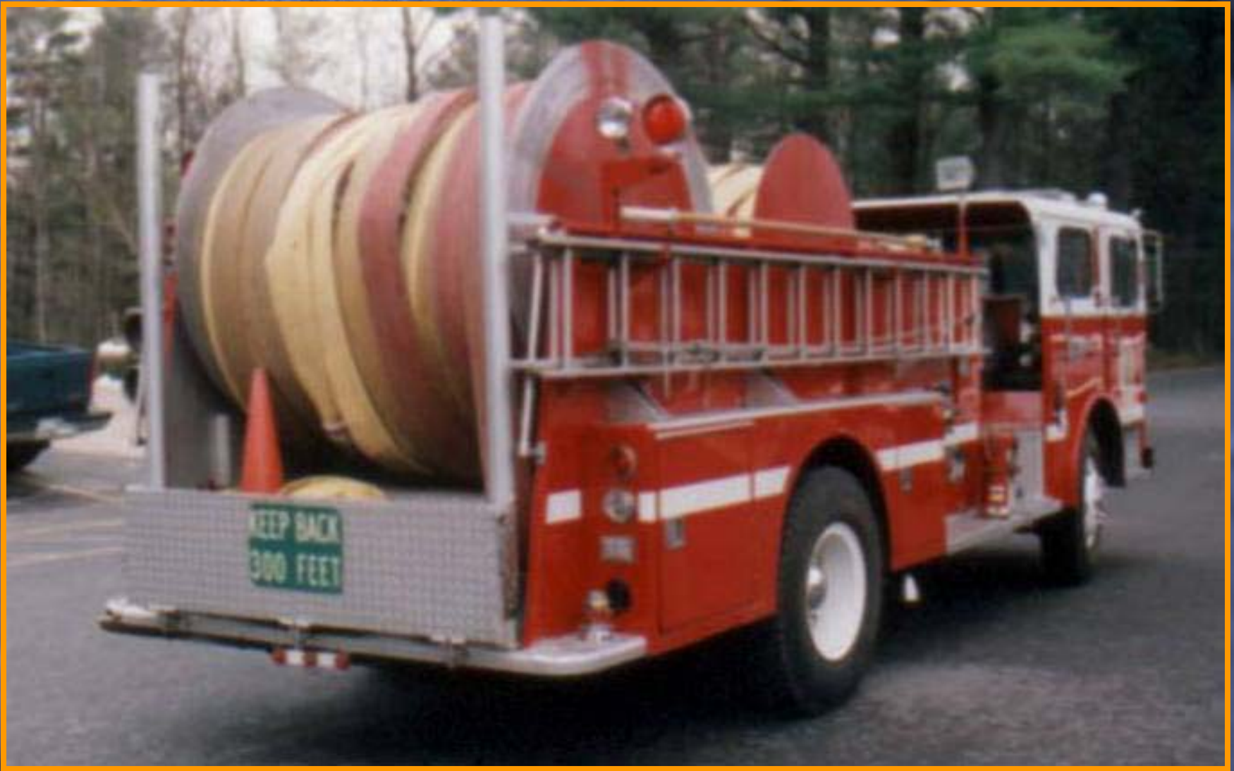
Figures 26. The unit's several thousands of feet of 4" are carried on two reels to keep from overloading a single reel.
