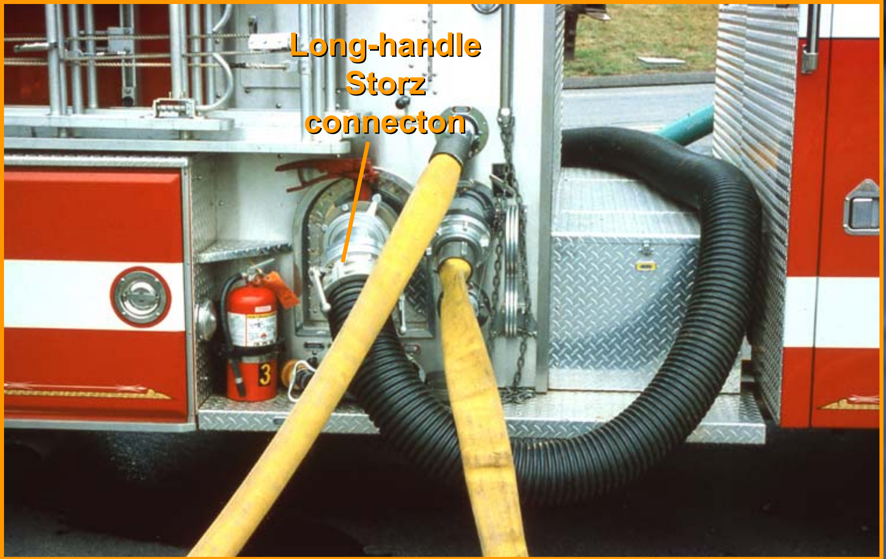
Figure 7. With the flexible Kochek suction hose, a second suction from the right side can be run through the walkway for the top-mount pump panel. With dual suctions, the 1250-gpm pumper can easily deliver 2000 gpm.
