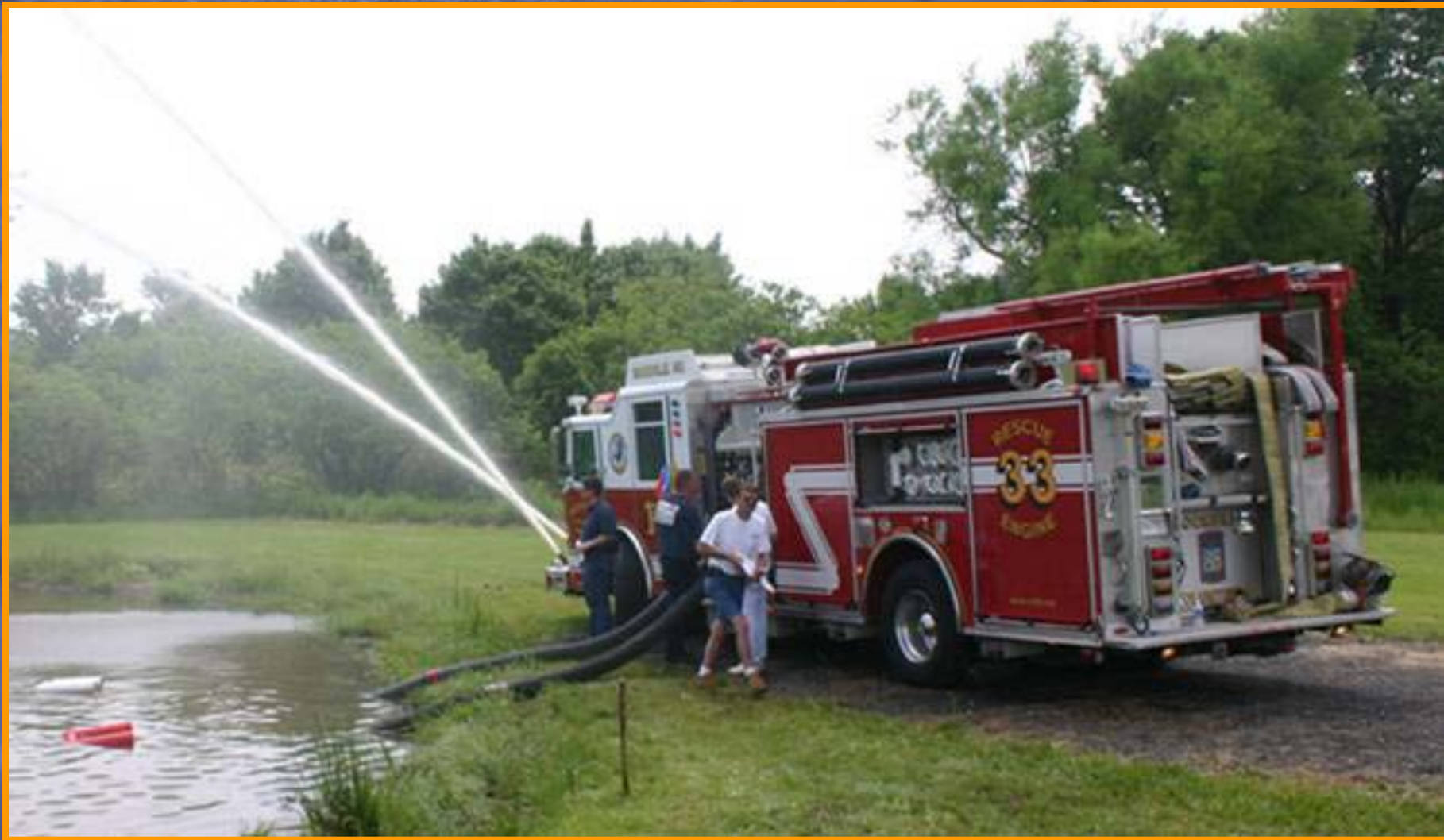
Figure 15. Rockville (MD) VFD's 2000-gpm pumper drafting with dual 6" suctions connected to a Kochek jumbo siamese.
