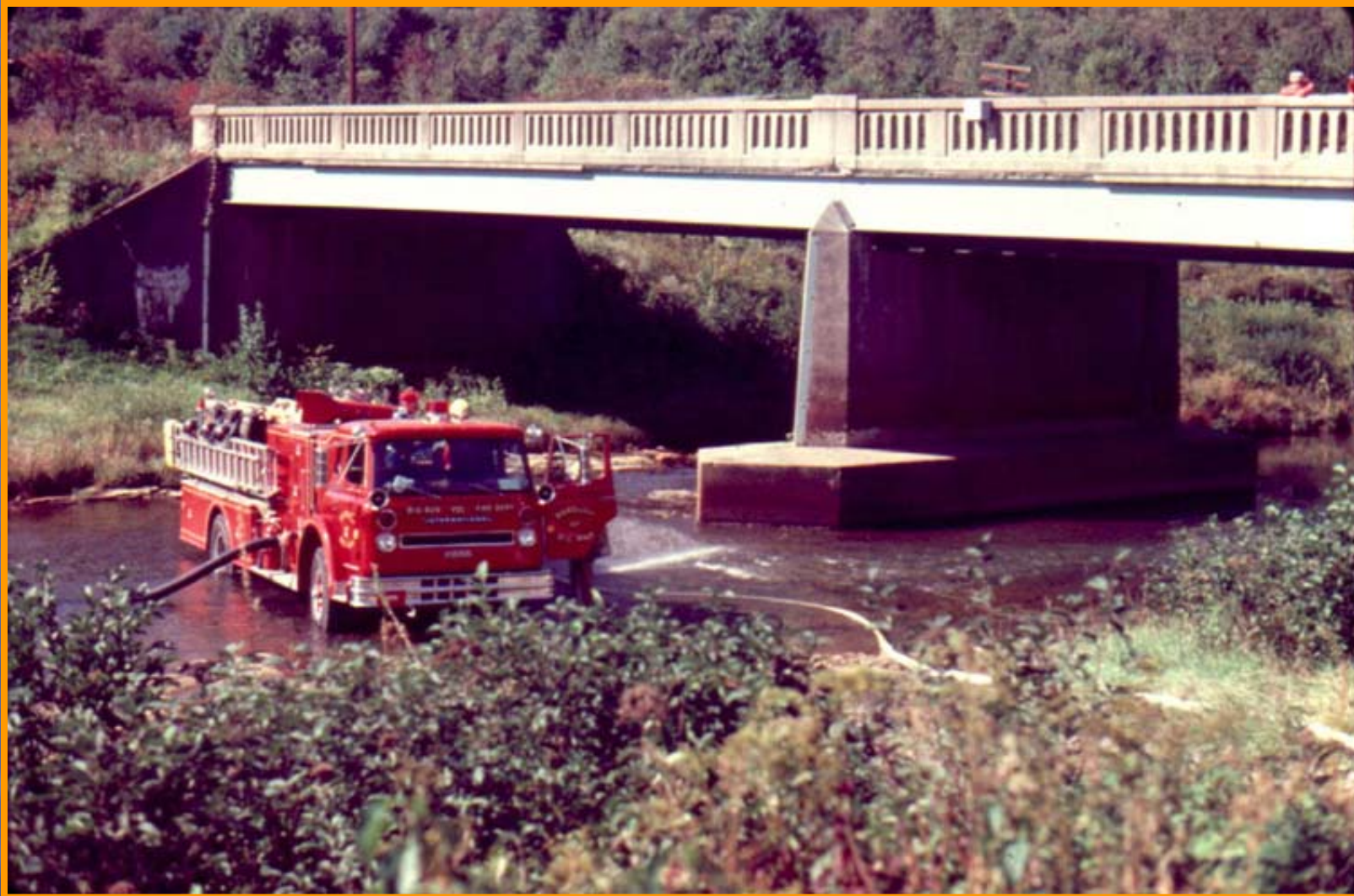
Figure 3. The Big Run (PA) VFD found a great way to reduce static lift in setting up this tanker fill site — simply back the engine into the stream. A decent roadway and a solid stream bed certainly helped maximize tanker fill rates.
