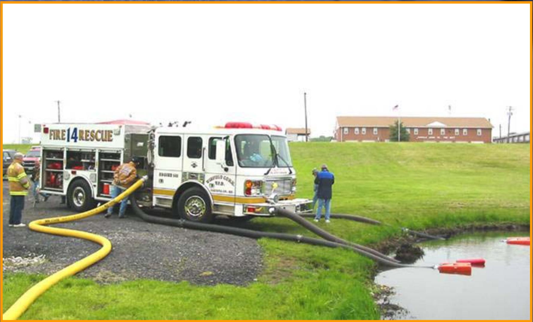
Figure 13. A test of Winfield Community (MD) VFD's 1500-gpm pumper, used 3 suction lines — both side suctions and the front suction — to deliver over 2300 gpm.
