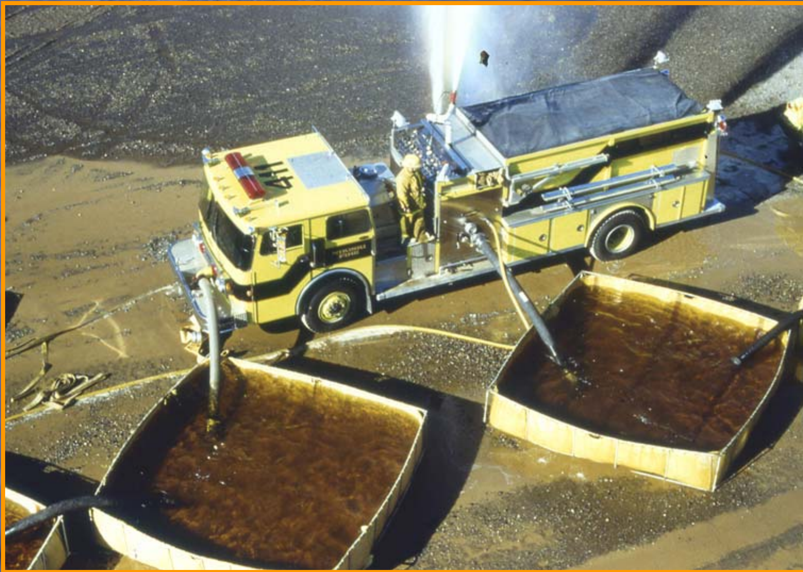
Figure 11. The Nikiski (AK) FD designed two 2000-gpm pumpers with front suctions so that dual suctions could be used to maximize flow of the dump site pumper in shuttle operations. Here Engine 411 drafts from two porta-tanks on one side to deliver over 1000 gpm.
