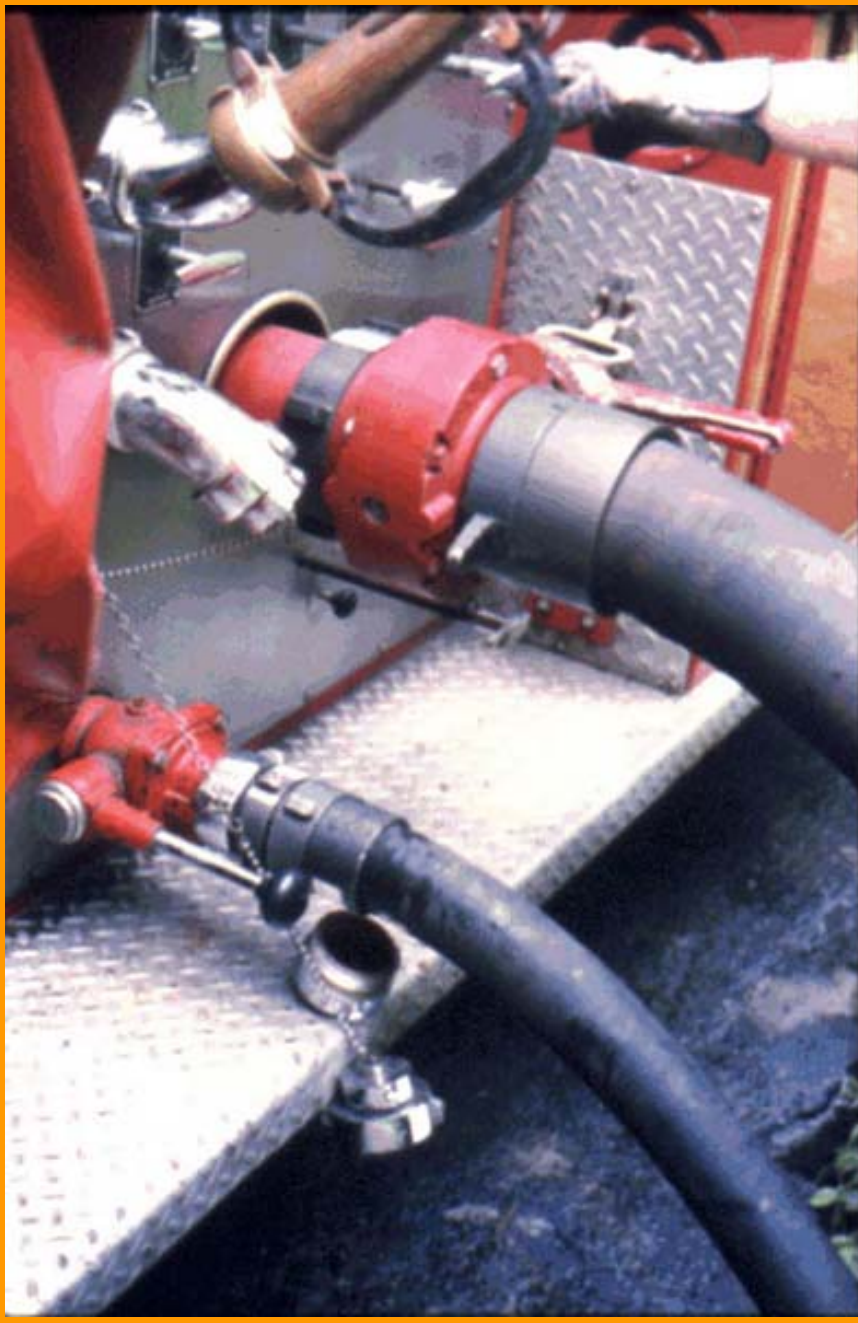
Figure 17. This Rhode Island pumper uses both 5" and 2-1/2" suctions to improve flow into the pump at a tanker fill site.
