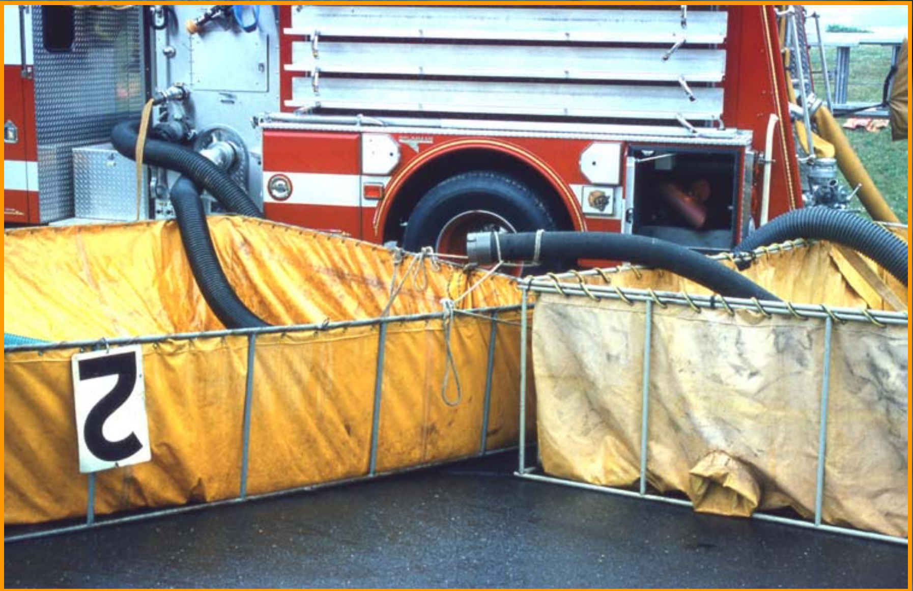
Figure 6. Middlefield uses dual 6" suctions from two porta-tanks at a water shuttle dump site.
