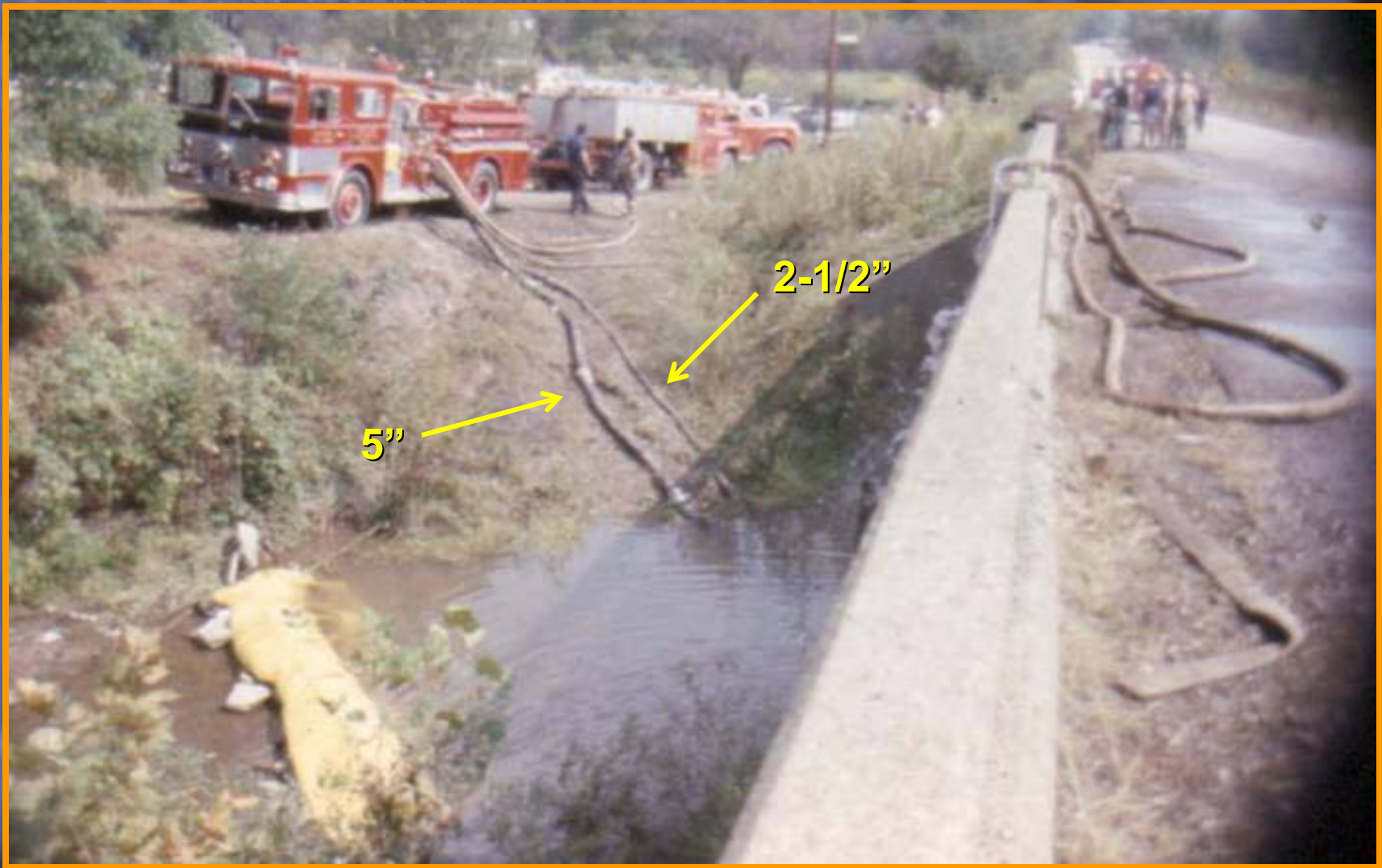
Figure 18. The Muse (PA) VFD's 1000-gpm pumper utilizes both 5" and 2-1/2" suctions to draft from a dammed-up stream to fill tankers.
