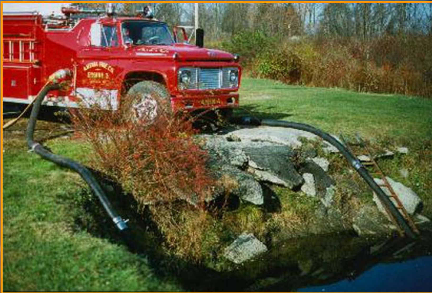
Figure 10. The Amenia (NY) VFD utilized dual 30-ft suctions to supply this pumper being used as a source pumper for a tanker fill site. Dual suctions maximized fill capability.
