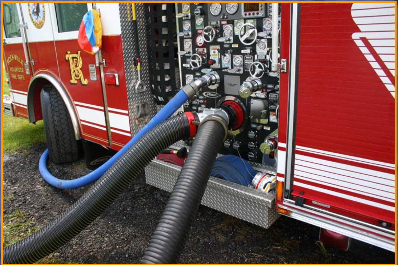
Figure 16. The Kochek jumbo siamese can significantly improve a pump's drafting capability through a single 6" suction intake.
