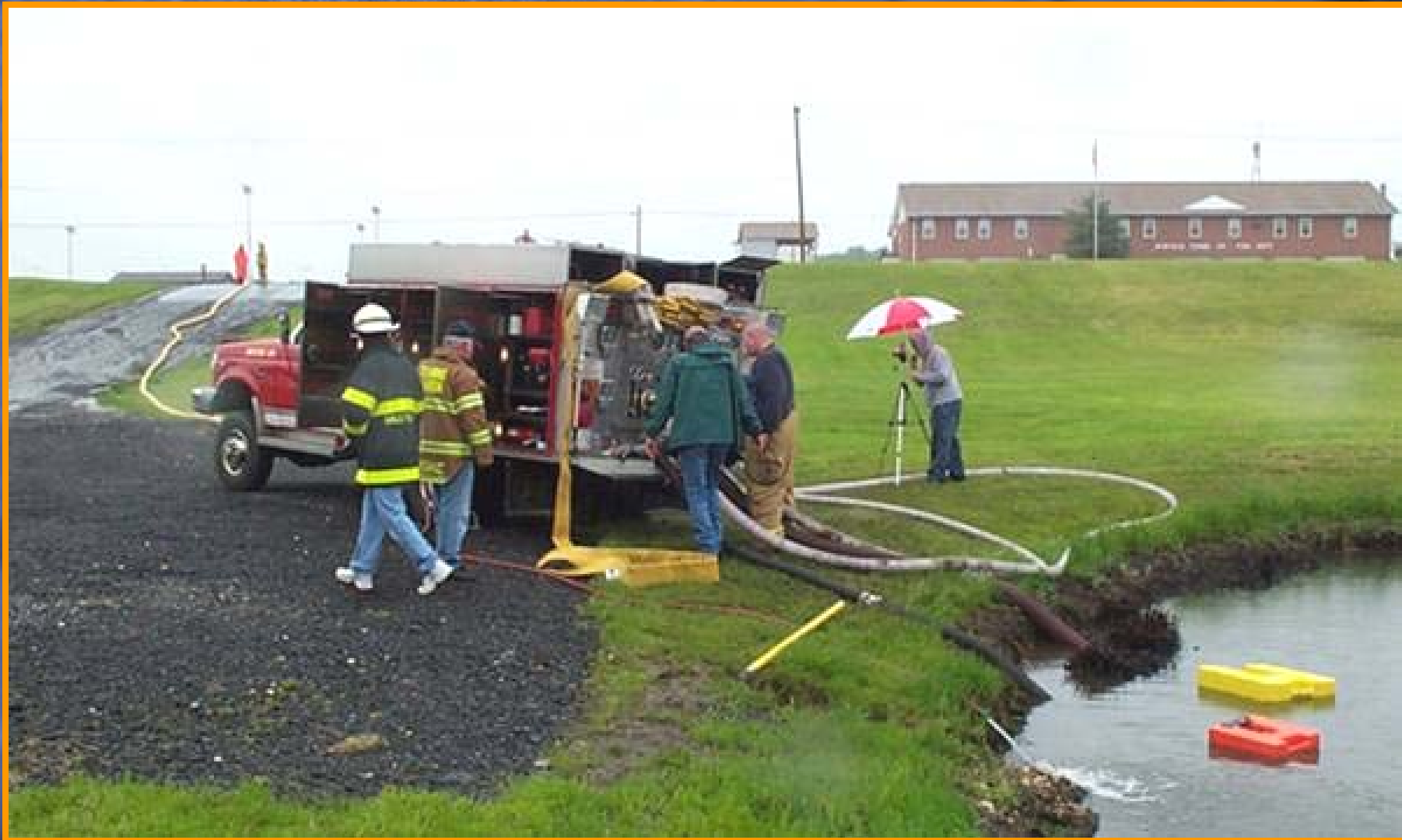
Figure 19. The Gamber Community (MD) VFD's 750-gpm rear-mount pumper delivered over 1100 gpm when a 2-1/2" suction was used to supplement the 4-1/2" suction. The pumper supplies a 5" line to a manifold for use in filling tankers.
