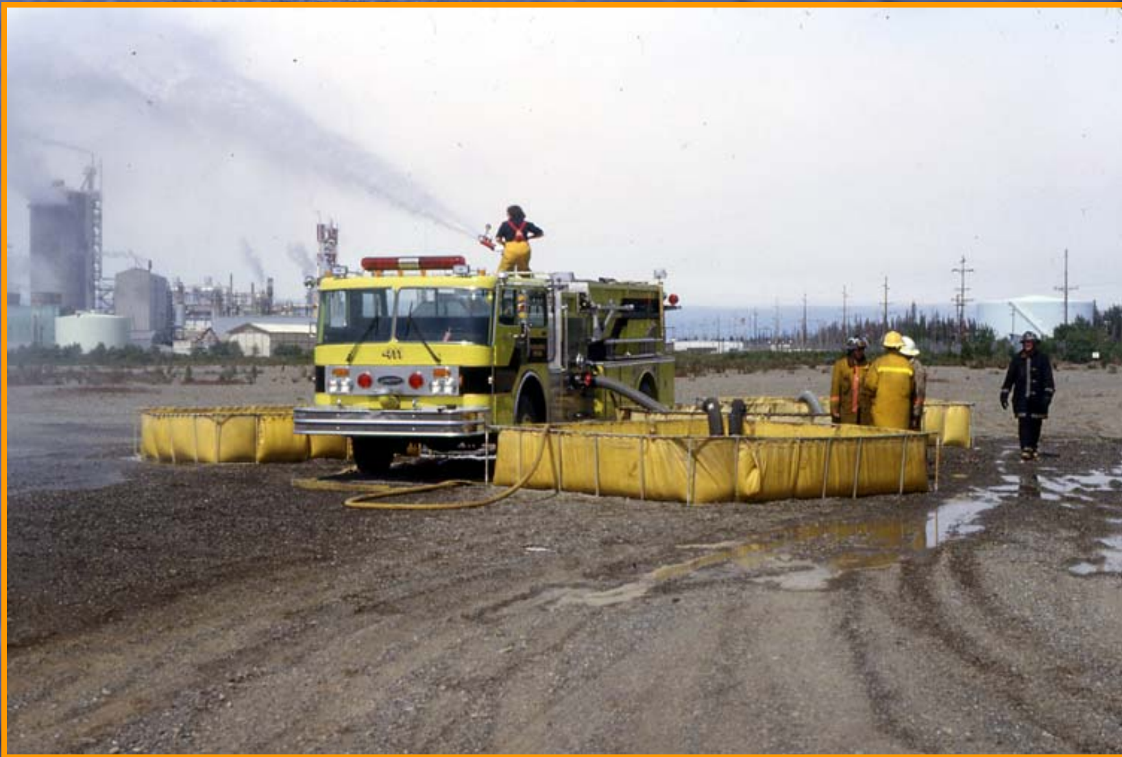
Figure 12. When needed, porta-tanks can be set up on each side of the dump site pumper. Here Engine 411 drafts from porta-tanks on both sides.
