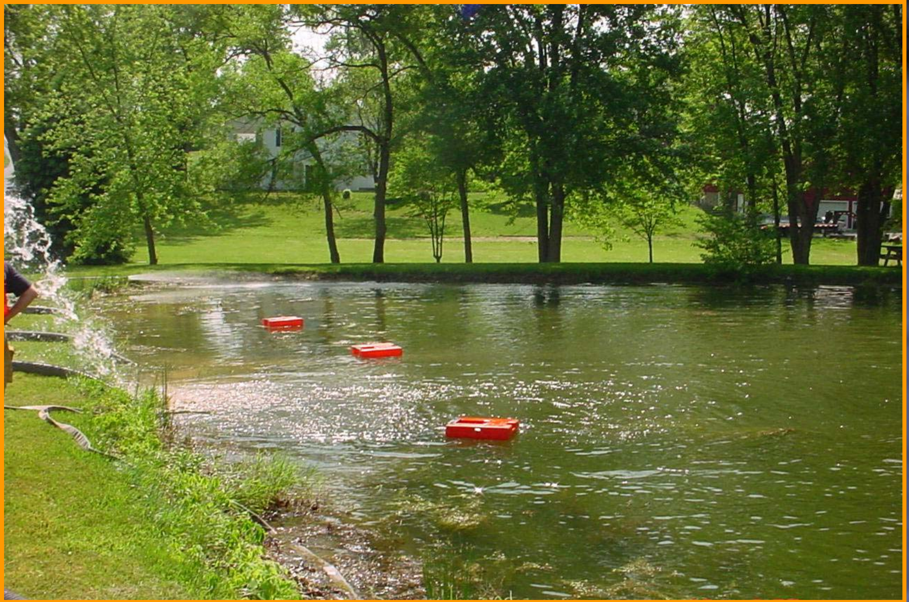
Figure 11. During a water supply drill, two pumpers using three suctions with floating strainers were used to draft water from the pond to fill tankers.
