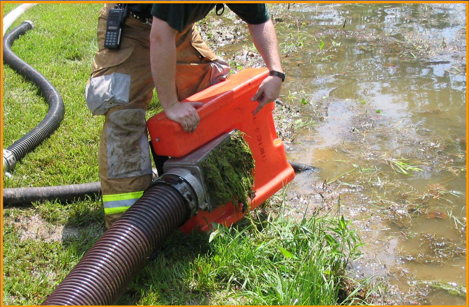
Figure 12. A major problem arose when the vegetation clogged and actually collapsed the metal strainer portion of the floating strainers. This occurred in a matter of a couple of minutes because of the force of atmospheric pressure pushing the vegetation as well as water into the suction hose when the pumpers were drafting.
