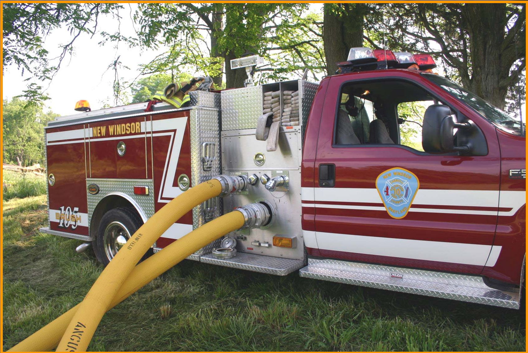
Figure 18. The 1000-gpm attack pumper showing the 5" intake and discharge lines that allowed the Mini to supply it with full capacity when needed.
