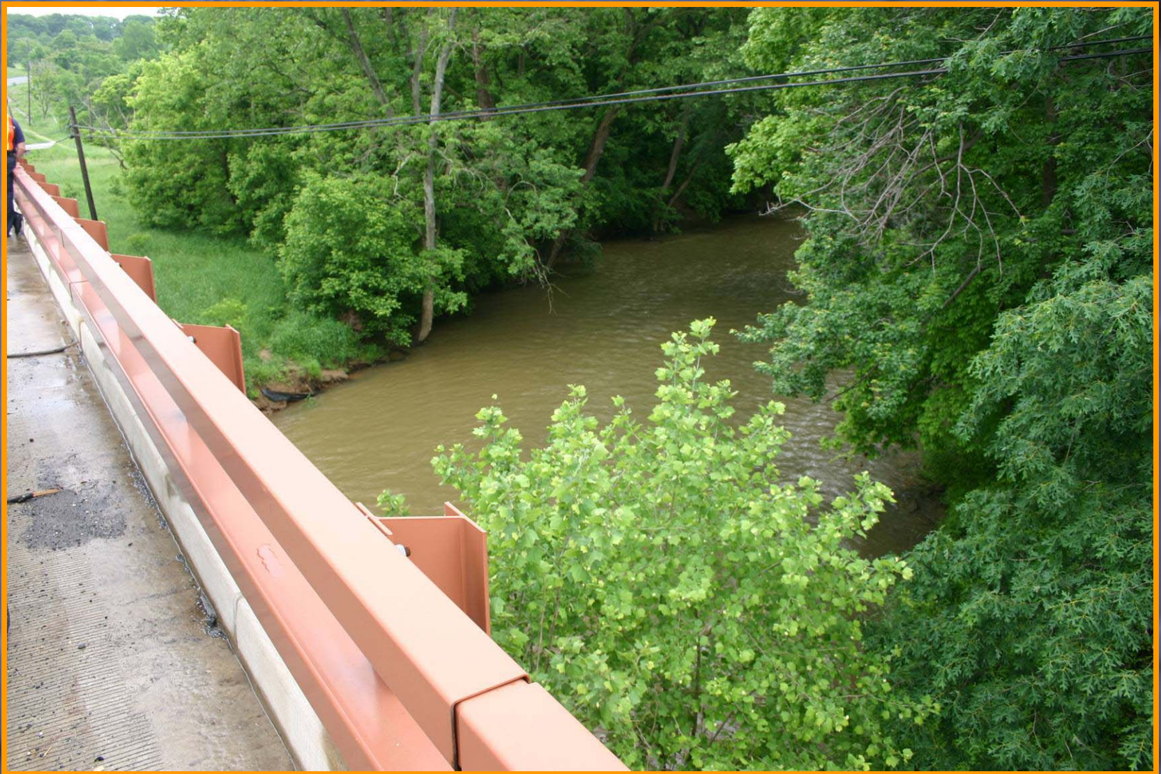
Figure 5. The problem: a very good water supply for either a relay operation or a tanker-filling operation but because of the 33-ft lift it is of little use.
