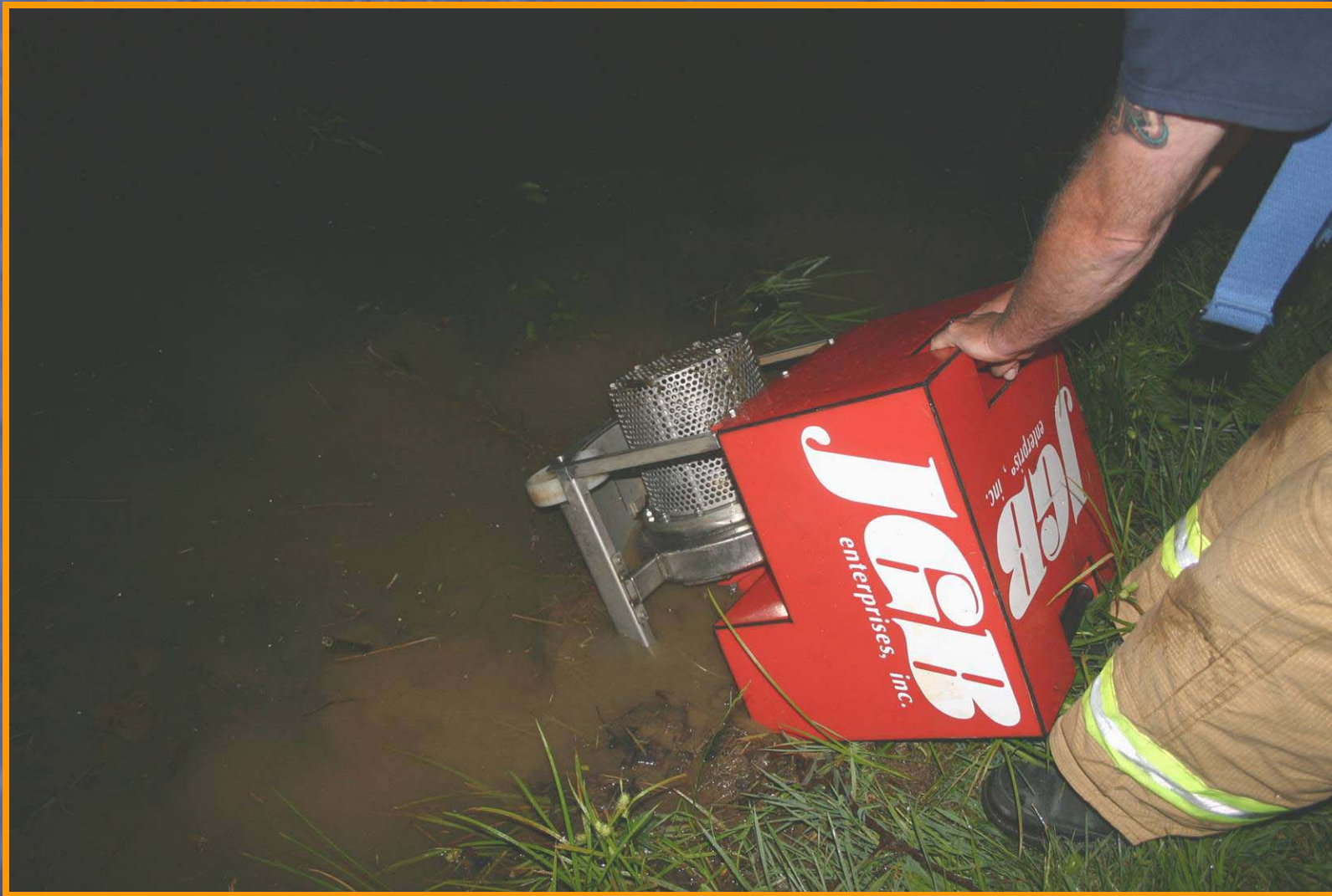
Figure 14. After 10 minutes of supplying 1000 gpm, the Mini was shutdown and pulled from the water. Notice there is no vegetation on the strainer. This is because the pump is not operating under a vacuum which allows atmospheric pressure to force the vegetation to plug the strainer.
