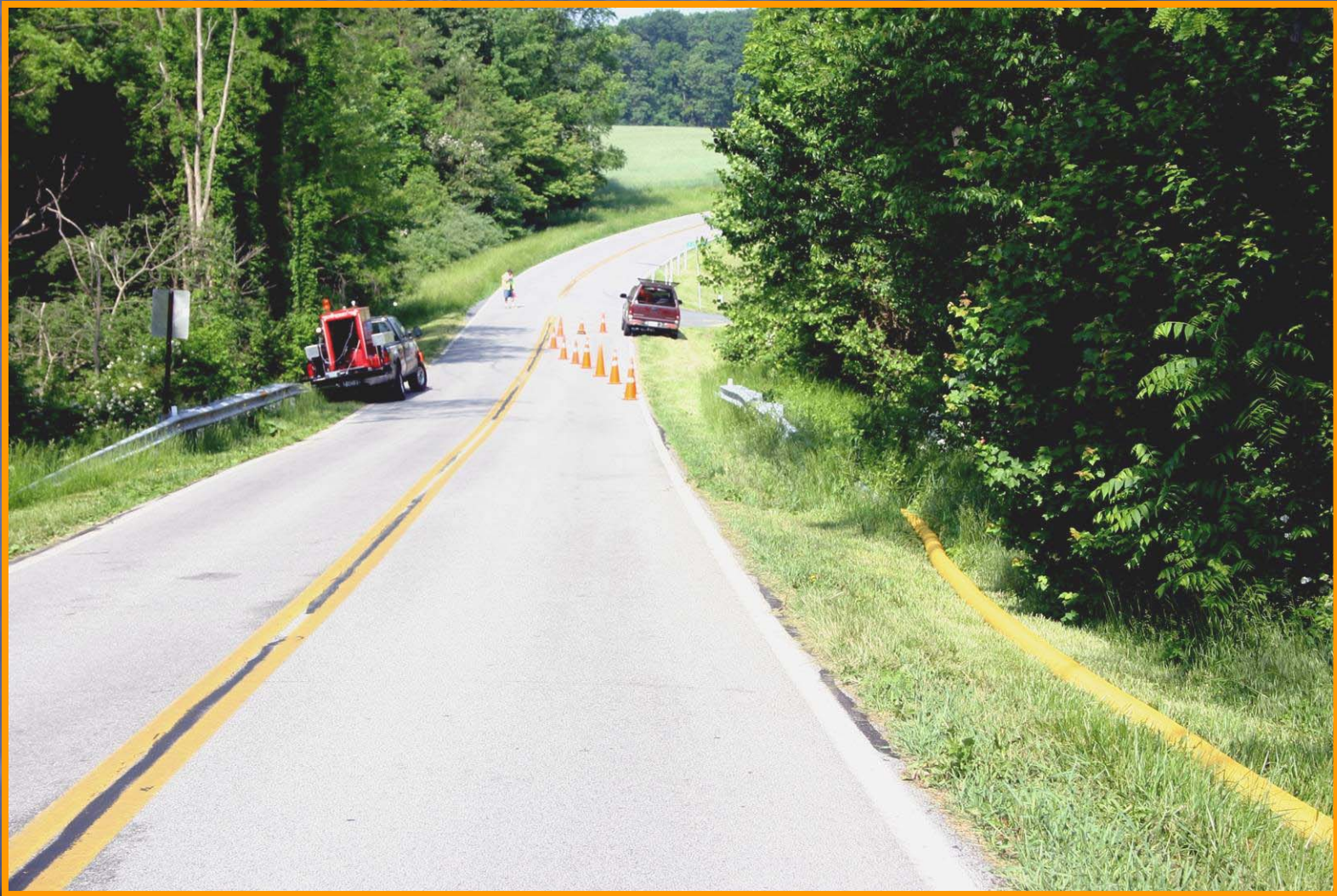
Figure 15. The Mini operates along the south side of the road to pump through a 5" line that runs in a culvert under the road and extends 600 feet to the attack pumper.
