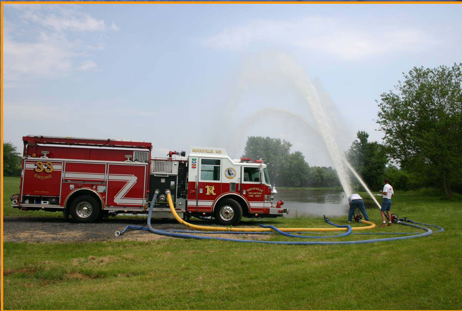
Figure 3. The Mini discharged through 100 feet of 5" to a 2000-gpm pumper which then supplied a TFT Crossfire and a TFT Blitzfire equipped with smoothbore nozzles to allow pitot readings to be taken to measure flow.
