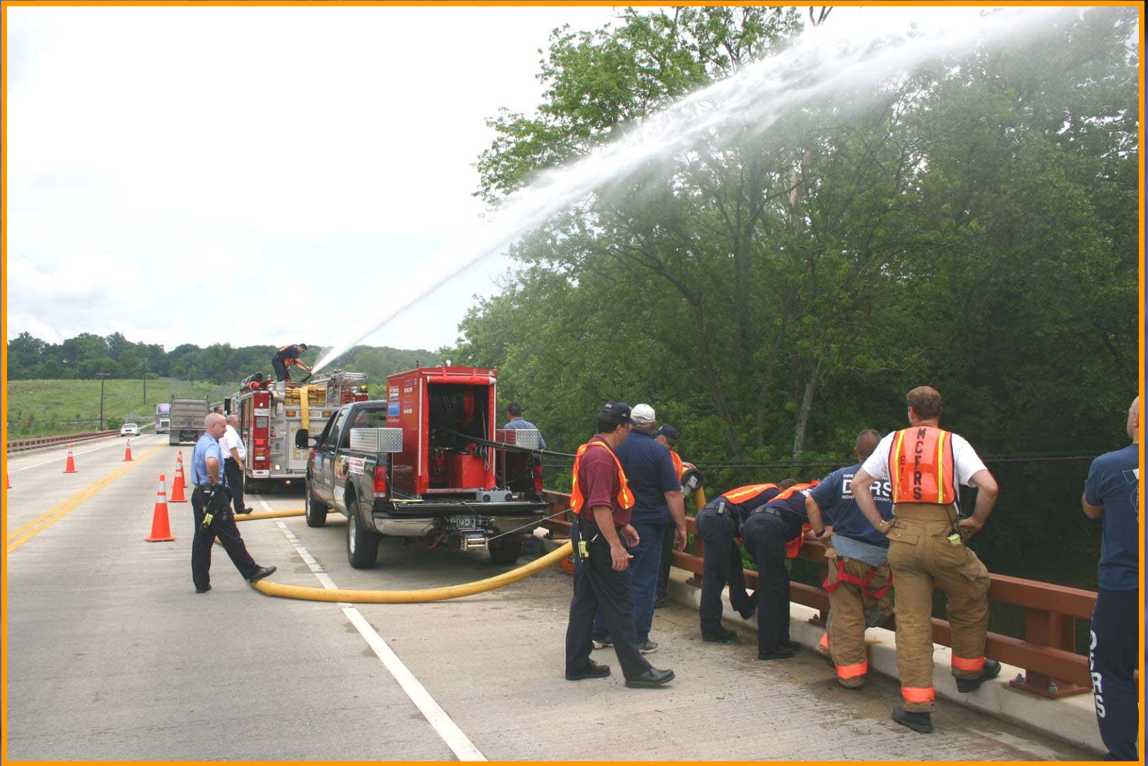
Figure 9. In this relay operation, the pumper is discharging 994 gpm from its deck gun. Naturally, a higher flow could have been achieved if 5" hose were used instead of 4". Not bad for a water supply that is otherwise inaccessible.
