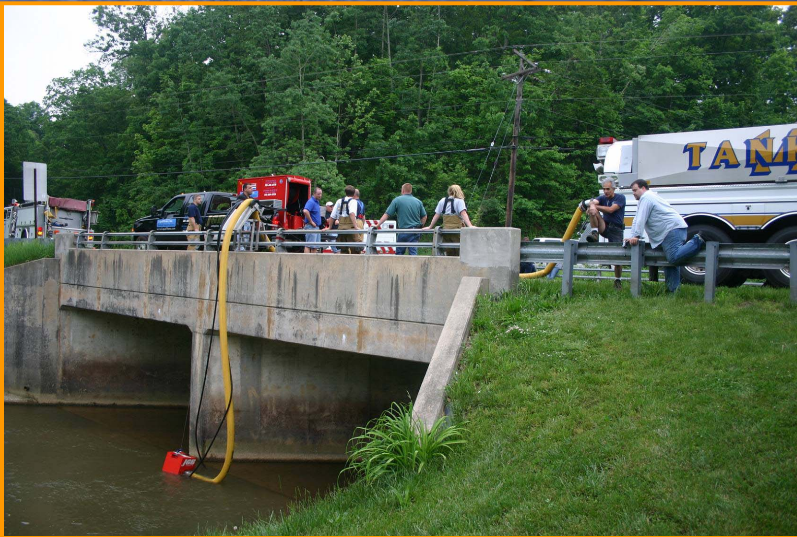
Figure 1. One of the Mini's major advantages is its ability to lift water without suction hose, a strainer, or a pump primer. During this test, the unit discharged through 100 feet of 5" hose to fill a tanker at just under 1000 gpm.
