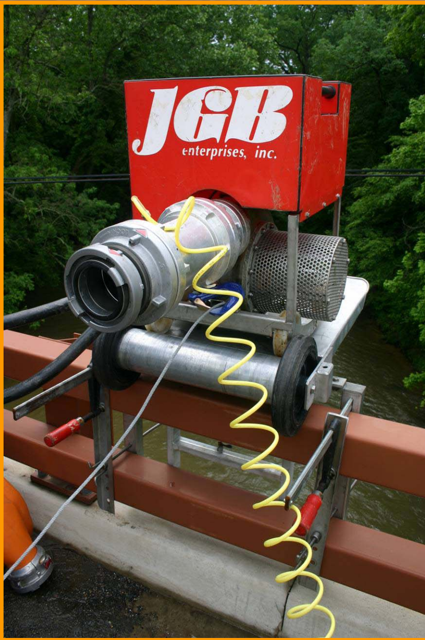
Figure 7. The Mini with gauge connection attached prior to the 4" discharge being connected.
