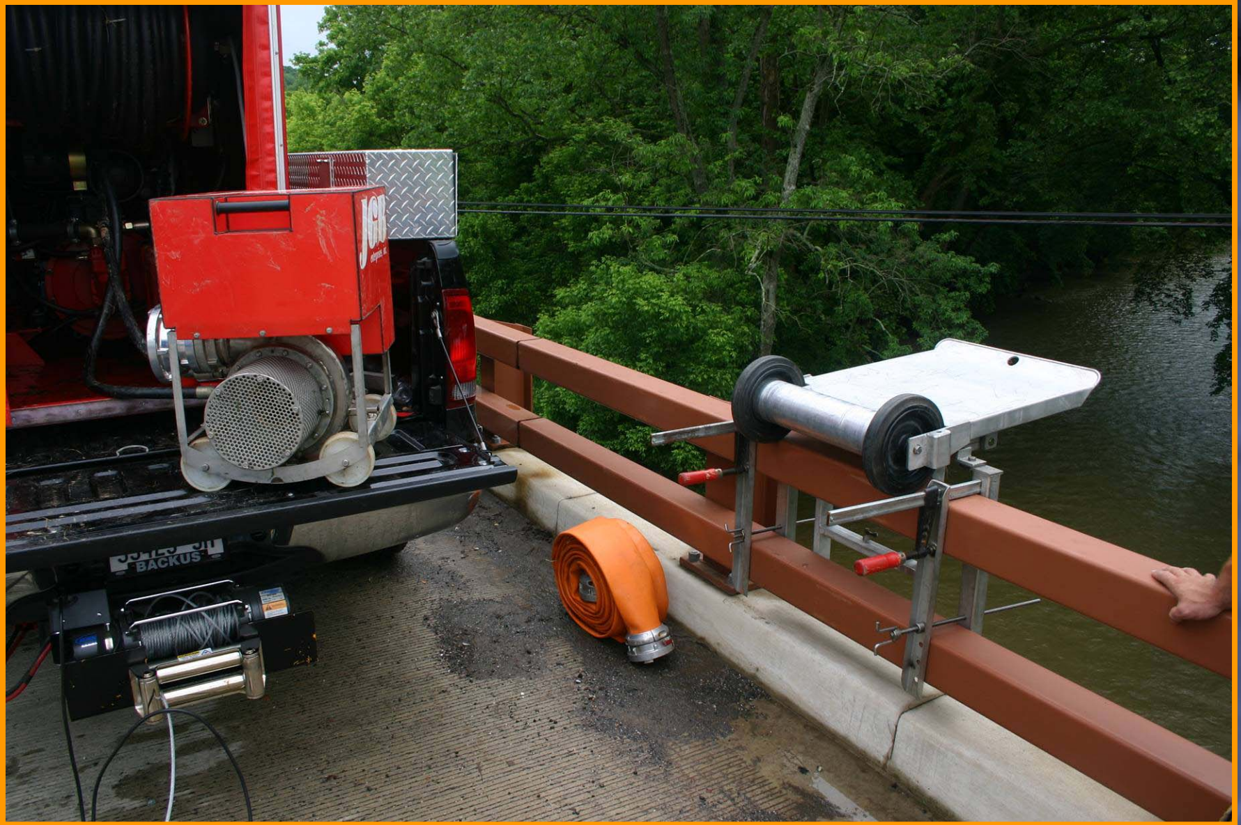
Figure 6. The bridge deployment mechanism attached to the bridge.
