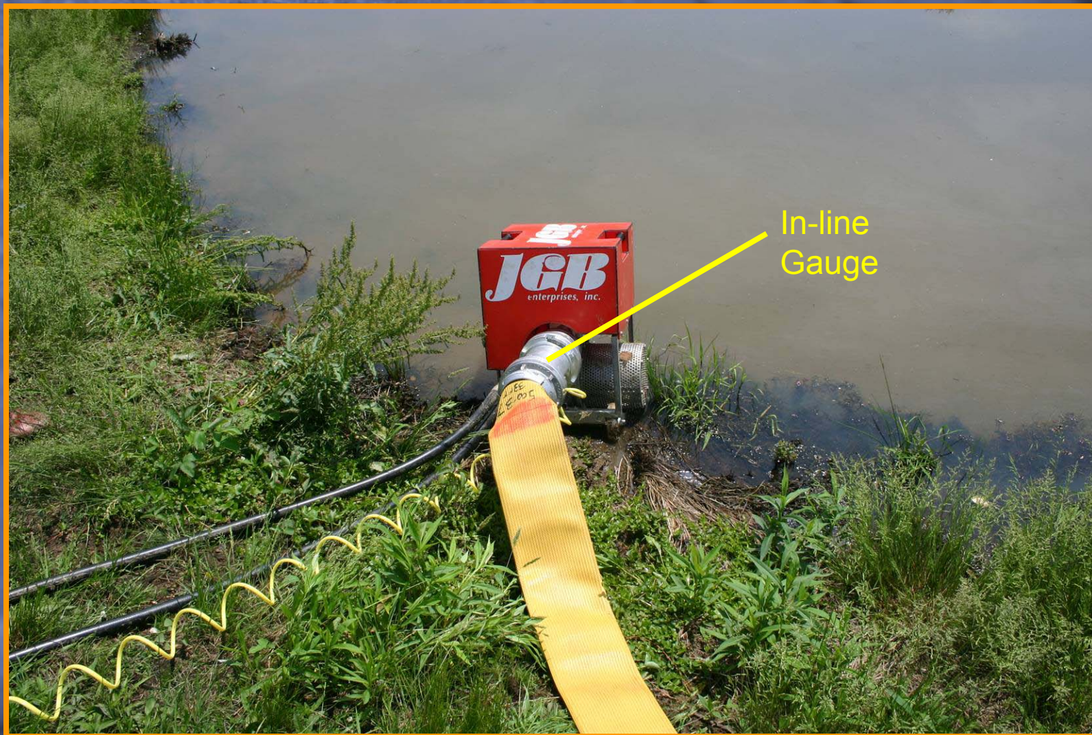
Figure 2. To measure the discharge pressure at the pump, a 5" in-line gauge was attached between the pump and the 5" discharge hose. The yellow coiled hose is 50 feet of 1/4" air hose to allow reading the discharge pressure while the pump was in the water.
