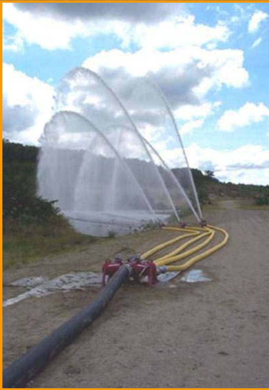
Figure 4. Pushing the envelope, this 8" hose, manufactured by Jaffrey and Oroflex for a petrochemical plant's fire department, delivers 3000 gpm to 4 portable monitors.
