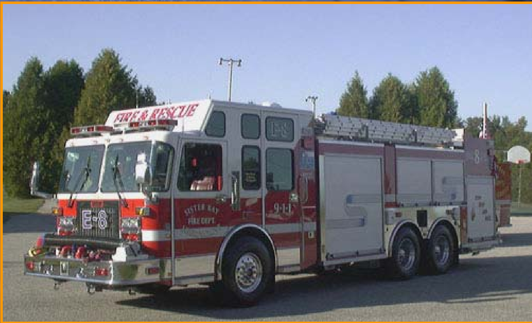
Figure 11. The mother of all fire assault apparatus. Chief Chris Hecht and the Sister Bat (WI) FD exhibit the “think biug, hit it hard” concept of rural firefighting. This pumper is equipped with a 2500-gpm, rear-mounted pump; a 200-cfm CAFS, a 2250-gal water tank, a 100-gal Class A foam tank; and 1500 ft of 5” hose.
