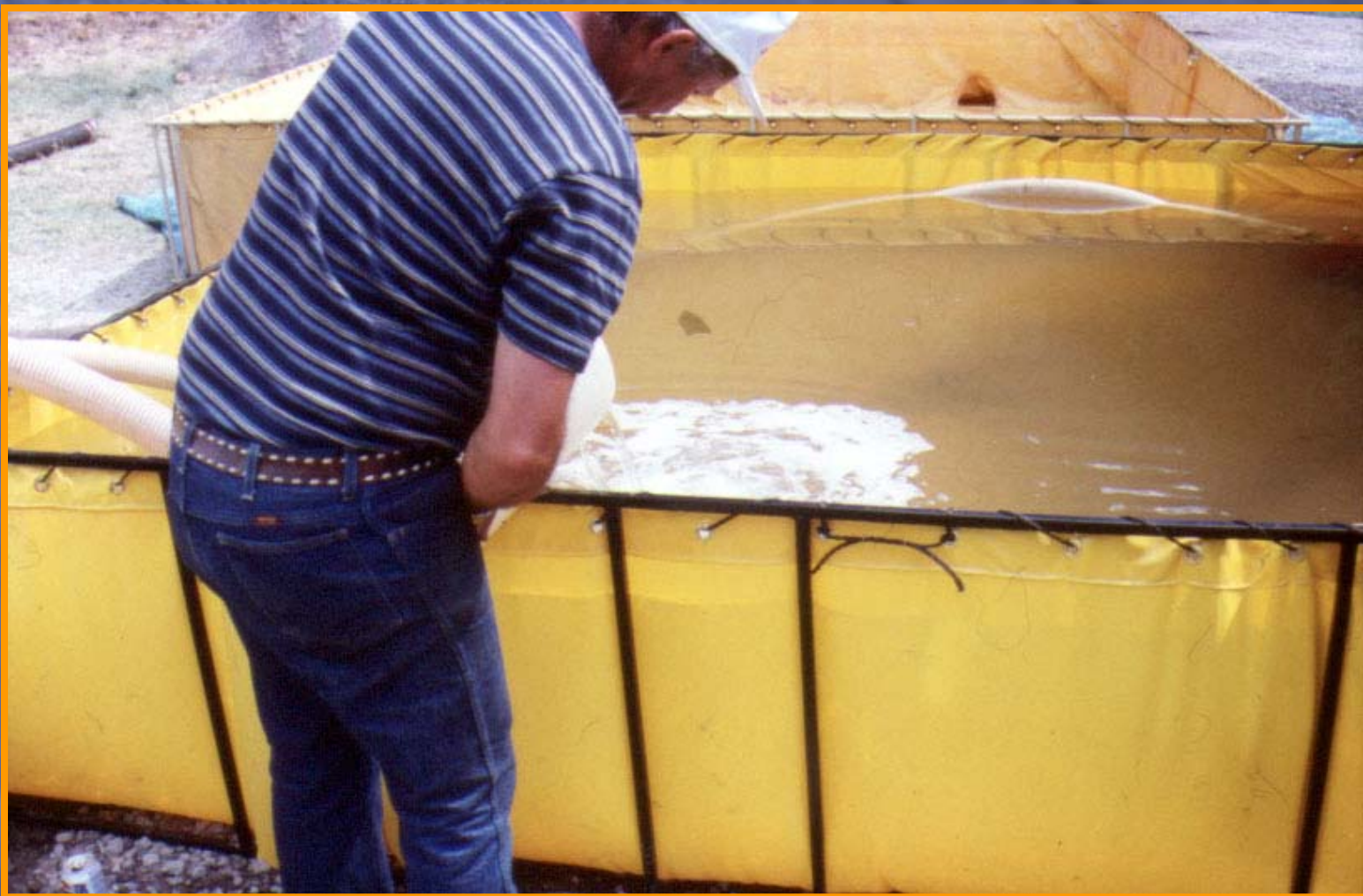
Figure 12. Don't have a Class A foam-equipped pumper? Want to double your water's effectiveness? Then batch mix Class A foam into your porta-tank at the rate of 1 gal of foam concentrate per 1000 gal of water (0.1%). The draft pumper can then supply Class A foam through all of its discharges with no need for foam proportioners or eductors.
