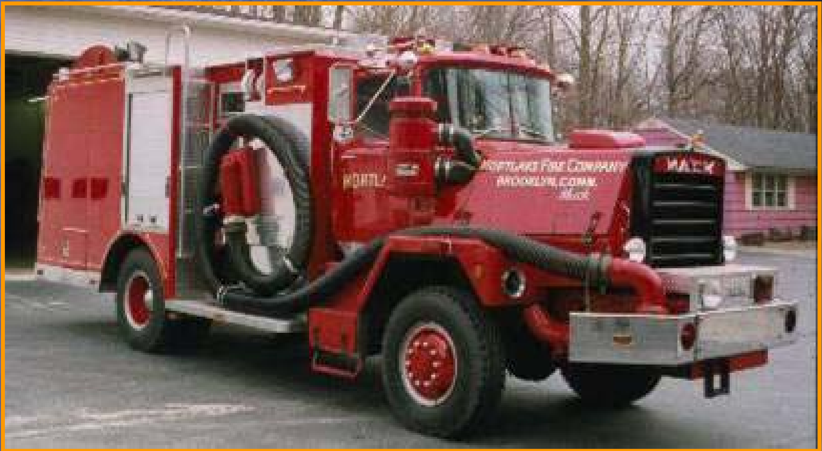
Figure 2. The Mort Lake Fire Co., Brooklyn (CT), resurrected an idea that was prevalent in the days of horse-drawn steamers—a preconnected suction line known as a “squirrel-tail” suction. Mort Lake’s 1500-gpm water-supply pumper carries a 28-ft x 6” squirrel tail preconnected to a 6” front suction. It has an additional 28-ft x 6” suction in a coil just ahead of the of the hose reel. The reel carries 5000 ft of 5” hose. A 15-hp vacuum pump, instead of a typical primer, allows the unit to prime from a 10-ft lift in 4 seconds. Dual suctions provide more than 2000 gpm. With this unit, 1 person can move more than 1000 gpm almost 1 mile.
