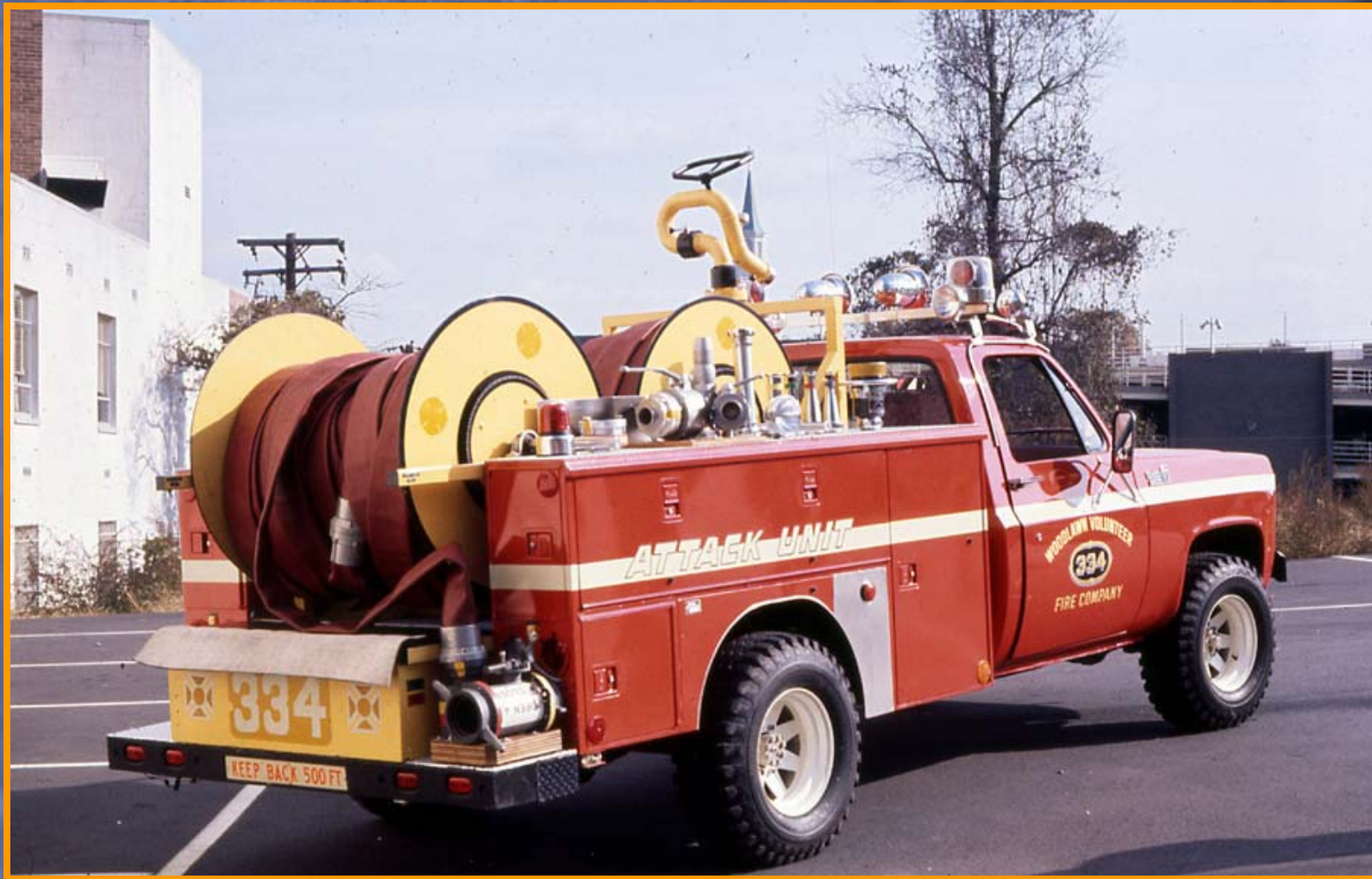
Figure 9. Rural departments often have to deal with long, narrow driveways. This Woodlawn (MD) attack rig, which has no pump or water tank, lays a 4" supply line from the main road up the driveway and into the truck's manifold. Responding engines or tankers then supply water to the attack unit. The unit carries 1-3/4" and 2-1/2" preconnects and a prepiped deck gun.
