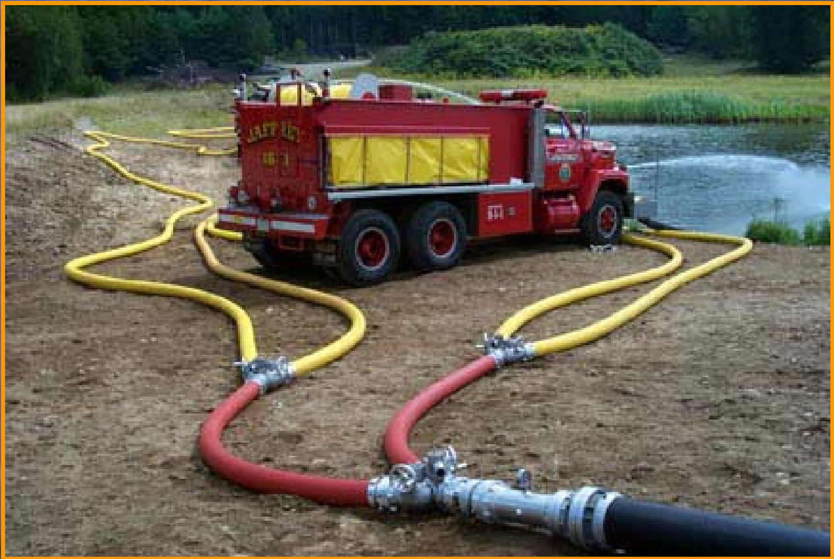
Figure 5. In drafting operations, pumps expend energy on the suction side by lifting water against friction loss and elevation loss, and on the discharge side by pushing water through pipes, hose, and appliances. Here four 5" lines (each supplied by a 1250-gpm pumper at draft) are supply the 8" hose.
