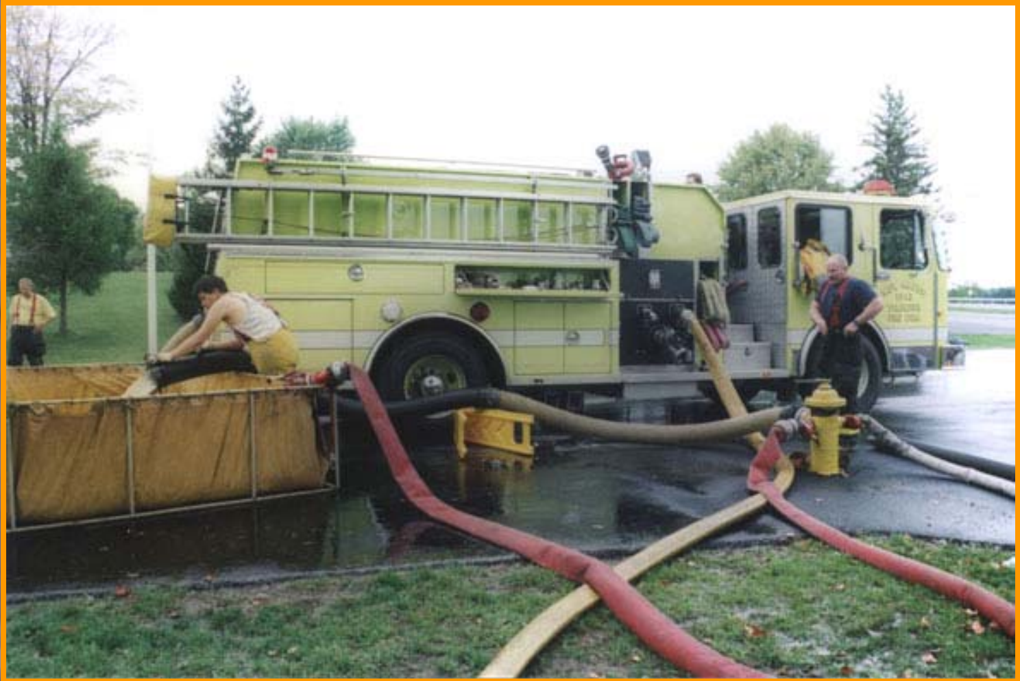
Figure 7. This is one of three fill sites used in a tanker shuttle drill in Oswego County (NY). Originally, the pumper was connected to the hydrant with a short length of 4" hose. The problem: The hydrant could only flow about 600 gpm, so the tanker's fill rate was 600 gpm as well. To maximize tanker filling, we set up a porta-tank, connected 6" hard suction from the hydrant into the porta-tank and set up the pumper to draft through its rear 6" suction.
