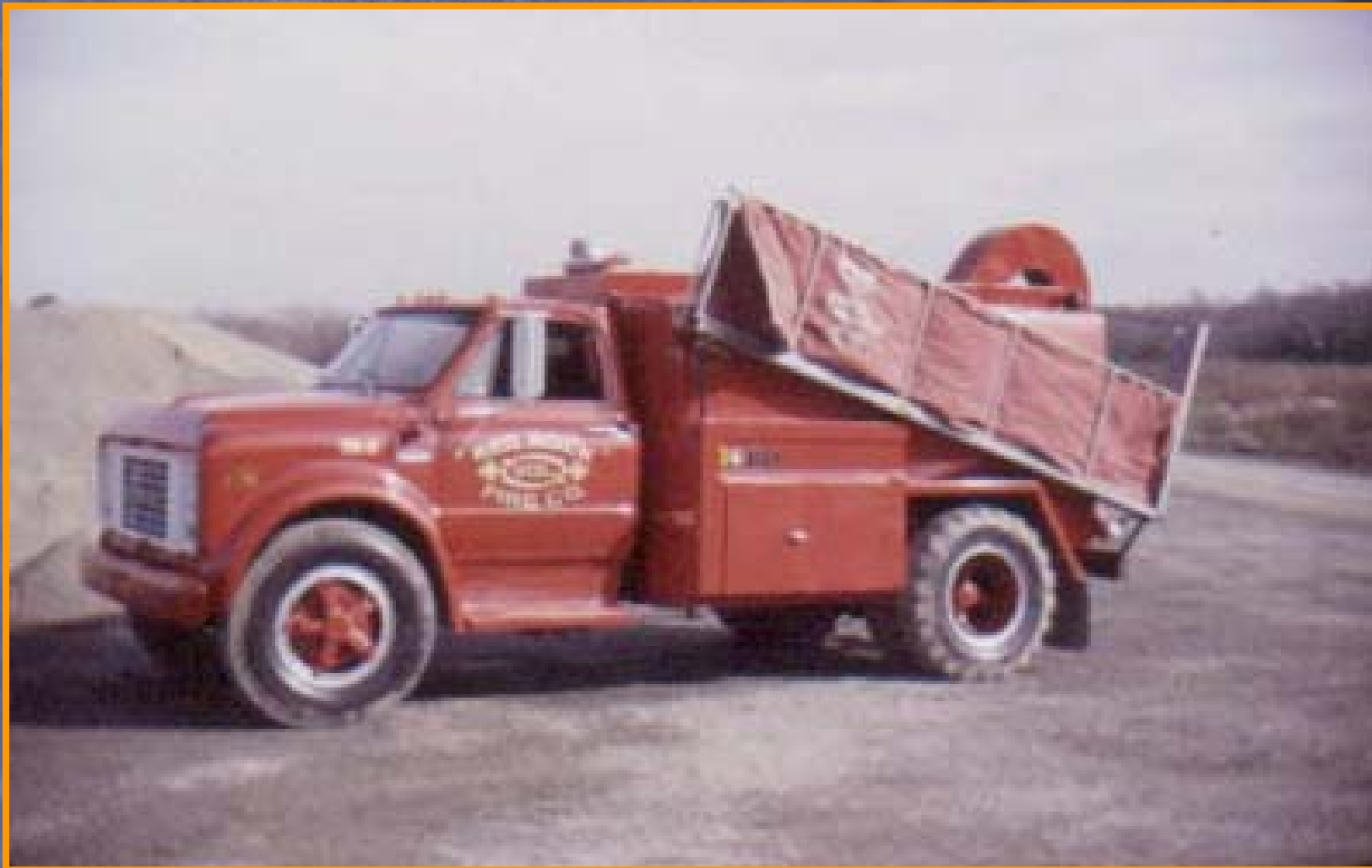
Figure 6. Both efficient and inexpensive, this 1220-gal tanker from Red Rock VFD (NY) has a 12" dump valve that can off-load 70% of its water in the first 30 seconds. This used oil truck was modified to safely carry water. The unique porta-tank rack allows the tank to slide off, minimizing the time and personnel required to set it up.
