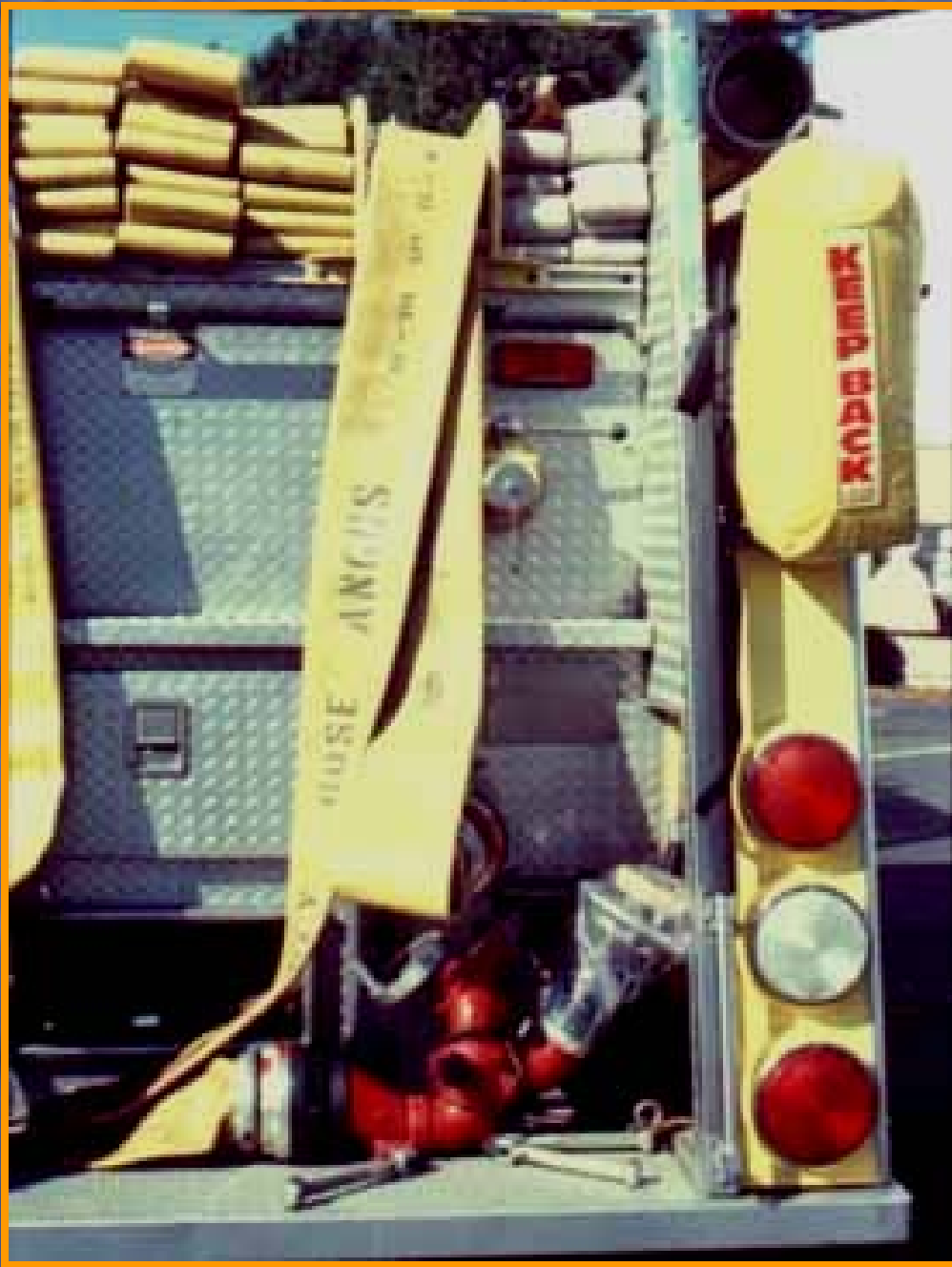
Figure 9. This Colchester (CT) attack pumper carries a preconnected master stream where it needs to be—on the tailboard. Supplied by 5" hose, this portable monitor can easily flow in excess of 1000 gpm. Two people can have it in operation in less than 1 minute.
