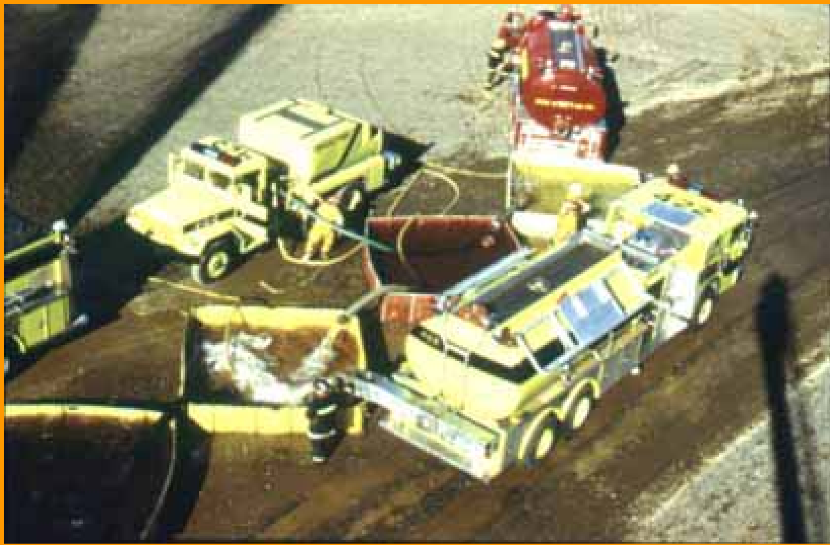
Figure 8. In a 1000-gpm tanker shuttle drill, the Nikiski (Alaska) Fire Department perfects its high-flow tanker-shuttle techniques. The drill utilizes multiple porta-tanks, 2000-gpm pumpers, and 4000-gal tankers with simple, rear-dump arrangements that allow off-loading from either side or the rear using only 1 valve
