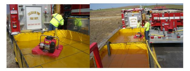
**Above:** Floating pumps can be used to move water from rectangular dump tanks behind a pumper to the drafting dump tank in front of the pumper as part of the single lane water supply set up. Tankers can travel in the other lane. Side dumps make it possible for a tanker to dump in any of four dump tanks in one pass.
