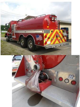
Above: (Left) Easy access to suction hose is one of the convenient features of vacuum tankers. (Right) Easy access to "difficult to handle" floating pump. The ease and convenience of reaching heavy equipment is important.
