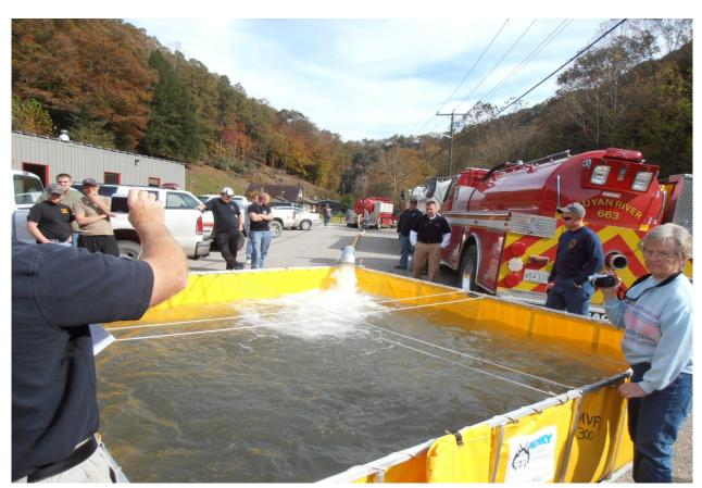
**Above:** After the tanker shuttle drill at Morrisvale West Virginia a test was conducted to determine the water movement capabilities of vacuum tankers. A 2,000 gal. vacuum tanker used only vacuum tank pressure of 15 lb. to push water at 922 GPM through 100 ft. of 5 inch LDH to a dump tank. There will likely be many more such tests to demonstrate the many capabilities of vacuum tankers.
