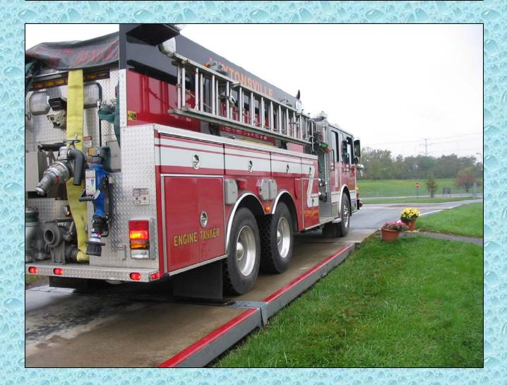
The front axle is driven off of the scale and the rear axle weights are recorded.
