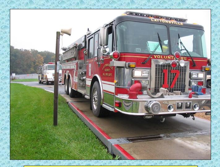
This 2000-gallon engine tanker stops with just its front axle on the scale. A weight reading is taken and the rig then pulls completely onto the scale.
