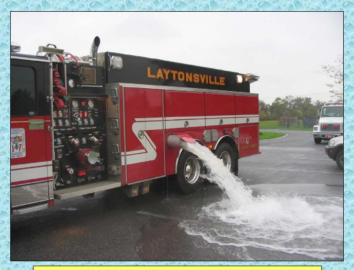
The engine tanker dumps for one-minute and then returns to the scale for a weight reading. (All axles are weighed together – there is no need to weigh the axles independently at this point.)
