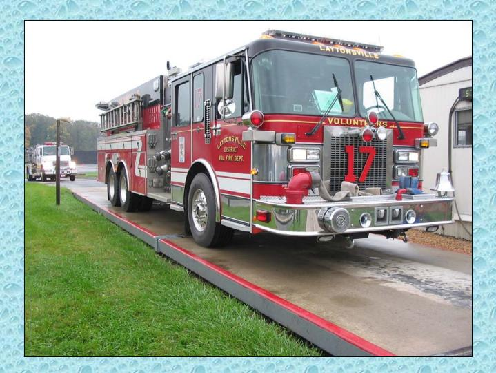
All three axles are on the scale and the weight is recorded and compared to the listed GVW.
