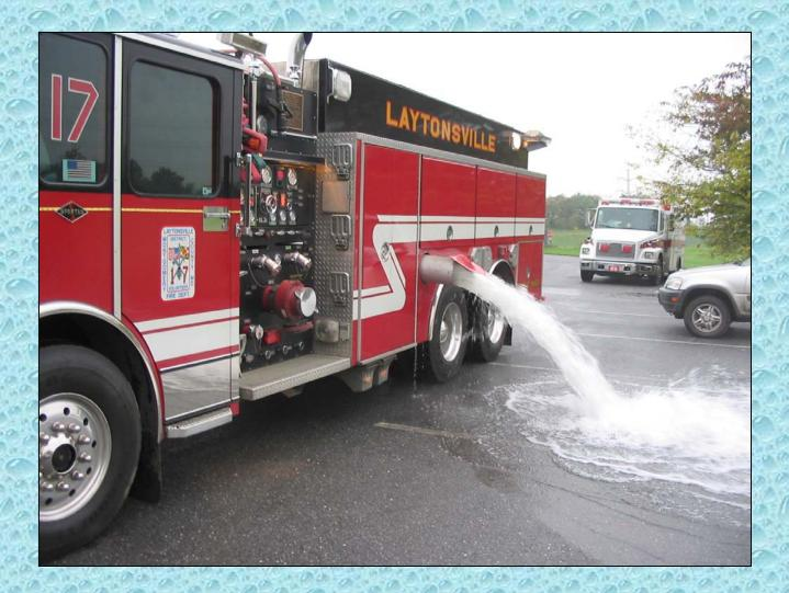
The tanker dumps for another minute and then reweighs. The critical dump time for this 2000-gallon engine tanker was calculated at 90 seconds with a total off-load of 1800 gallons.
