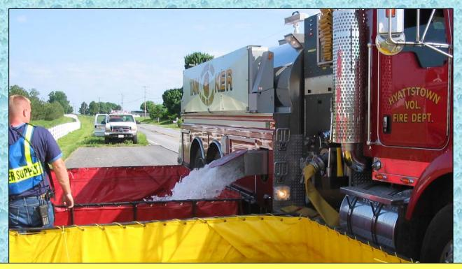
This 3,500 gallon, 4-Guys tanker has a 10-inch square dump located in front of the rear wheels. It is also equipped with remote dump valve controls in the cab of the vehicle..
