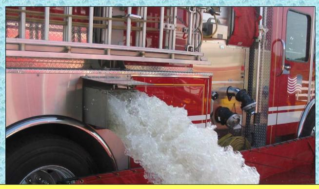
This engine tanker has a 10-inch square dump located in front of the rear wheels.
