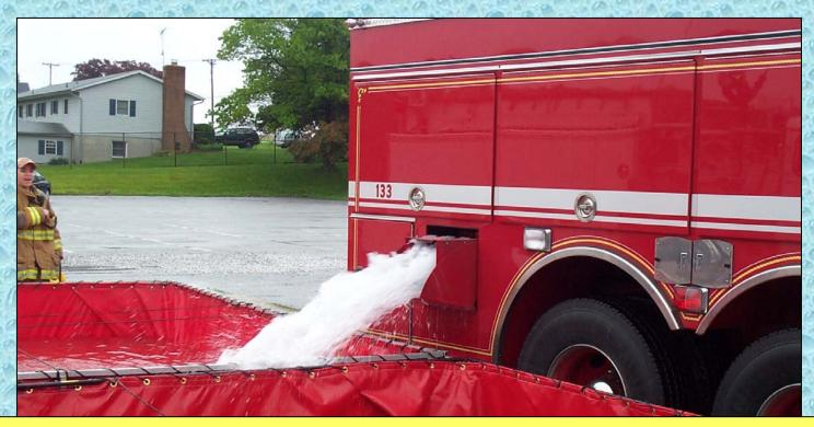
This engine tanker has a 10-inch square dump located to the rear of the rear wheels. On this rather lengthy rig, it can be a bit tricky to align the chute with the dump tank.
