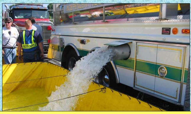
This 3000-gallon elliptical tanker has a 10-inch round dump located in front of the rear wheels allowing for easy alignment with dump tanks.
