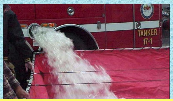
This 3500 gallon elliptical tanker has an 8-inch round dump located in the teardrop section of each rear wheel well. It also does not have any kind of extending tube which results in the driver having to maneuver the rig very close to the dump tank.
