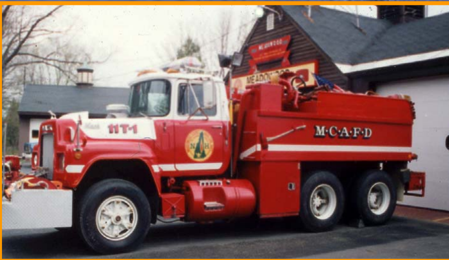
Figure 2. Although these vehicles vary greatly in design, they all share one thing in common: Departments designed them to haul water to fires to supply rural fire-attack operations. From the first time fire departments used tank vehicles to haul water to fires, these vehicles have been called tankers .
