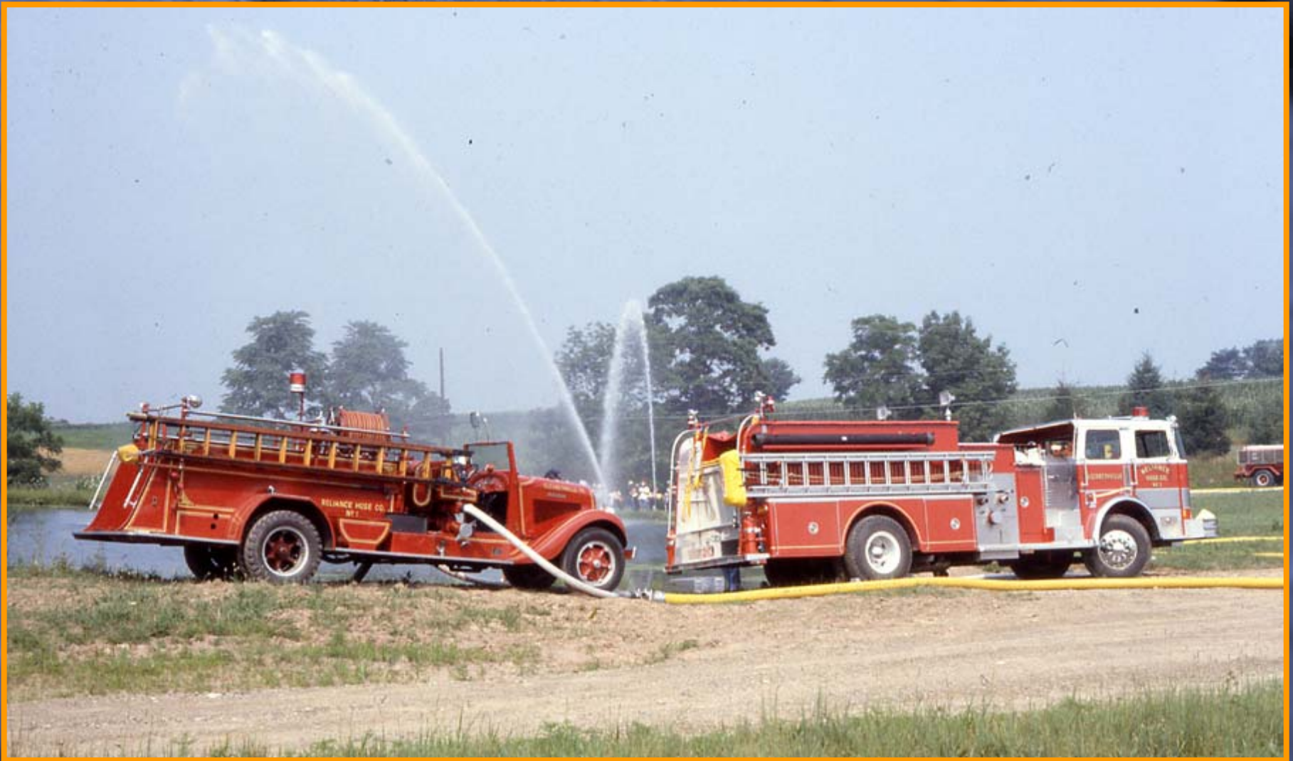
Figure 1. The stream from the 1-1/2" tip on the left supplied by the 40-year-old 500-gpm pumper is much better than the stream from the 1-1/2" tip on the right, which is supplied by the new 1500-gpm pumper.
