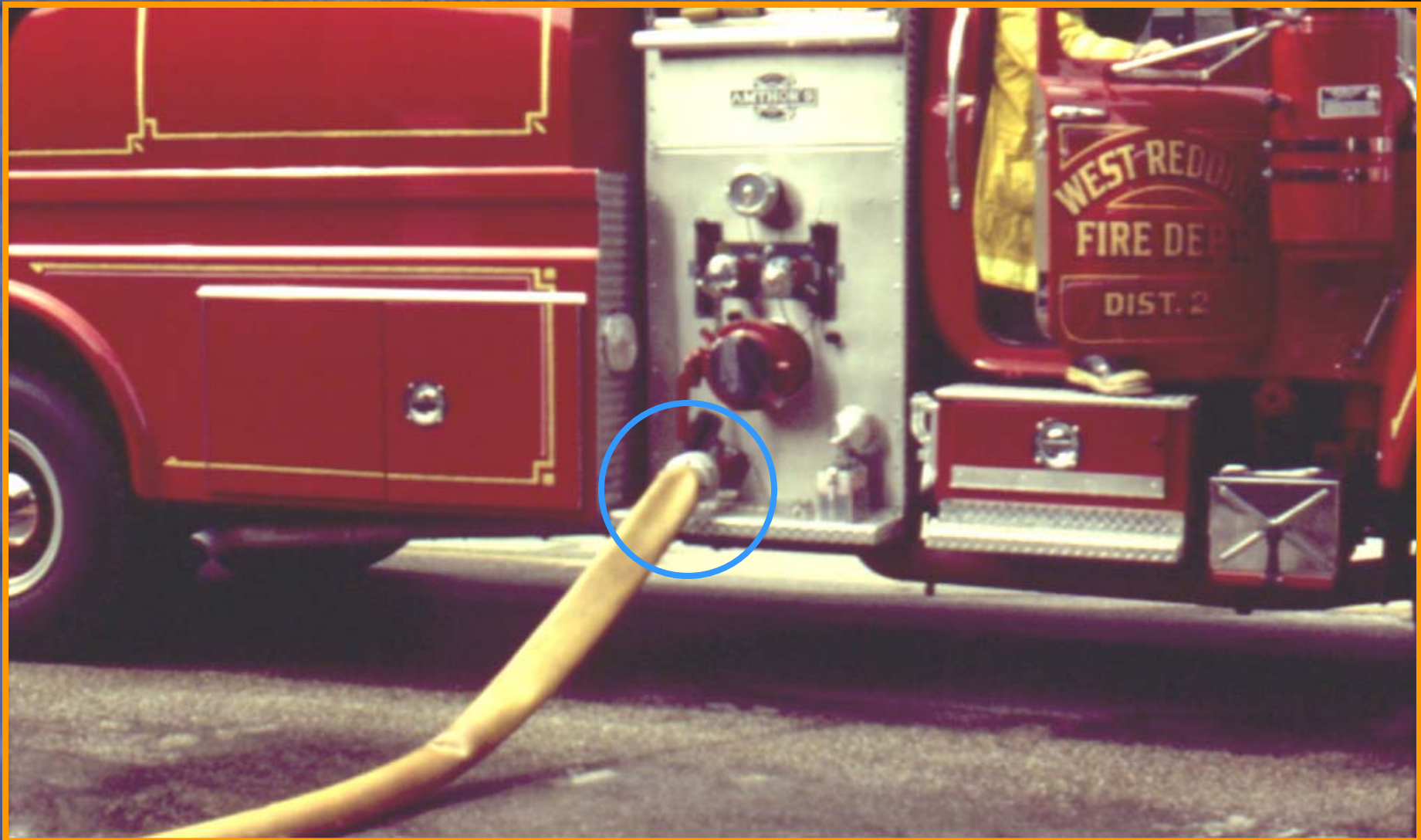
Figure 7. This pumper's 6" intake is equipped with a butterfly valve to facilitate drafting. However, due to the lack of an LDH Storz adapter for the butterfly valve, this LDH supply line had to be run into the 2-1/2" auxiliary intake. This significantly reduced the flow from the LDH into the pump.
