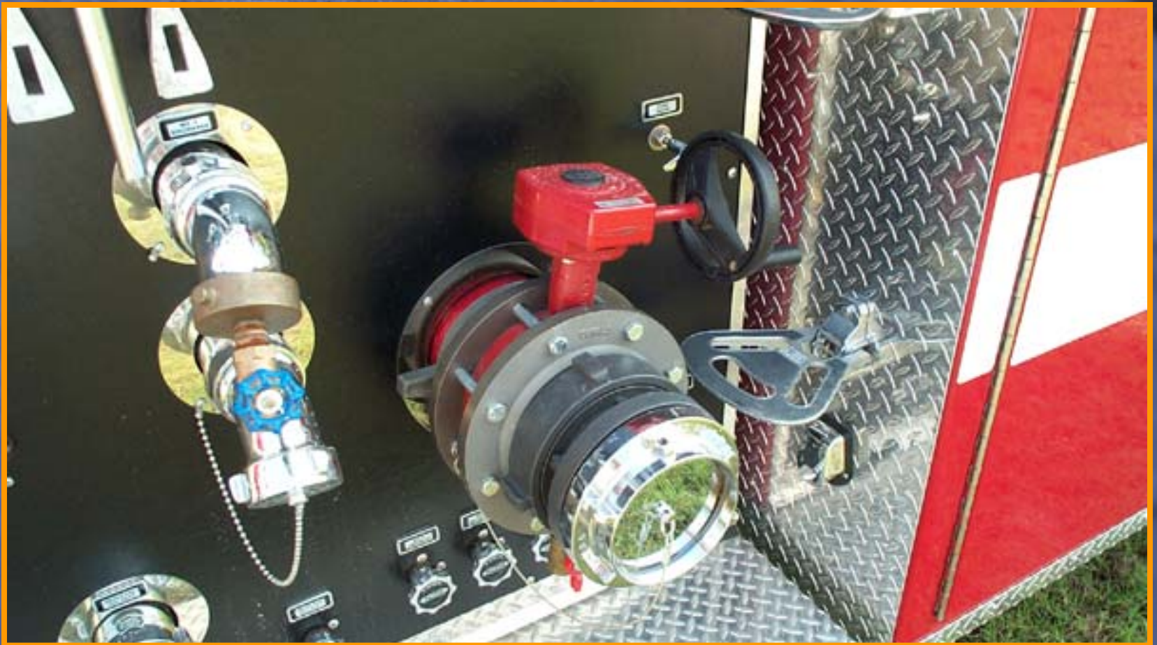
Figure 8. This intake is primarily used for drafting from a porta-tank. It is equipped with a gear-operated slow-opening valve. Just in case the pumper must be supplied by a 5" LDH line, the department did a very smart thing. The valve has a 6" NST threaded connection on the outboard end. A 6" NST female x 5" Storz adapter with a 5" Storz blind cap finishes off the valve. When a 5" supply line is to be used, the Storz cap is removed. When the pumper must draft, the Storz adapter is removed. The cost of the 6" x 5" Storz adapter is small and provides versatility to this intake.
