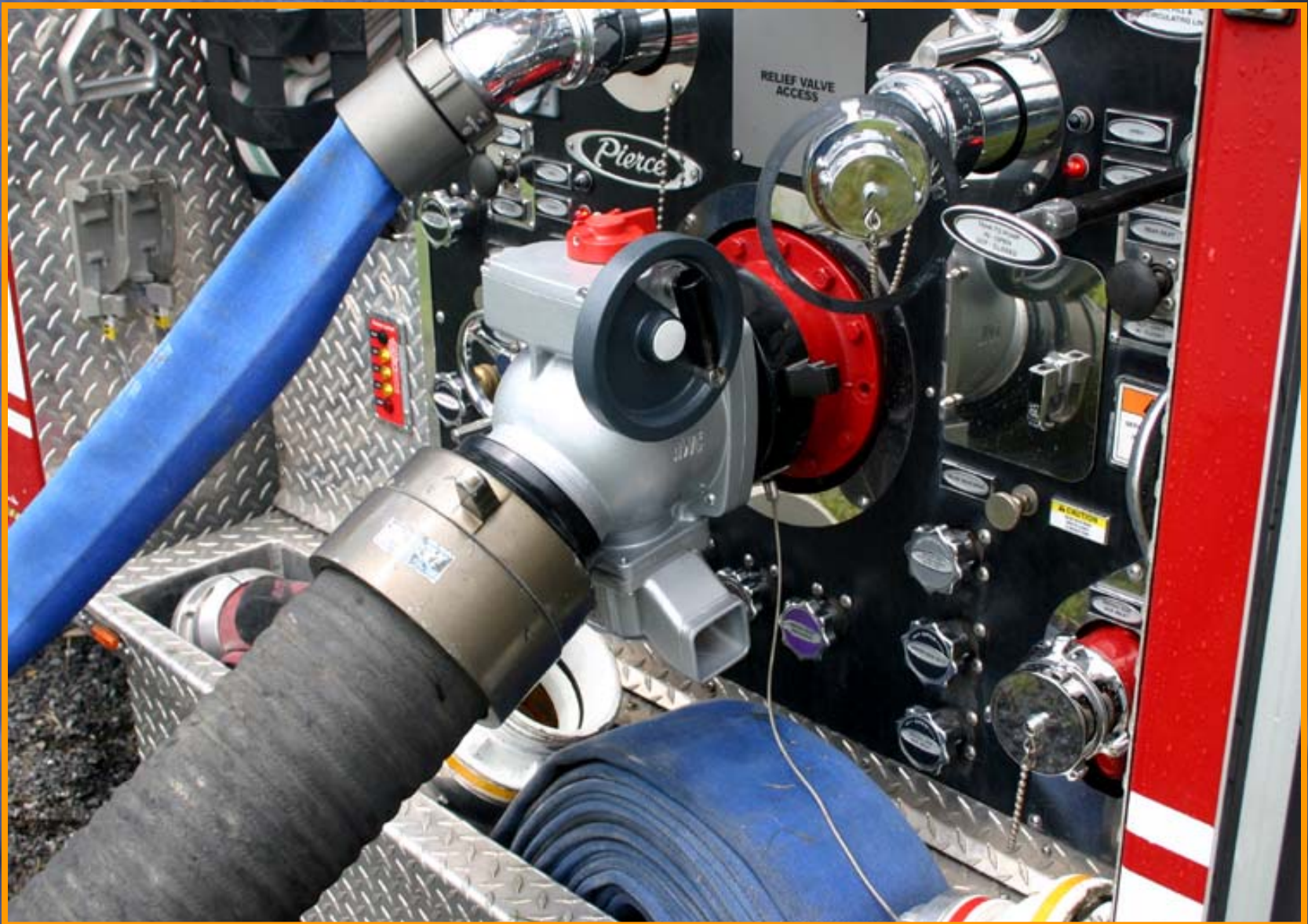
Figure 11. This pumper is equipped with a Kochek gear-operated ball intake valve equipped with both an air release and pressure relief valve.
