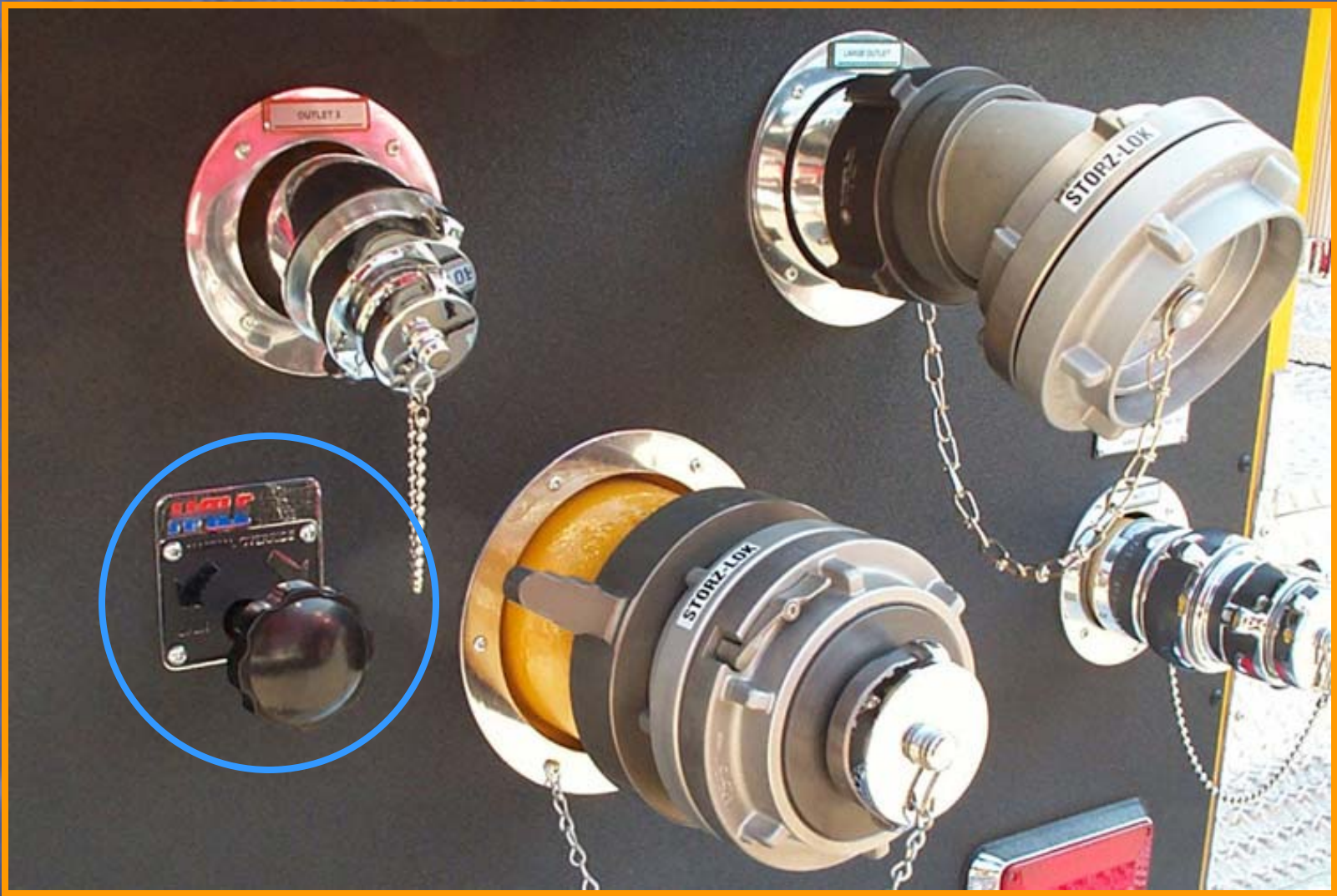
Figure 9. This intake is equipped with a Hale MIV (master intake valve). While the control can be remote or at the valve, the control for this valve is the black knob to the left of the valve.
