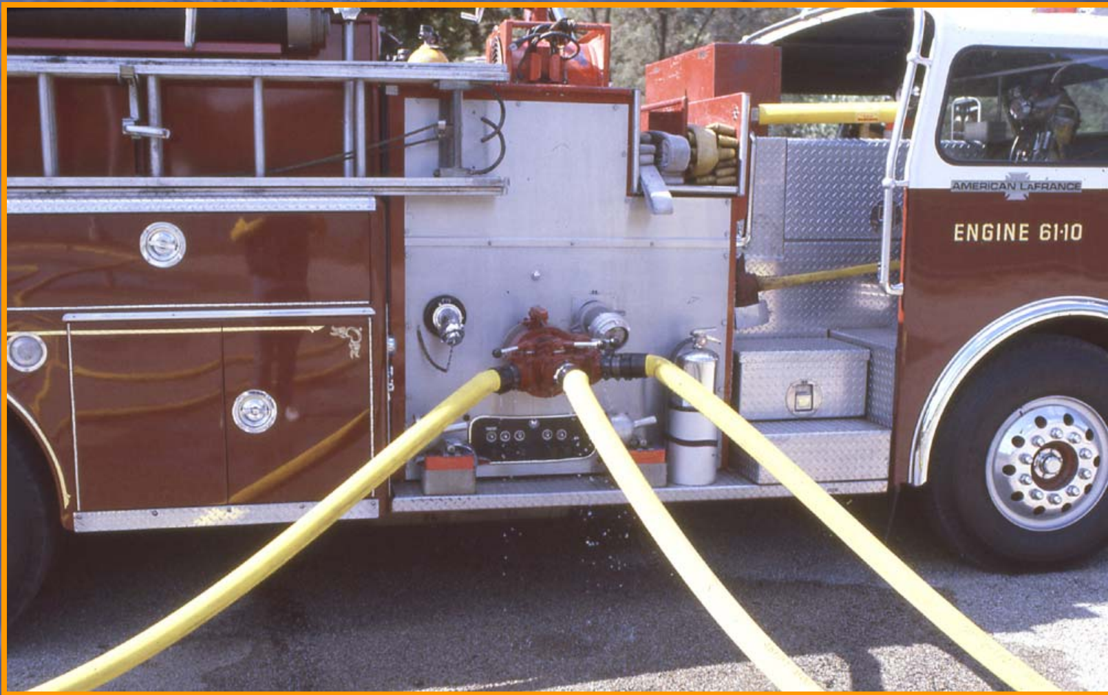
Figure 3. If the purpose of having auxiliary intakes is to maximize pump output, a 2- or 3-inlet siamese into the large pump intake is much more efficient than auxiliary small intakes. In specifying apparatus, eliminate the auxiliary intakes required by NFPA 1901 and specify a siamese. This will maximize flow from the intake lines.
