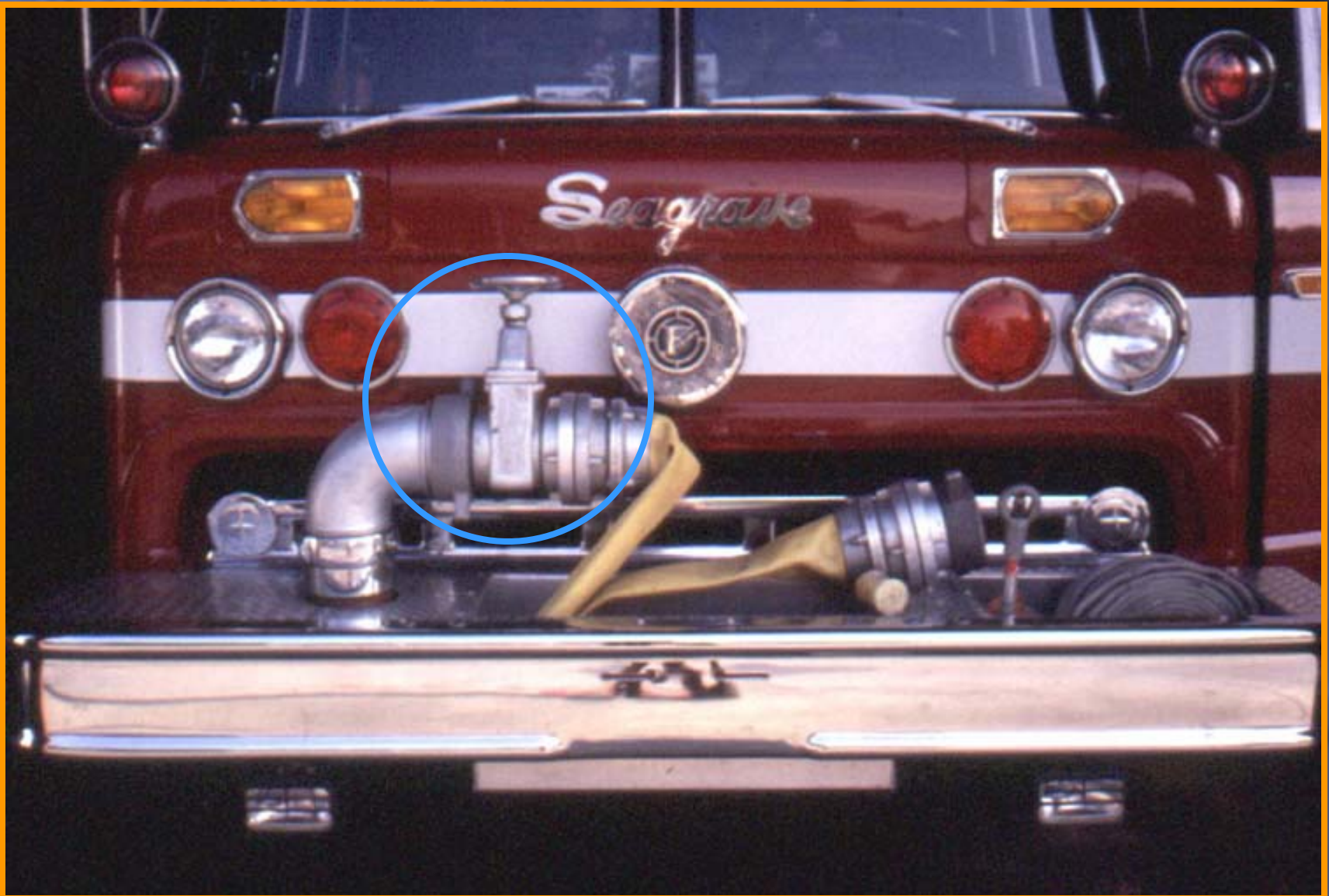
Figure 10. This department valved this engine's front suction by using a Jaffrey gate valve.
