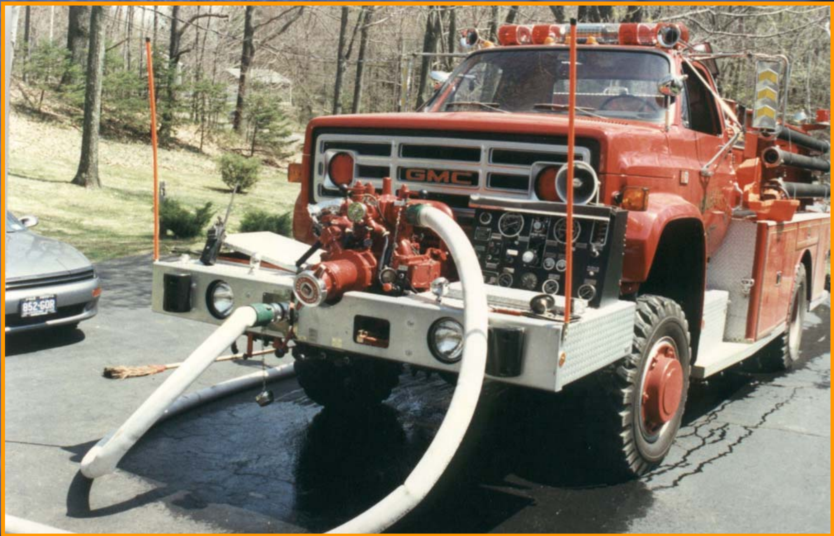
Figure 1. Historically, the only intakes that were valved were the 2-1/2" (or 3") auxiliary intake valves. This attack pumper is being supplied by a 3" line from a nurse tanker.
