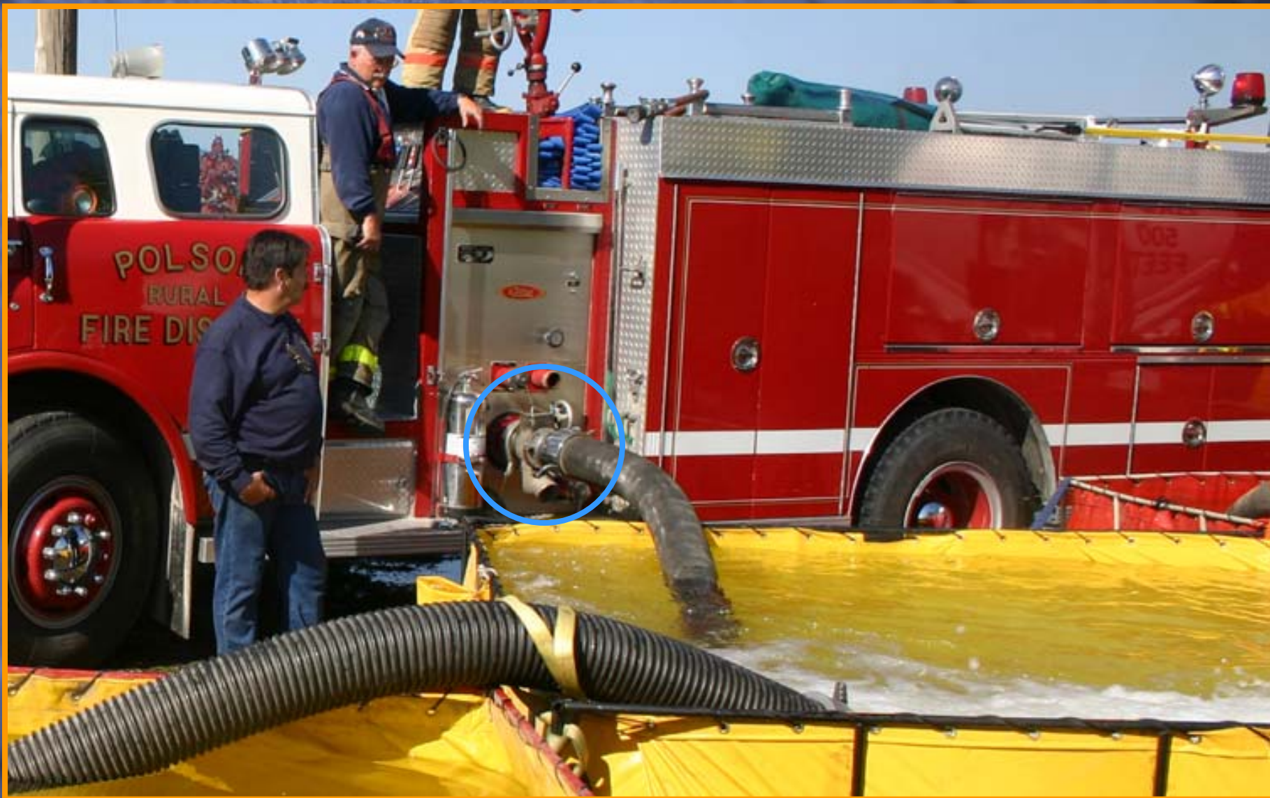
Figure 5. To set up this porta-tank drafting operation using the pumper's 5" Storz-connected intake valve, a 5" Storz x 6" male NST adapter had to be used.
