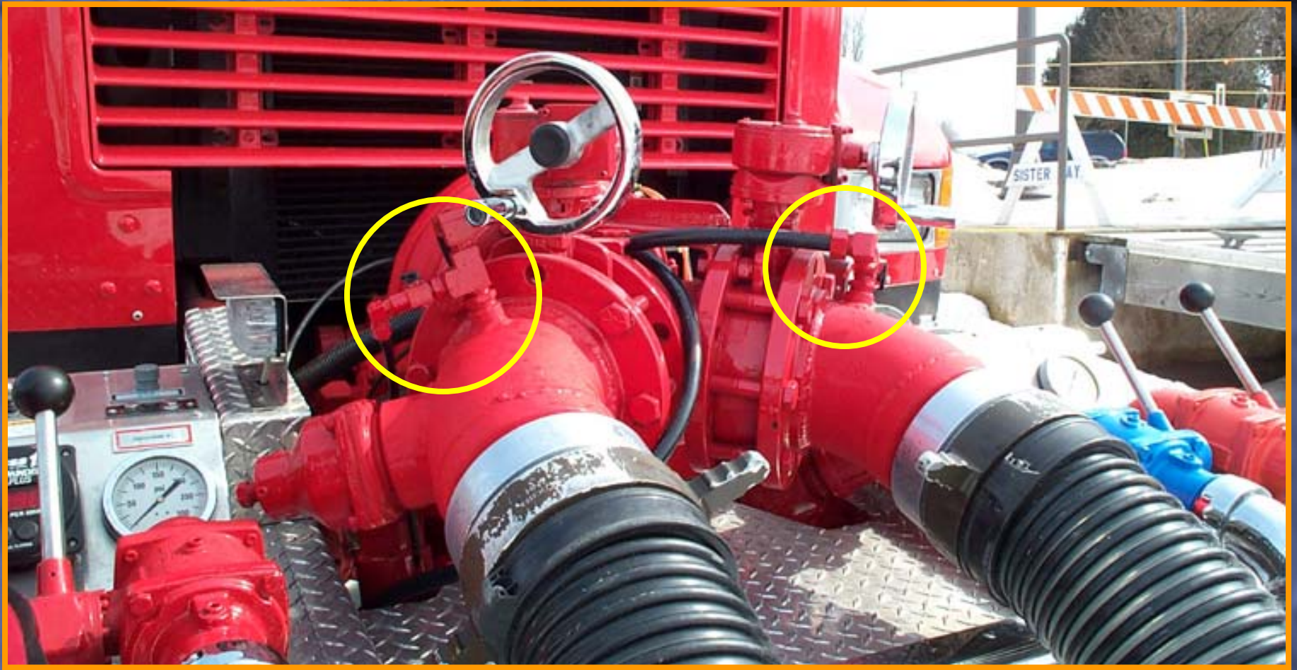
Figure 12. This 1250-gpm front mount pump of Sister Bay (WI) is equipped with dual suctions equipped with gear-operated butterfly valves and pre-primers. The black hoses extending to the suction hose side of the valves are separate priming lines to allow the suction hose to be primed up to the pump. This allows the second suction to be connected and primed after the first suction and pump have been primed without losing water.
