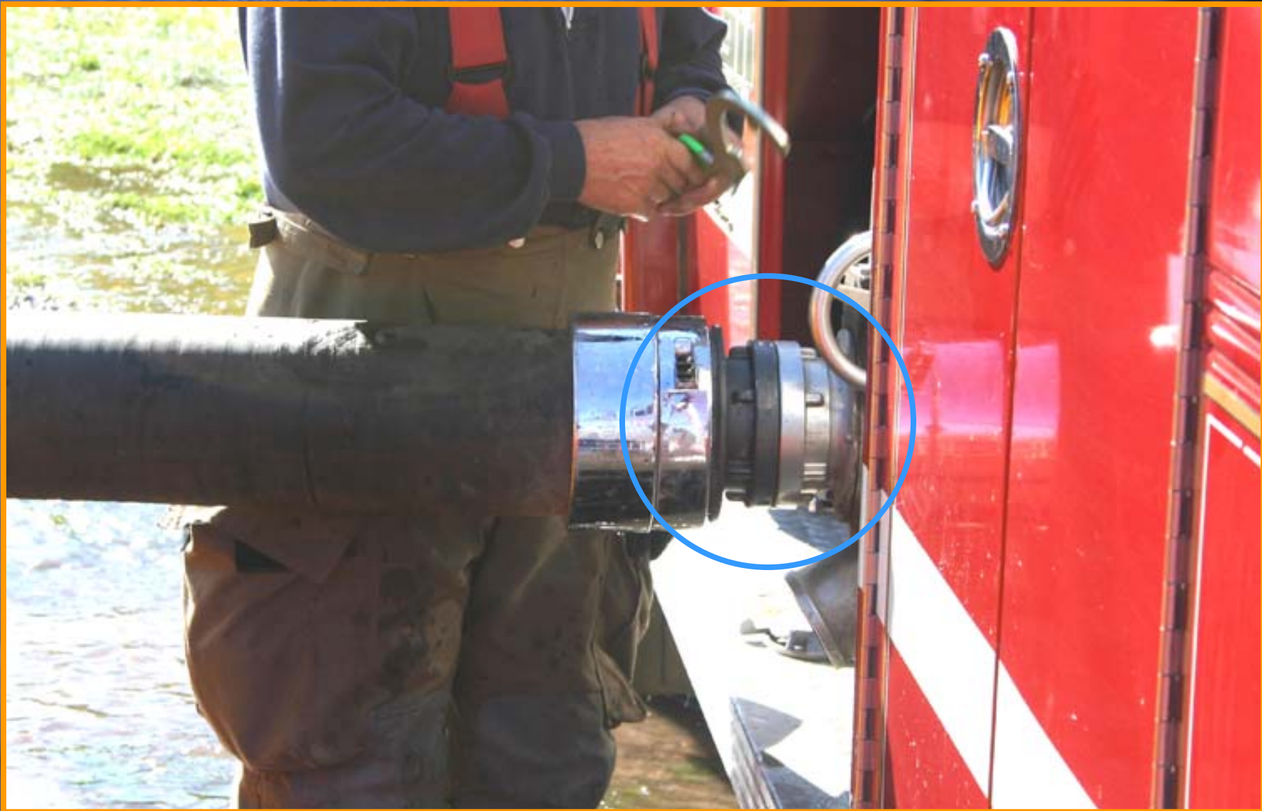
Figure 6. The simple addition of the 5" Storx x 6" NST adapter can reduce the delivery rate from draft by 200-300 gpm.
