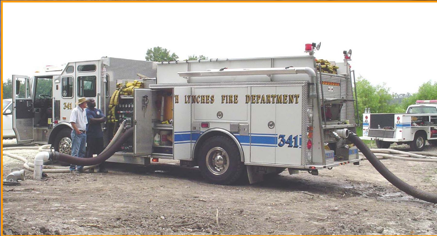
Figure 15. A South Lynches engine drafts from both a dry hydrant using 10 ft of 6" suction, and the static water source using its rear suction with its squirrel tail suction with barrel strainer and float to deliver 2250 gpm with a 1500-gpm pumper — a 50% increase in delivery.
