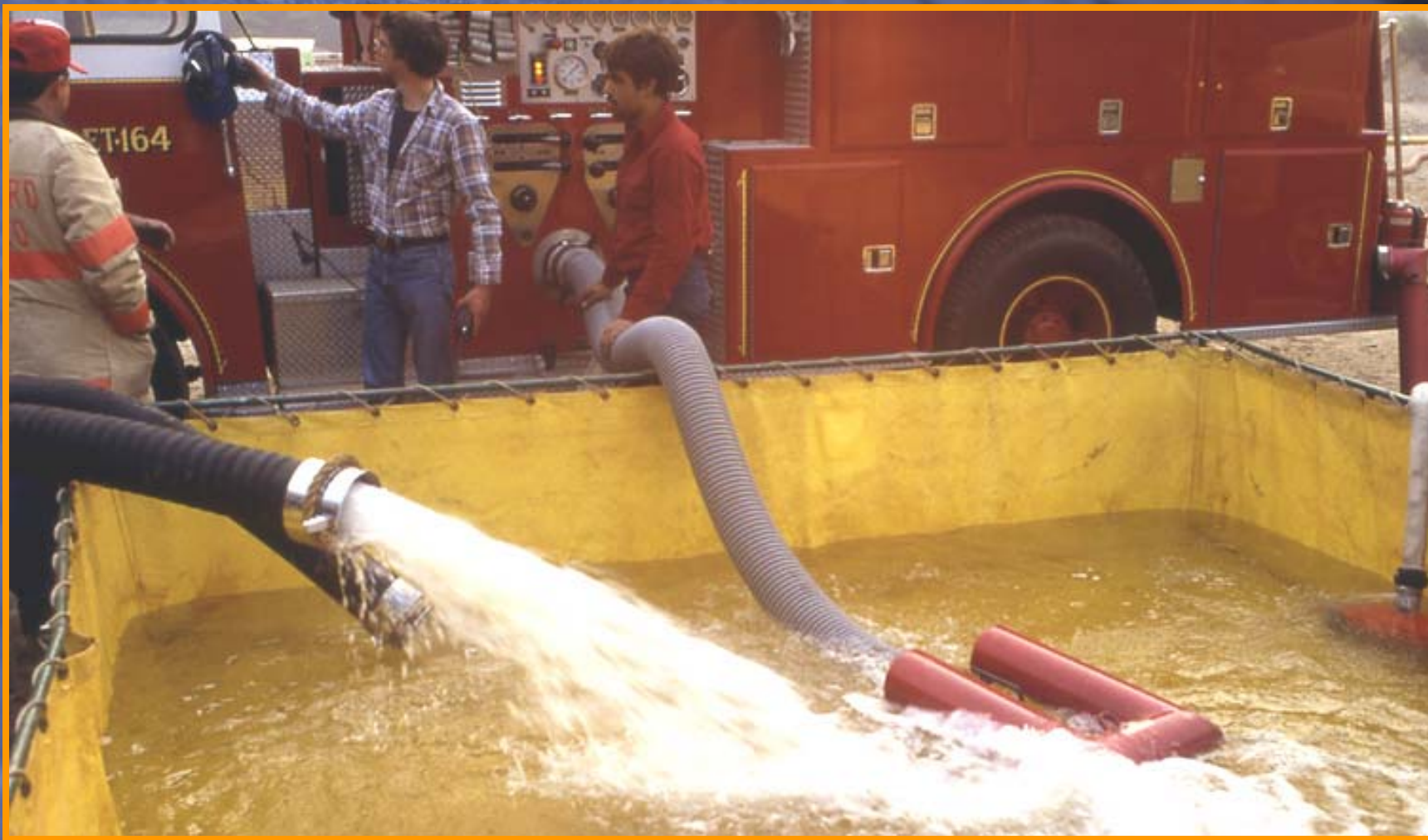
Figure 9. While some departments use floating strainers in porta-tank operations, this type of strainer can't draw the water down as low as a low-level strainer. In addition, since water enters the strainer from the bottom, if the water level drops too low, atmospheric pressure can force the fabric of the porta-tank to clog the holes in the strainer and actually stop the flow.
