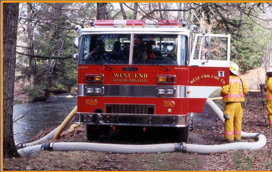
Figure 1. This 1250-gpm pumper is drafting from a shallow stream using dual suctions. The key to its being able to deliver over 1800 gpm was not only the dual suction lines but also the use of the strainers (as shown in Figure 2) designed for the specific drafting situation.
