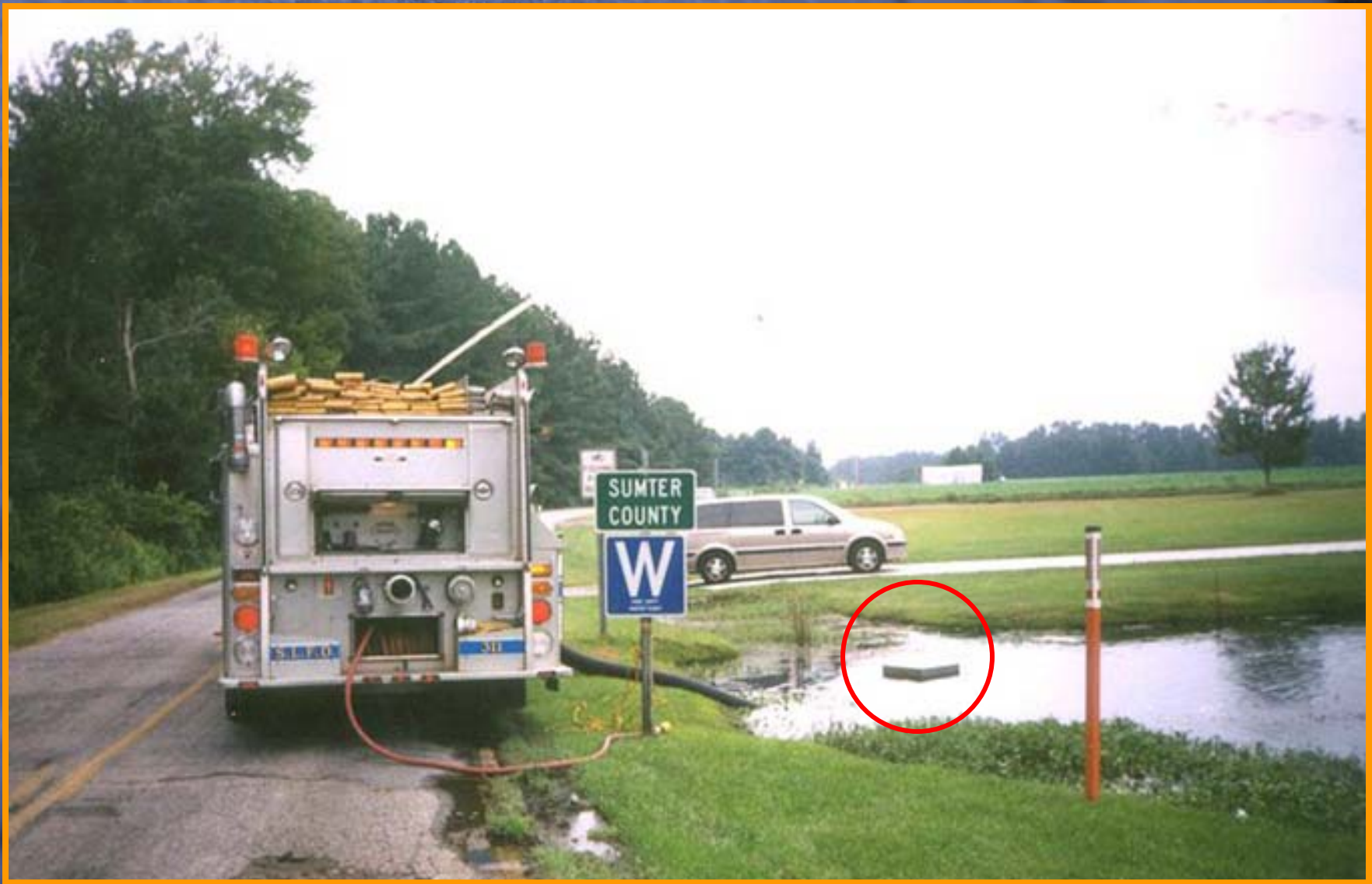
Figure 14. A South Lynches engine drafts from a water source to fill tankers. The suction strainer float (red circle) can be seen in operation.
