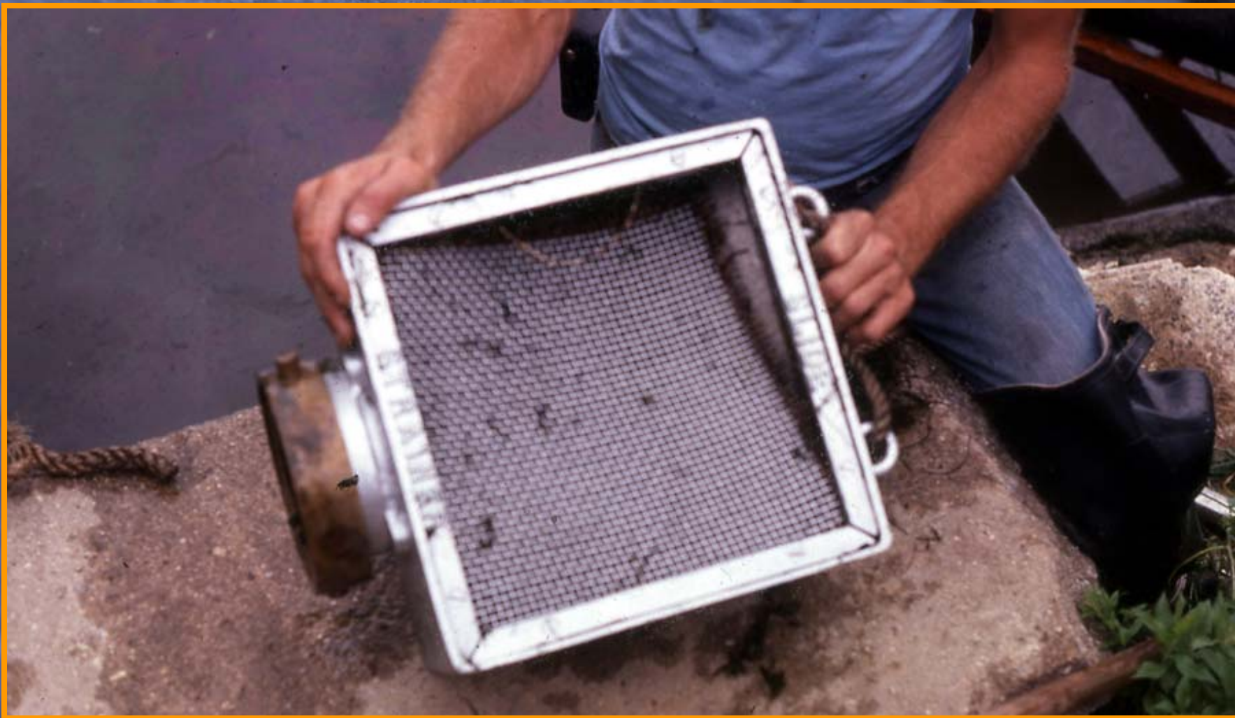
Figure 8. Most people don't have an appreciation for the force of atmospheric pressure on a strainer connected to a suction line that has been primed. This box strainer collapsed, breaking the welds, when surface vegetation in a New England pond clogged the openings in the strainer.
