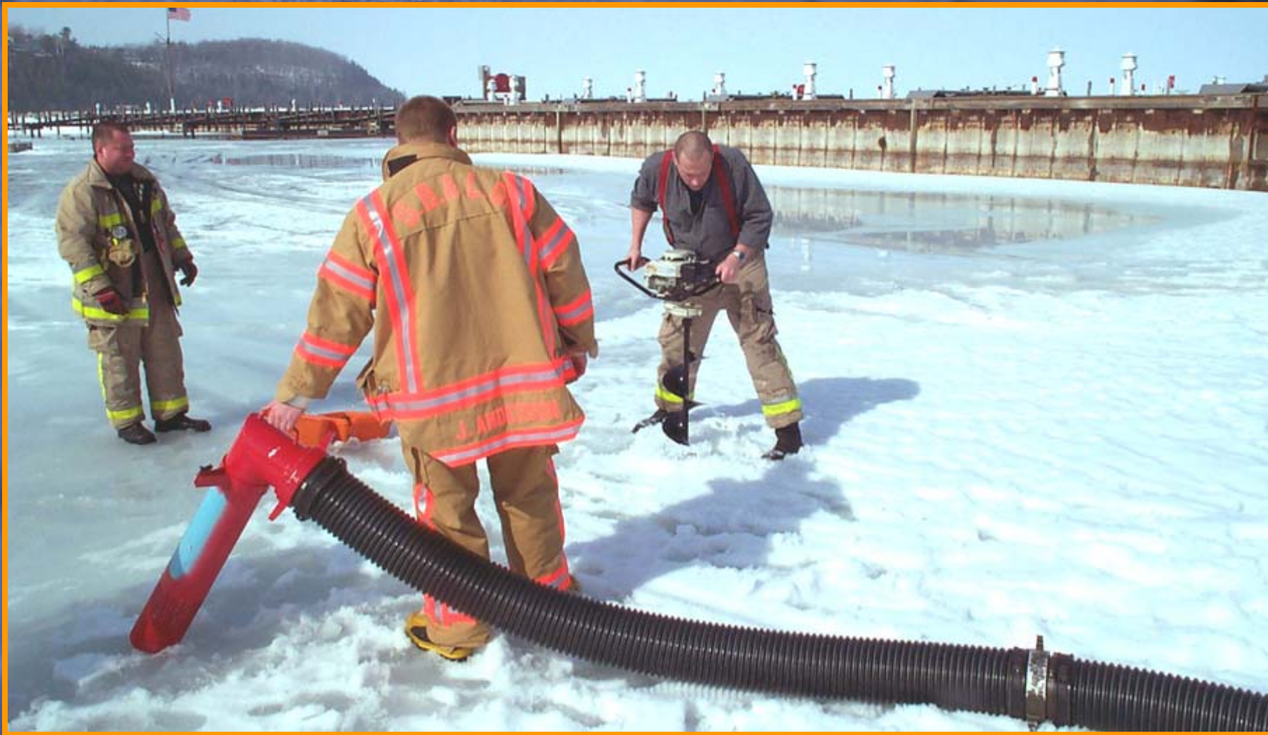
Figure 11. A Kochek ice strainer used in conjunction with a powered auger to access lake water. While a barrel or acorn strainer could be used in the same operation, the ice strainer's design simplifies the set up, requires less suction hose and eliminates the need to bend suction hose at a right angle.
