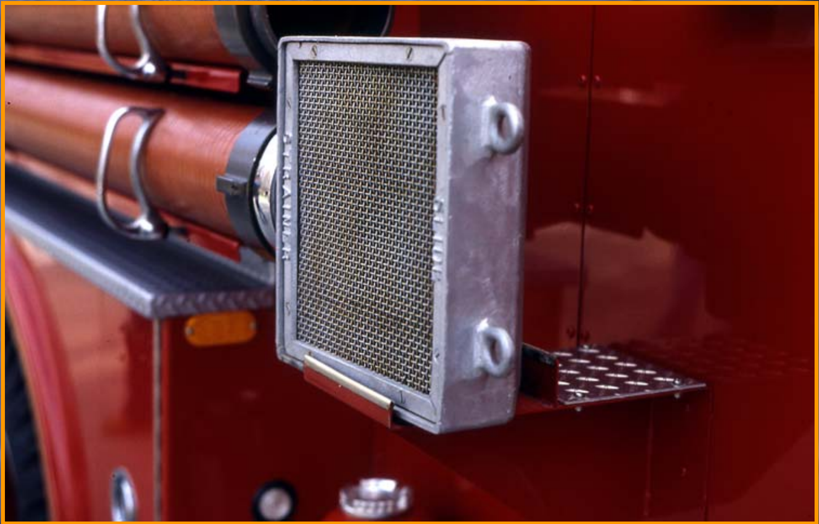
Figure 6. Another traditional suction strainer, especially common in the Northeast, is the box strainer. This strainer was designed to sit on the bottom of a water source and draft water from the top.
