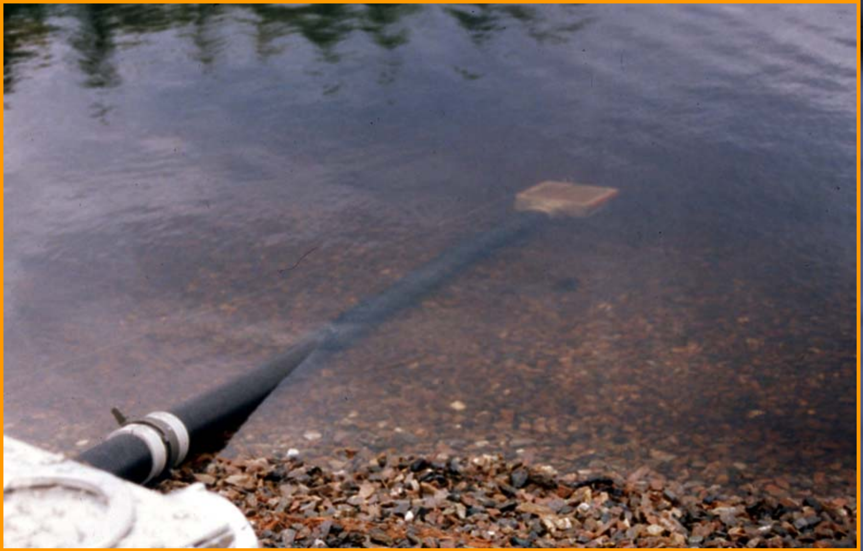
Figure 7. This is a perfect application for the box strainer — strainer lays on bottom and drafts from top in water deep enough so no whirlpool develops.
