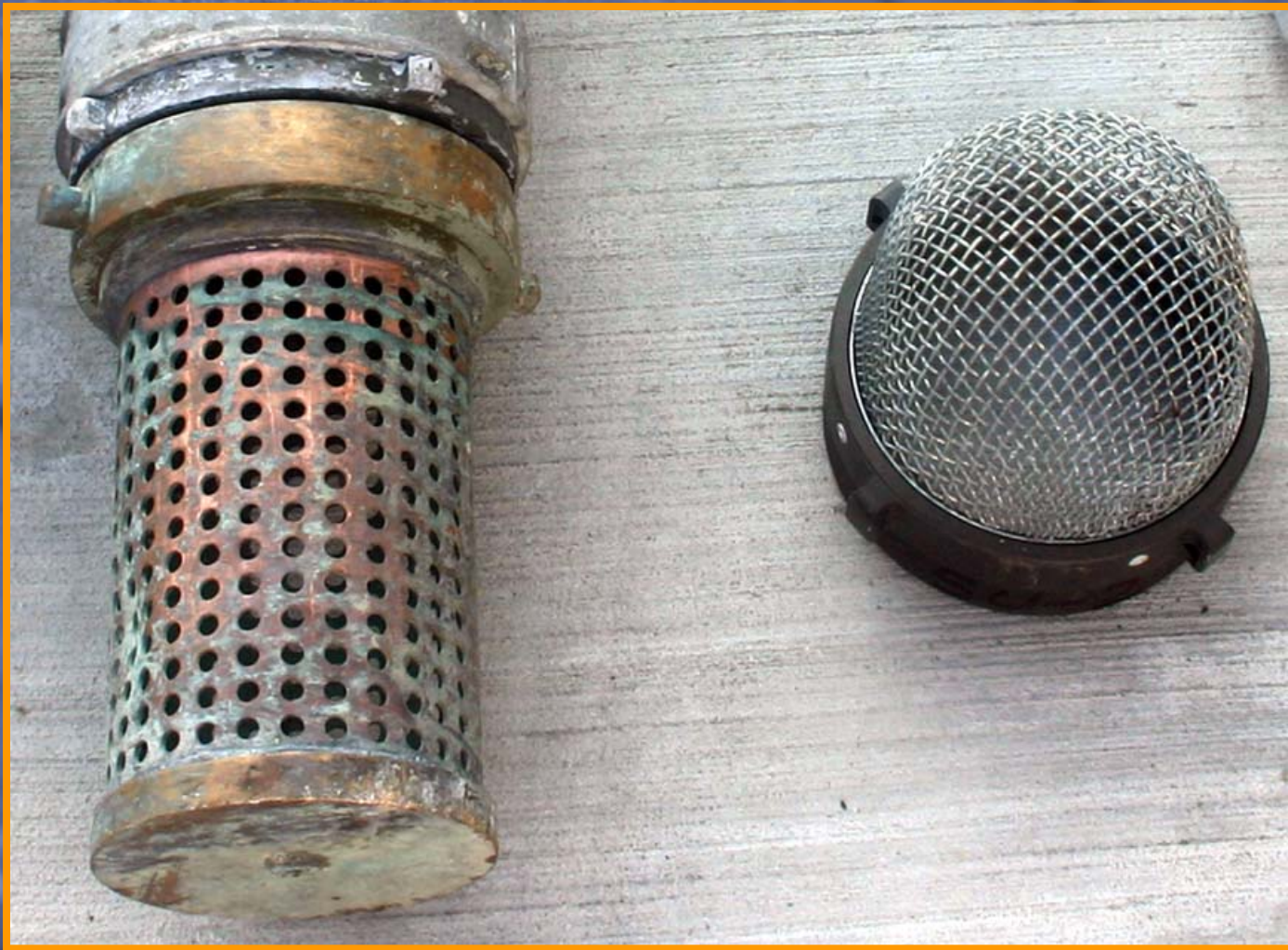
Figure 3. Both the barrel strainer on the left and an the acorn strainer on the right perform well as long as the water sources are deep enough so air is not drawn into them and they do not sit on the bottom where they can draw in debris and become clogged.
