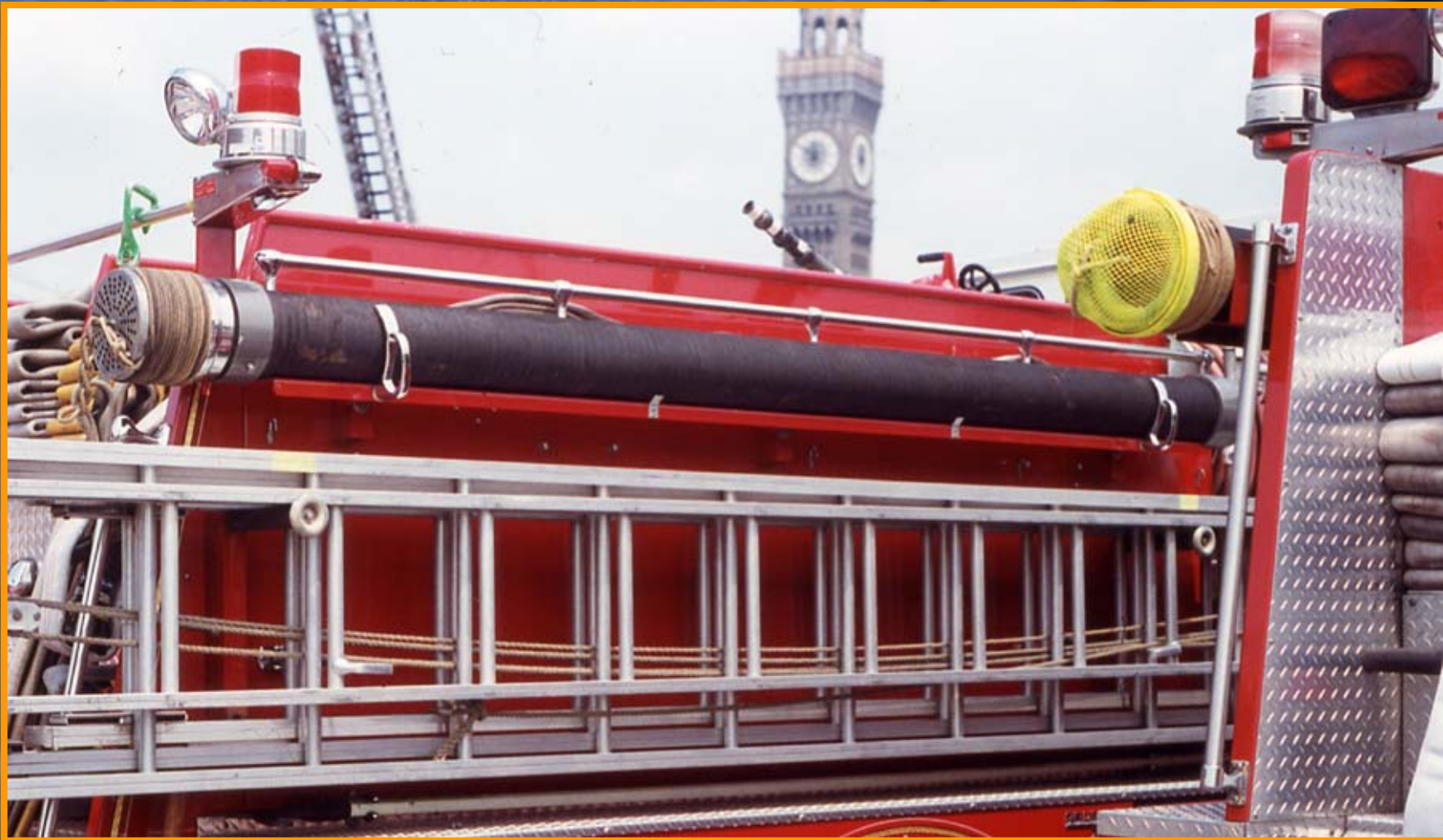
Figure 5. Many departments carry their suction strainers neatly tucked into compartments. Those who are serious about drafting generally carry suction strainers pre-connected. A key component of any barrel or acorn strainer is the rope attached to it to help in positioning and retrieving the strainer.
