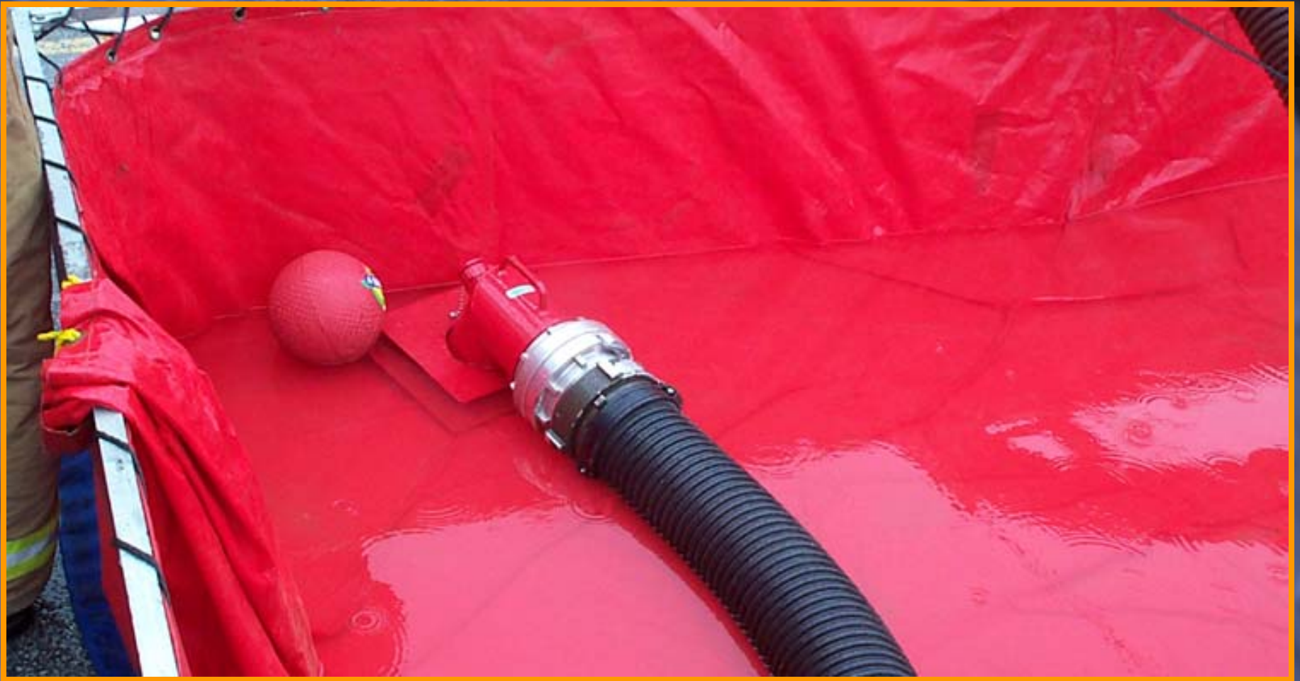
Figure 10. Low-level strainers were invented by rural firefighters who had to draft from porta-tanks in water shuttle operations. Because of the design of the low-level strainer, water can be drawn down to within a couple of inches of the bottom of the porta-tank. The ball also plays a vital role in porta-tank drafting operations. As the water level drops to the point where a whirlpool develops, the ball sits in the whirlpool to keep air from entering the strainer and prime to be lost.
