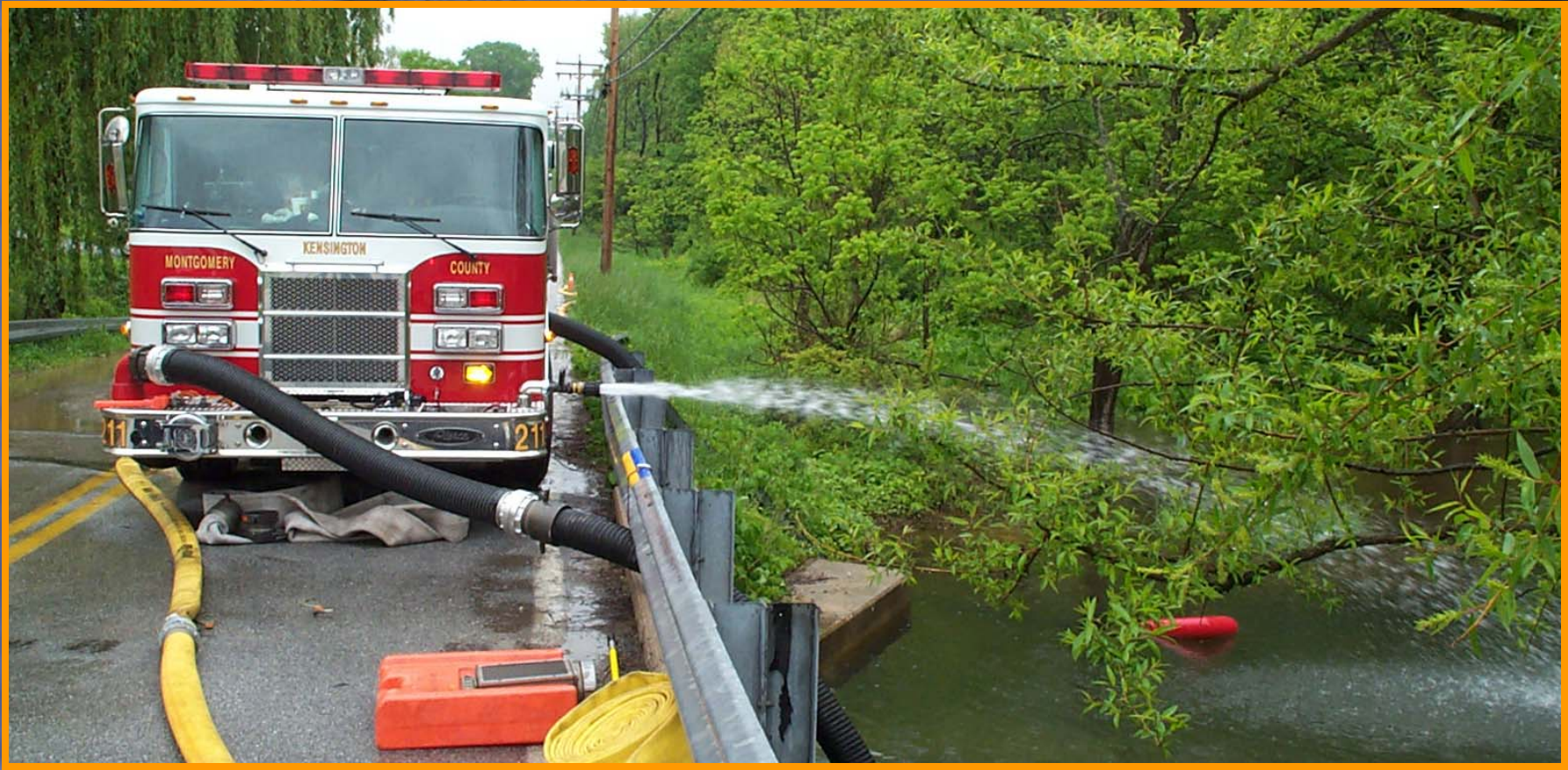
Figure 1. To get the highest flow for a tanker fill operation, a front suction must be supplemented with a side suction. If a side intake valve is not provided, the side suction must be connected first to get the operation working. Once the side suction is operating, the valved front suction can then be used. A good driver/operator can then prime the front suction by opening the suction valve ever so slowly without ever having to hit the primer.
