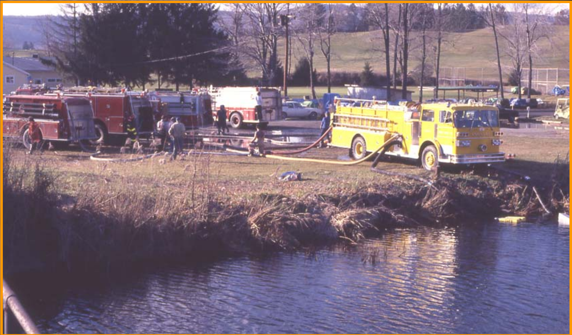
Figure 8. An overview of the fill site. With the pumper using dual suctions, it delivered between 1500 and 2000 gpm, and reduced tanker fill time significantly.
