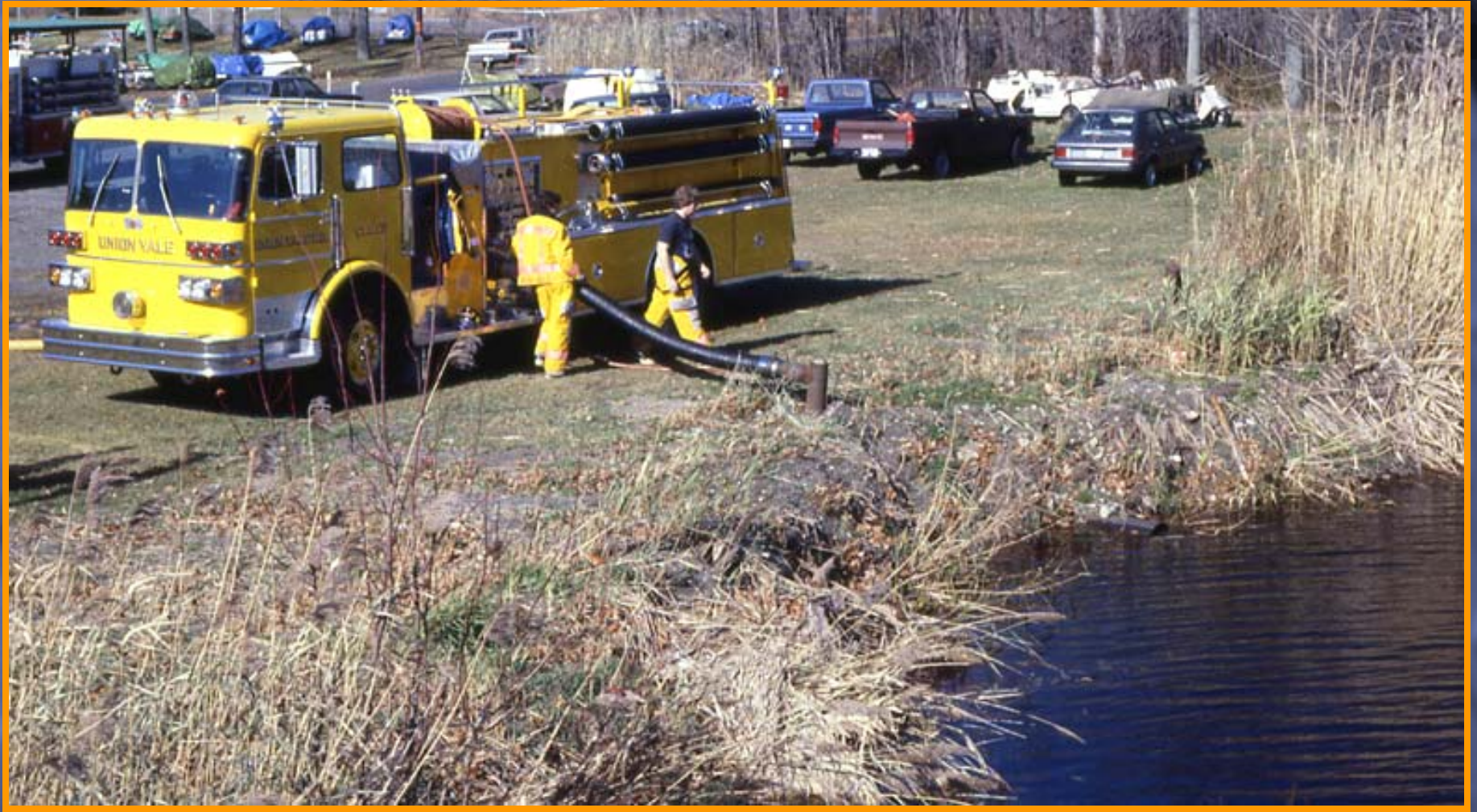
Figure 6. The 1000-gpm pumper originally hooked up with a 10-ft length of 6" suction to the dry hydrant. While this was convenient, much of the pump's energy was going to be lost due to friction loss in the dry hydrant piping. This would result in a tanker fill rate much less than it could be.
