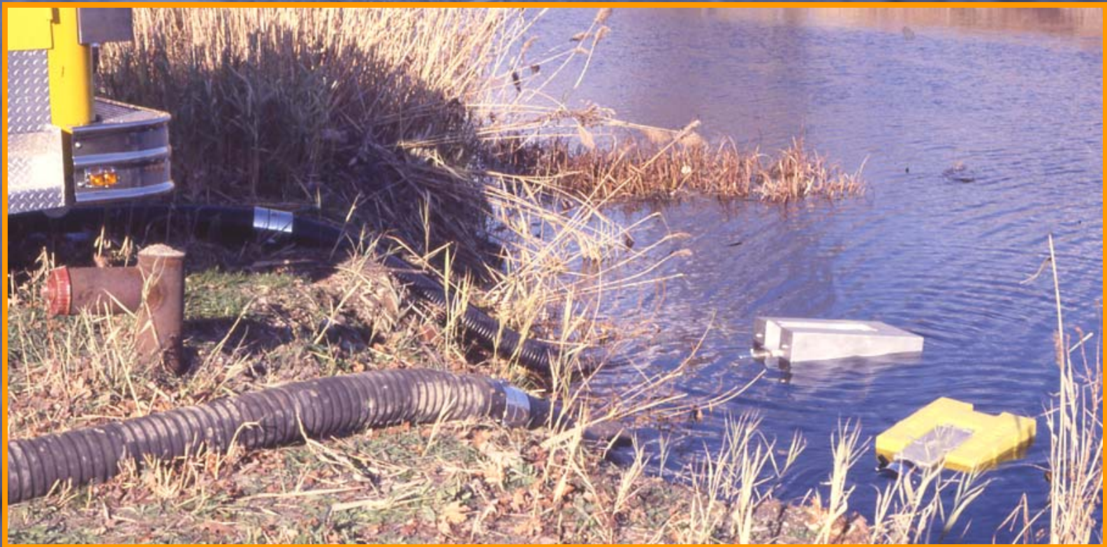
Figure 7. The pumper was nosed up to the water source with dual 6" suctions equipped with floating strainers used to minimize losses and maximize the delivery rate.
