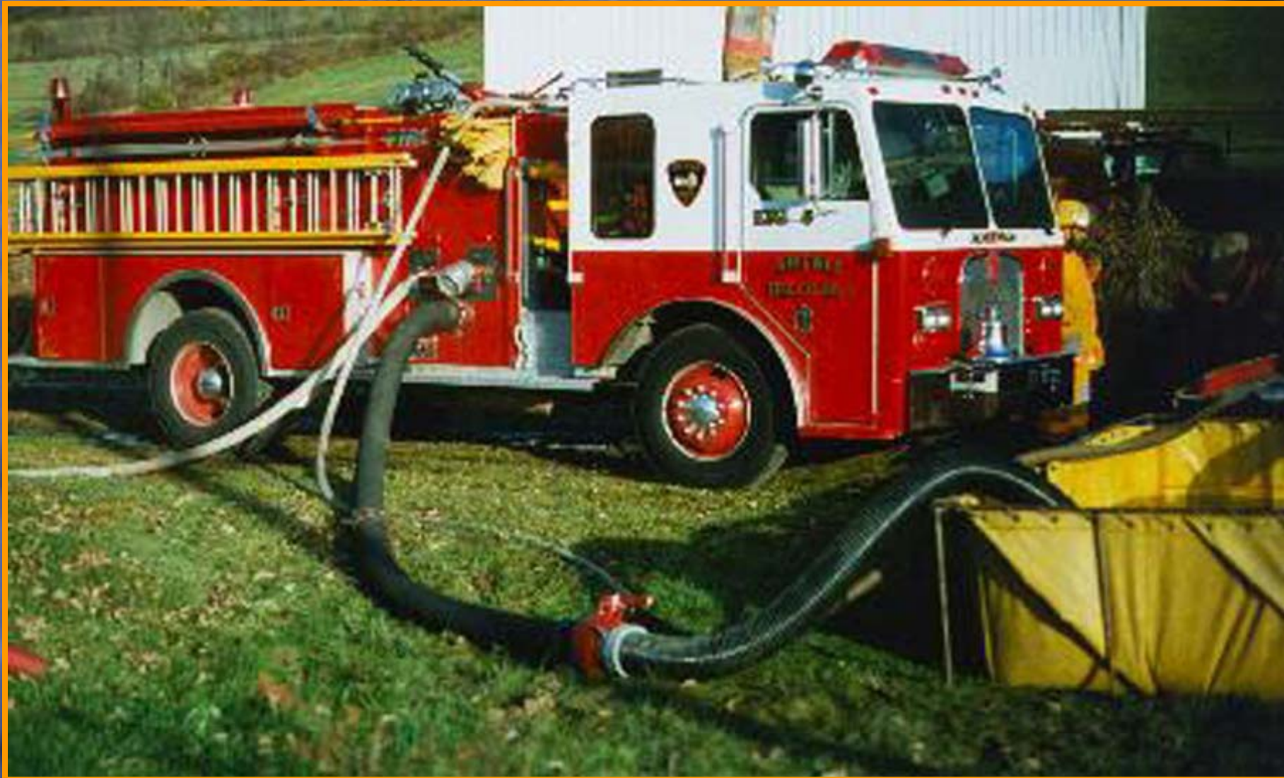
Figure 10. How to use a side suction to draft from the front of an apparatus.
