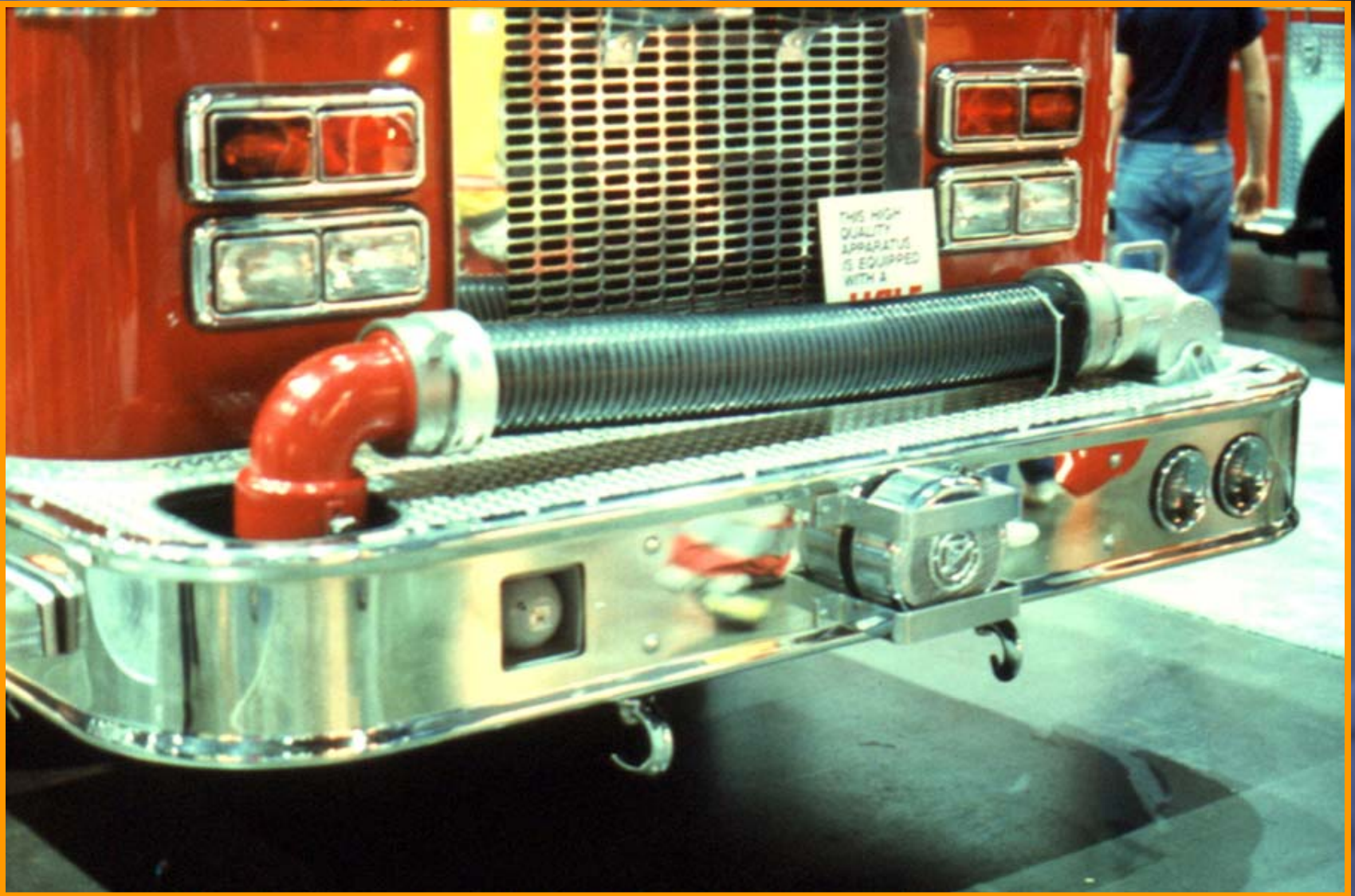
Figure 6. A 6' length of suction hose is better than a 10' length, but the water still has to travel through about 100 feet of pipe to get to the pump.
