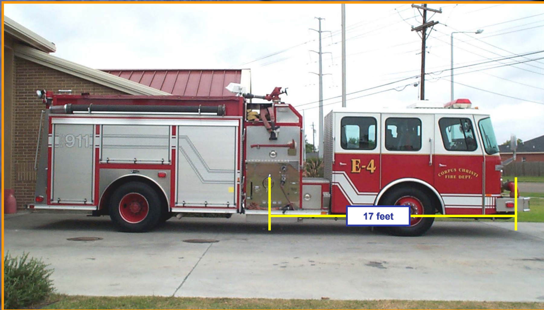
Figure 7. A side view of the Corpus Christi (Texas) engine with front suction and a preconnected 5" supply line in front bumper. The straight line distance from the front suction connection to the pump is 17 feet.
