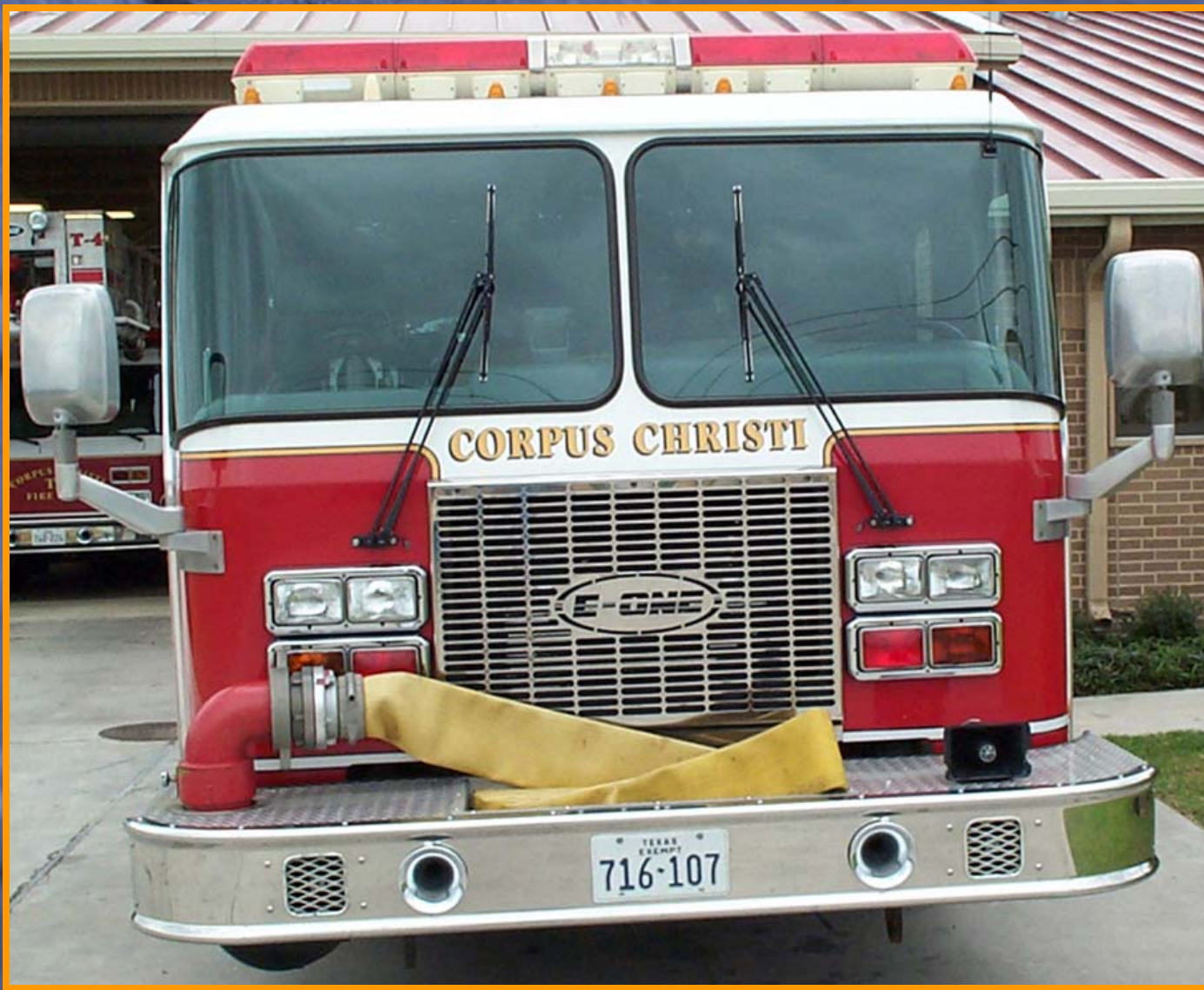
Figure 5. An urban engine with a typical front suction and a preconnected 5" supply line.
