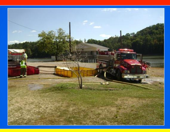
The pumper did a nice job of managing a three-dump tank set-up including multiple jet siphons and a master stream device.
