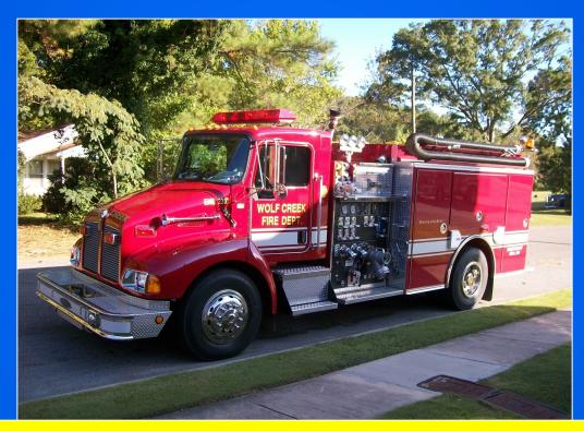
Engine 2352 is one of Pierce's "affordable" line of pumpers built on a commercial chassis. Although small in appearance, the rig's 1,250 gpm pump and 1,000 gallons of water make it a very effective pumper in "small town America."
