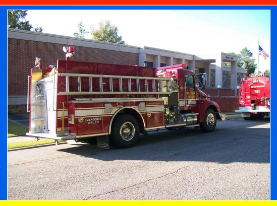
One thing for rural FDs to consider is the addition of extra suction hose. This photo is a good example of how another 10-ft could be mounted above the ground ladder. Or...better yet, move the ladder up some and mount 10-ft of suction below the ladder.
