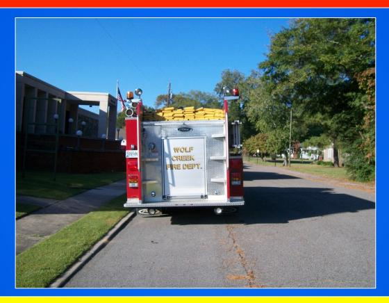
The use of 4-inch LDH makes a big difference in terms of the pumping ability of this 1,250 gpm pumper. Engine 2352 should be able to easily exceed its rated capacity when using the LDH.
