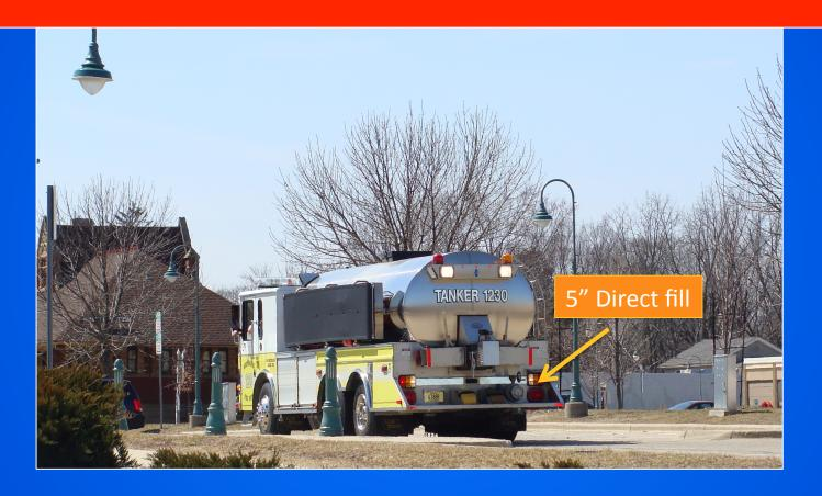
The 5-inch direct fill line is part of a standardized fill requirement for tankers operating in the mutual aid group.
