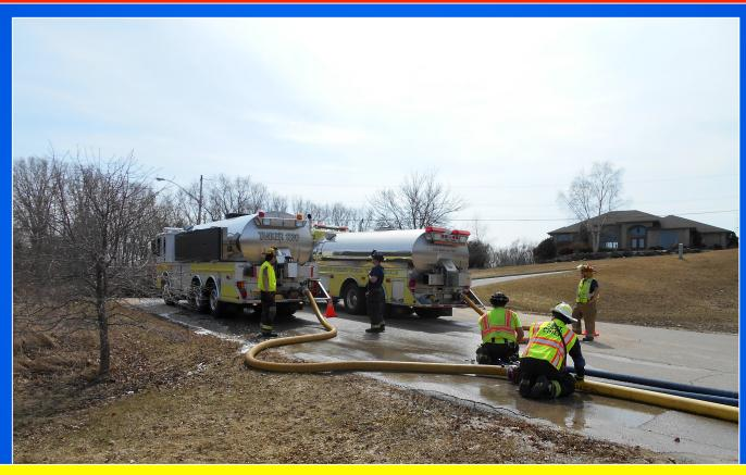
The "real" performance feature of Tanker 1230 is its ability to fill at a rate in excess of 1,000 gpm by using the 5-inch direct fill line. The tanker is shown here being filled using 5-inch LDH.
