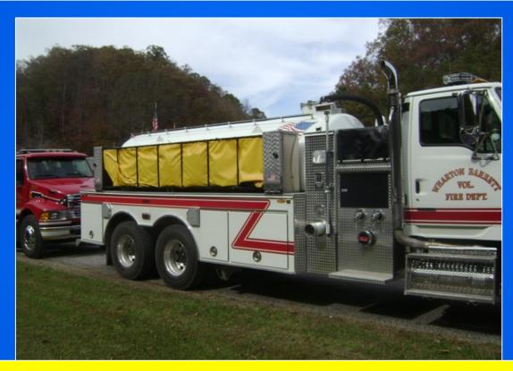
The dual, 3,500-gallon dump tanks are another important feature of this vacuum tanker. One dump tank is used at the dump site and one can be used at the fill site.
