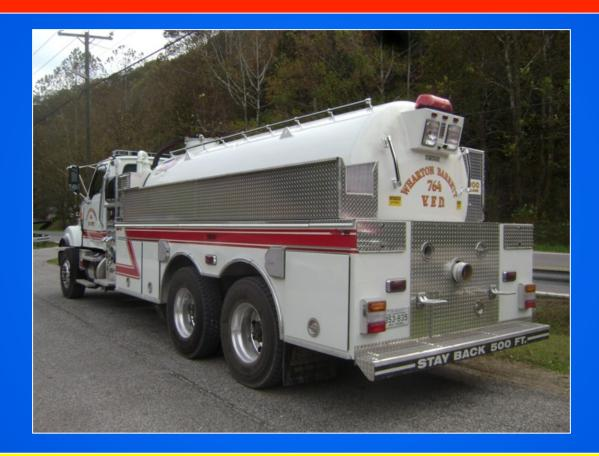
Tanker 764's 3,000 gallons of water can make a huge impact during initial fire attack operations.
