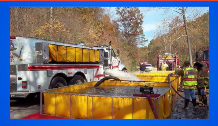
Tanker 764 is shown offloading at a 2011 water supply drill where 1,000 gpm was sustained using vacuum tankers.
