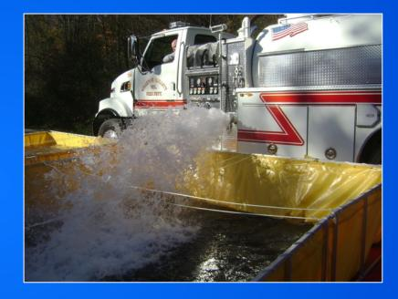
With the tank pressurized, water is off-loaded well in excess of 1,000 gpm making this vacuum tanker quite a water hauler!
