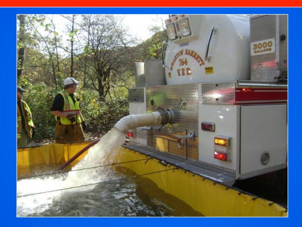
If needed, the vacuum tanker can also off-load via the rear dump.
