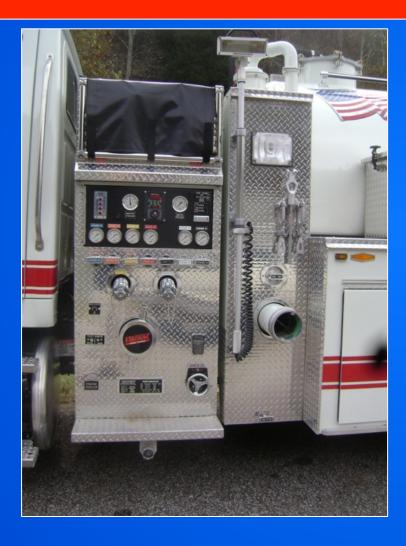
The tanker is equipped with a 1,000 gpm pump that is PTO driven. The addition of a regular fire pump to a vacuum tanker permits more variation in the use of the rig and also adds pump capacity to the FD. The added pump capacity may help meet the community's ISO Basic Fire Flow need.
