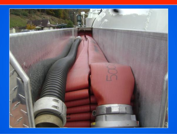
The tanker also carries a limited quantity of LDH and attack line – this allows it to function as a pumper if needed – just in limited capacity.
