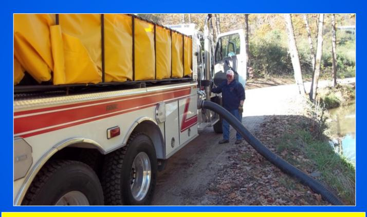
Perhaps the most important feature of a vacuum tanker is its ability to self-load – driver only if needed. And of course...no need for a pumper at the fill site. Tanker 764 self-loads at well-over 1,000 gpm.
