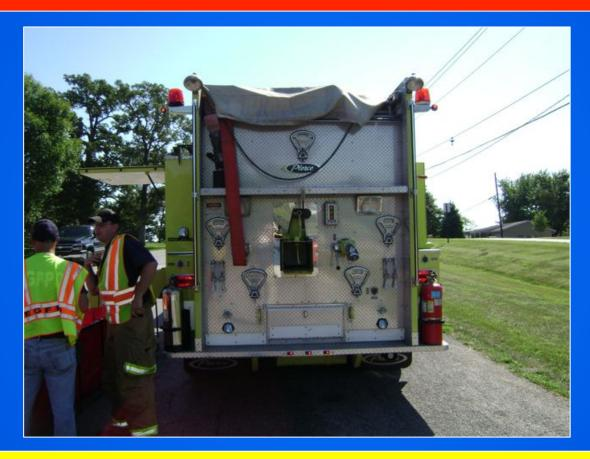
The 2,500-gallon engine/tanker has a single, 2-1/2-inch direct fill line. A larger direct fill line would be nice – it would improve filling time.
