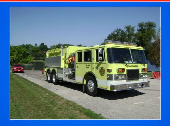
Engine 4 is well-equipped to function as a first-arriving pumper or as a water hauling tanker.
