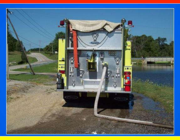
As with most any tanker, LDH is the preferred means by which to reduce fill times. Although, if the length is kept short, 3-inch hose can meet the 1,000 gpm fill rate goal.
