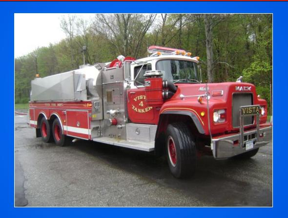
The rig carries a 3,500-gallon dump tank and also has an 8-inch round dump in the "tear drop" area on both sides of the body.
