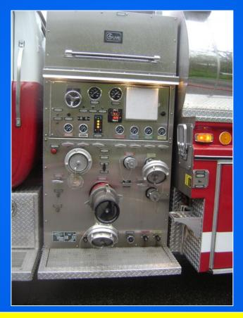
The tanker's single-stage, 1,500 gpm Hale pump is equipped to handle 5-inch hose on its intake and discharges making it versatile in several aspects.
