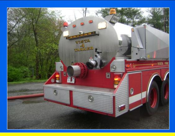
Tanker 4 has a 12" round dump on the rear as well as a 5" direct fill line which really reduces fill time – thus getting the tanker back on the road to the dump site.
