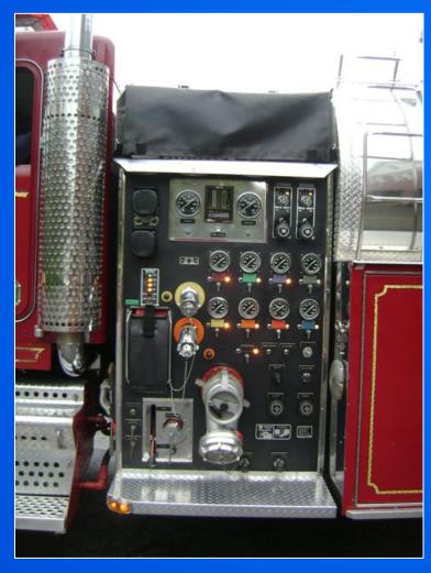
The rig's 1,500 gpm Darley pump is set-up to handle 5-inch hose as both a supply line and a discharge line. This size pump provides versatility in operation as a supply pumper, a relay pumper, or a nurse tanker.
