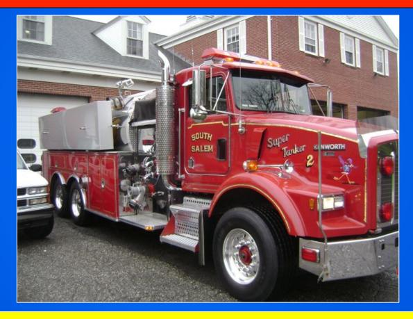
The tanker carries a 3,300-gallon dump tank. Note the LDH discharge on the officer side pump panel and the 6-inch round dump just ahead of the tandem wheels.
