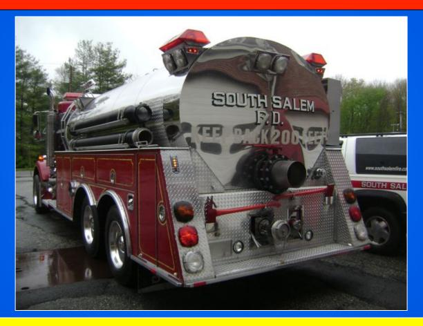
Tanker 2 has a 10-inch round dump and a 5-inch direct fill line – both allow for quick turn-around times at the dump site and fill site.
