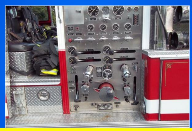
Even though the pumper's capacity is rated at 1,000 gpm, when operating as an "in-line" relay pumper, it is capable of supporting much higher flows.
