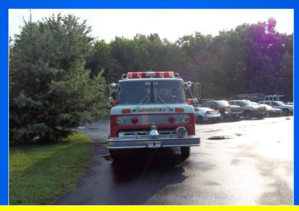
The E-One pumper is built on a Ford C-series chassis and is powered by a Caterpillar motor.
