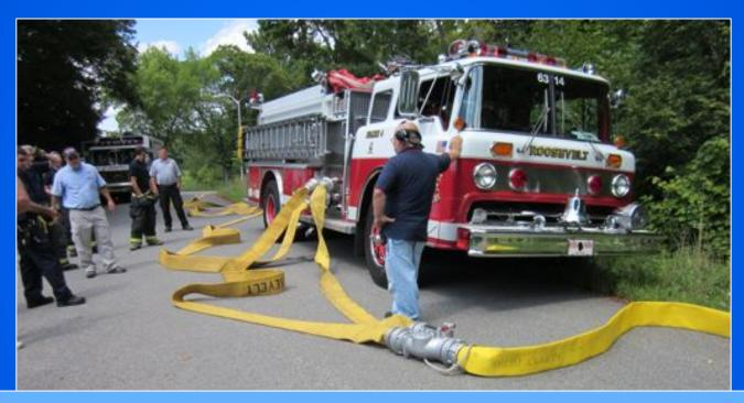
Using this set-up (August 2012 drill) the total flow for the 5,100-ft relay of 5-inch LDH using just three pumpers was 1,016 gpm. With five pumpers – 1,500 gpm. View the results of the drill at:
