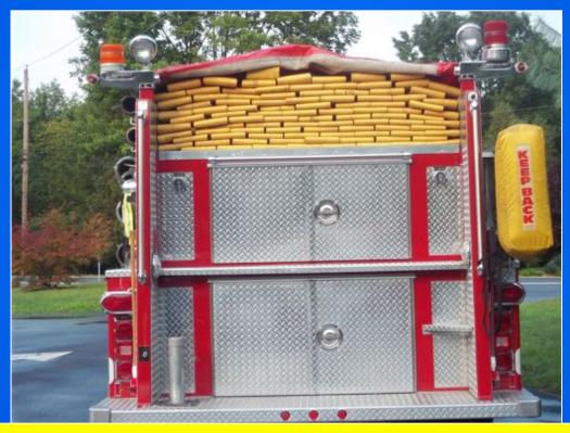
Engine 63-14 carries 3,000 feet of 5-inch supply hose plus various LDH appliances and adaptors to support water supply operations in the mutual aid response area.
