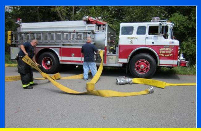
The crew operates the pumper as the middle-pumper in a three-pumper relay operation.
