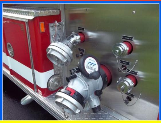
With no high-flow discharge, the pumper is challenged to "get rid of" all the water that comes into the pump. However, the rig is set-up to support a clappered siamese operation that uses two pump discharges.
