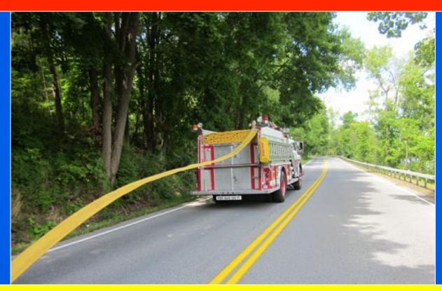
Engine 63-14 is shown laying out its 3,000 feet of supply hose at the August 2012 drill. The photo makes it look like the pumper is going 70 mph – it is not. The photo frame caught once moment in time where the hose was coming out of the hose bed.
