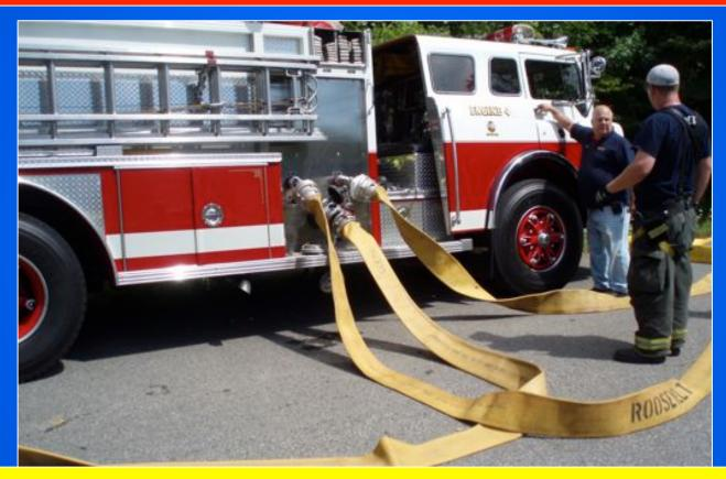
Two discharges are used to supply a double-clappered siamese into a single, 5-inch supply line to the attack pumper.
