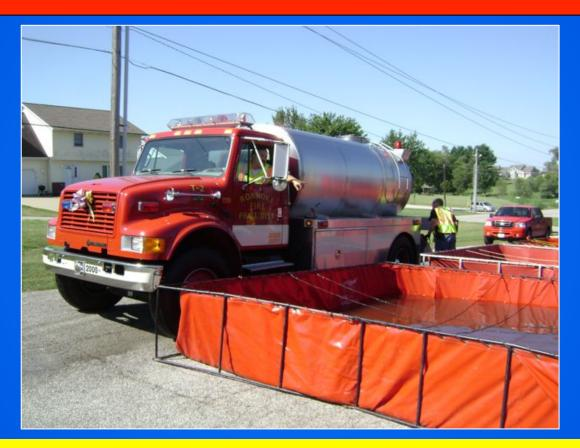
The elliptical tank provides for a better center of gravity while still taking advantage of head pressure for dumping operations.
