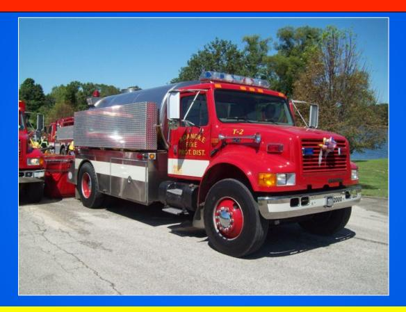
Tanker 2 is set-up to work as a "pure" water hauling rig. Its short wheel base allows for maneuverability and its smaller tank allows for quick runs.
