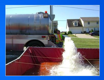
Tanker 2 is shown above offloading water at a water supply drill in nearby Deer Creek. The elbow attachment allows the tanker to dump its water off of the side instead of having to maneuver into position to use the rear dump.
