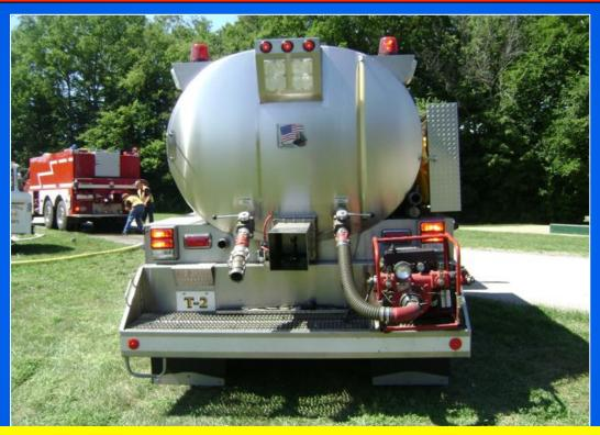
Tanker 2 is set-up to dump off of the rear of the rig. An elbow attachment is available for side dumping. The unit carries a portable pump connected to the direct fill – this arrangement will support fire flows up to about 250 gpm.
