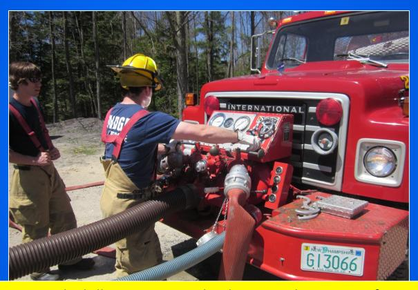
At this water supply drill in May 2013, the driver used a section of 2-1/2" (pony) hard sleeve to increase pump capacity in order to support the 1,000 gpm flow and operate jet siphons.
