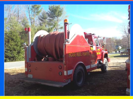
3,300-feet of 4-inch LDH is carried on one large hose reel. This area of New England is historically known for the use of LDH on large hose reels. The reel is powered to assist with reloading and it also has braking control to protect against over-speed when deploying.
