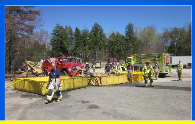
26-Reel-1 was used as the dump site pumper at the 2013 water supply drill. The original plan did not have the pumper serving in such capacity – however, as in real life (sorry about the pun), the reel pumper had to do that job!
