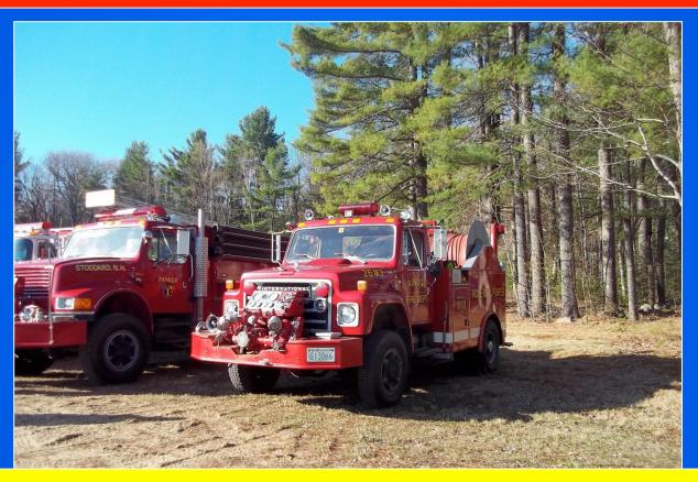
The hose reel pumper is outfitted with a Hale 1,000 gpm front mount pump. The front mount design is popular in rural environments because it allows the driver/operator to "nose up" to a static water source for drafting.
