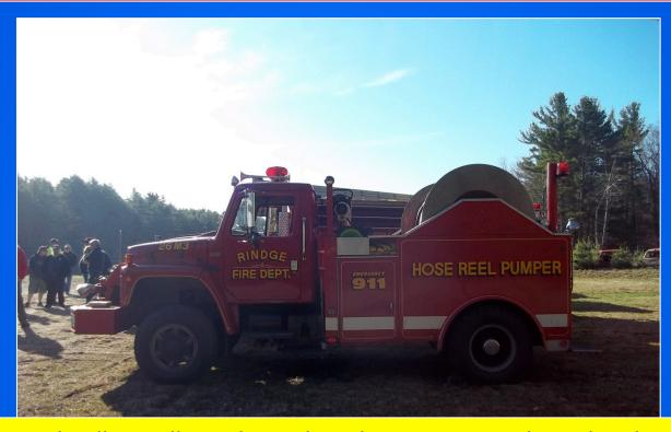
The short wheelbase allows the reel truck to maneuver through tight spaces in order to get to a water supply source or a fire scene. The unit is set up to either conduct a forward lay or reverse lay depending on the water supply needs at the incident scene.
