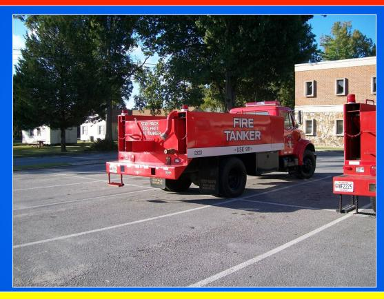
Carrying two dump tanks is a unique feature not often seen on a traditional tanker. The two tanks certainly make the rig more versatile in terms of helping out at dump sites AND fill sites.
