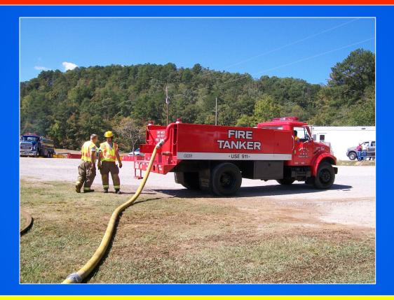
The 4-inch direct fill means this tanker can load fast and get back on the road hauling water.
