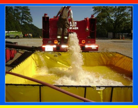
Tanker 8065 is shown here dumping water at a 2010 water supply drill. Its ability to load and off-load fast make it a great little water hauling unit!!!
