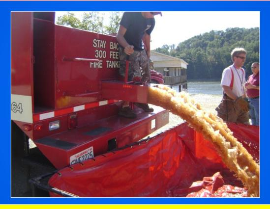
The rectangular dump chute/valve on Tanker 8064 is a rather unique feature on this tanker.
