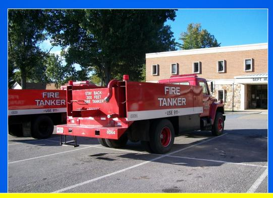
Carrying two dump tanks is a unique feature not often seen on a traditional tanker. The two tanks certainly make the rig more versatile in terms of helping out at dump sites AND fill sites. Plus, the 4-inch direct fill allows this tanker to load fast and get back on the road!
