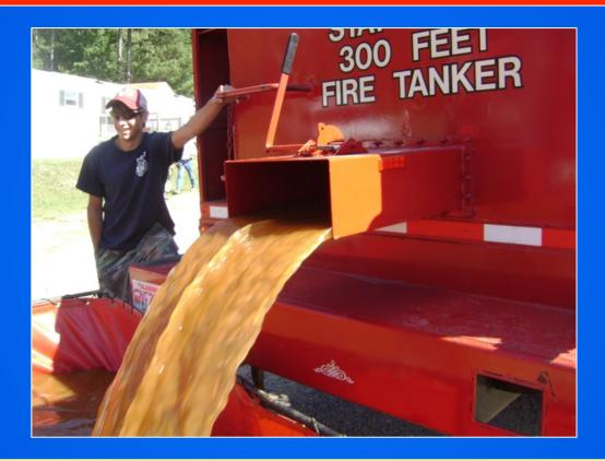
We have seen this style of dump on a tanker from Chile; this is the first time we have seen one on a U.S. tanker.
