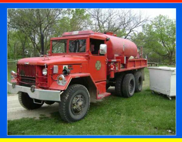
This all-wheel drive tanker will go just about anywhere and its 10-inch side dump lets it offload all of its water in about 60 seconds!
