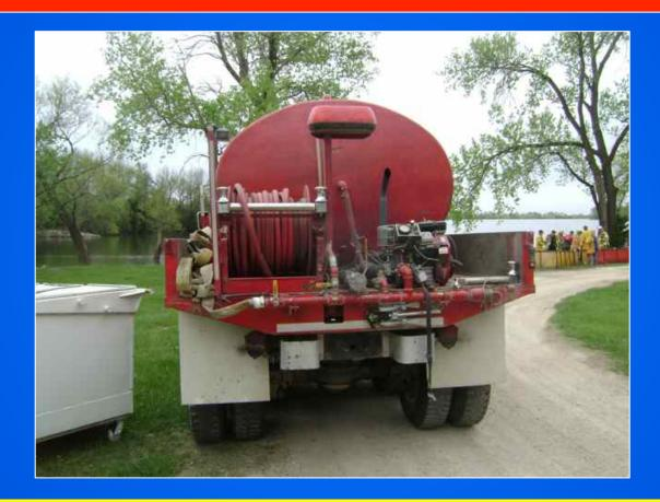
Brush Tanker 3 is equipped with a small pump and a couple of attack lines that can be used for fighting prairie fires.
