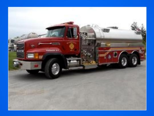
Tanker 5-7 is a large capacity tanker set up to operate as a water hauling unit in a tanker shuttle operation or as a nurse tanker in an initial attack operation.
