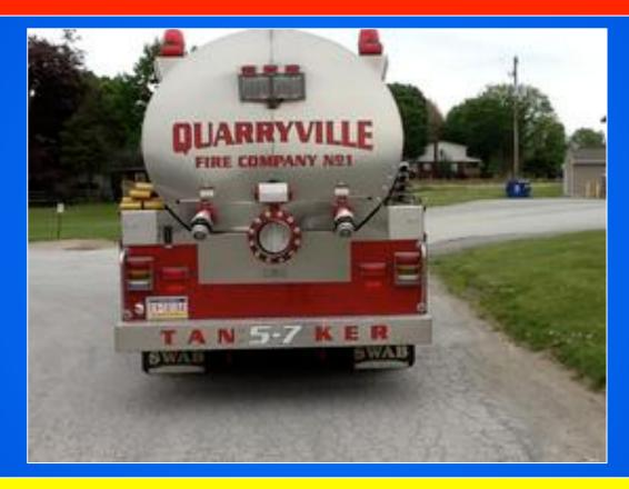
The "business end" of the tanker is equipped with a 12" round dump and two, 3-inch direct fill lines.
