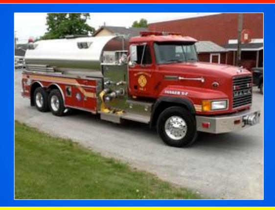
The tanker does not carry a dump tank because it often operates as a nurse tanker. The rig is also equipped with two, pre-connected attack lines and a pre-connected, 4-inch discharge line.
