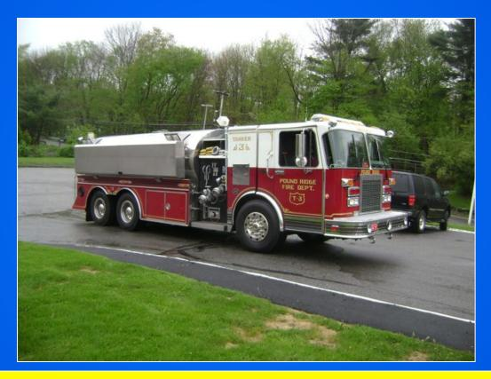
Tanker 3 is equipped with 8" round dumps behind the tandem wheels on both sides of the body. It also carries a 3,000-gallon dump tank.
