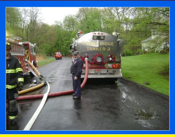
The tanker has a 12" round dump and dual, 4" direct fills on the rear of the rig.
