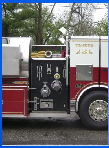
The tanker is also equipped with an LDH discharge – again – a handy fixture when working as a nurse tanker or a relay pumper.
