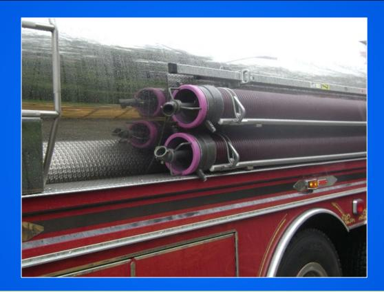
The tanker carries jet siphons pre-connected to its 6-inch suction hose. We like this idea – saves time – quicker set-up.
