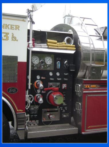
The rig is outfitted with a 1,000 gpm Waterous pump and carries a minimal amount of hose. Note the use of an external control valve on the suction intake – it is a hand-operated butterfly valve – often referred to as a "keystone" valve.
