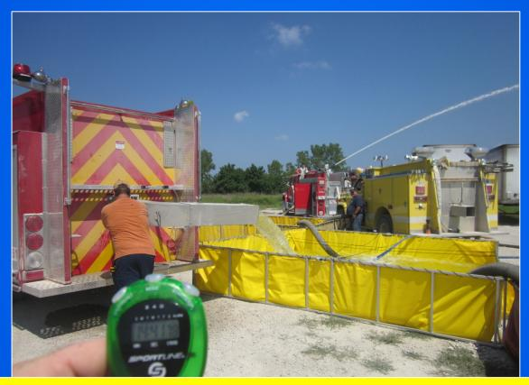
Tanker 3361 is shown here dumping its 3,000 gallons of water at a drill in nearby Ottawa.
