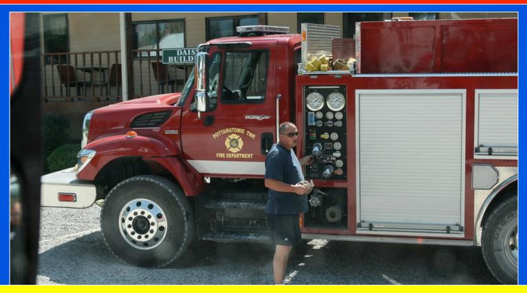
Tanker 3361 has a 750 gpm PTO-driven fire pump and is equipped with a couple of pre-connected attack lines. The tanker does not have a rear tank fill – but has a side-mounted direct tank fill on the pump panel.
