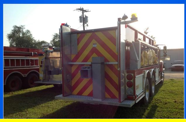
The tanker has a 10-inch rear dump and a detachable chute that is used to allow the tanker to dump water off of either side – which also allows compliance with NFPA 1901 for a Mobile Water Supply Apparatus.
