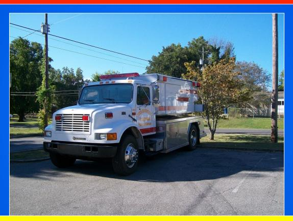
Tanker 1462 is set up to operate as a water hauling unit in a tanker shuttle operation. It has a 250 gpm pump for small scale operational support such as brush/woods fires.
