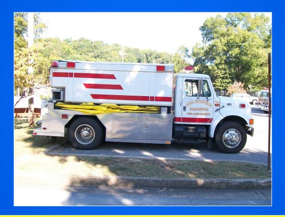
Tanker 1462 carries a 2,000-gallon dump tank in a low position on the unit for easy deployment.
