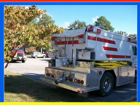
The rear end of Tanker 1462 is the "business" end of the unit. The rig can dump off either side or rear and the 4-inch direct fill makes for a quick turnaround time at the fill site.
