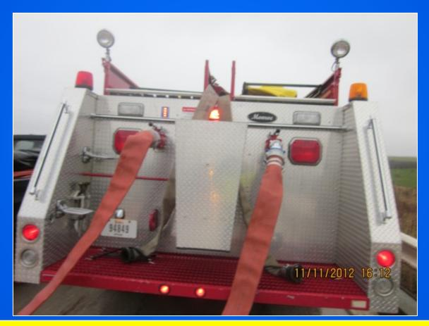
Dual, 4-inch hose lines were used at the Stanley drill to fill the tanker.
