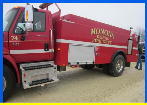
Perhaps the most unique feature of the tanker is its tilting tank. Hydraulic pistons (similar to a tilt cab set-up) raise the tank about one foot which aides in a "faster" offload of water when the tank level gets low..
