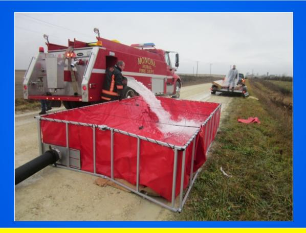
The tanker is equipped with 10-inch side and rear dumps thus allowing it to offload water very fast.
