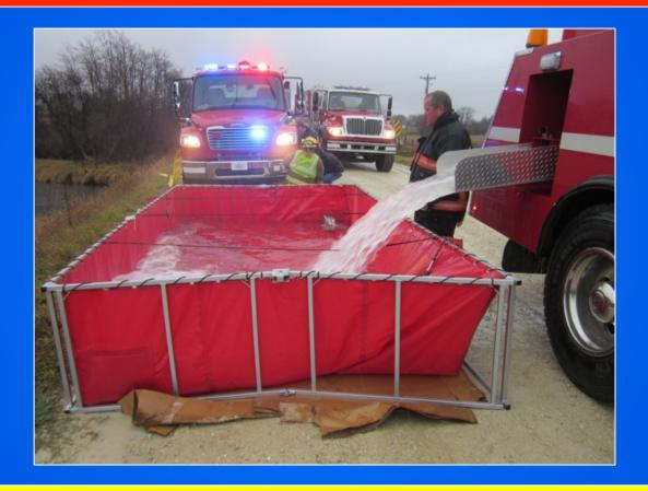
Tanker 14 is shown dumping water from one of its side dumps at a recent drill in nearby Stanley, Iowa.
