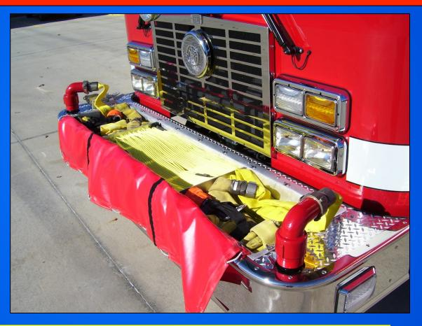
The front bumper compartment is equipped with two, 200-ft, 1-3/4-inch attack lines plus 100-ft of 1-inch forestry hose.
