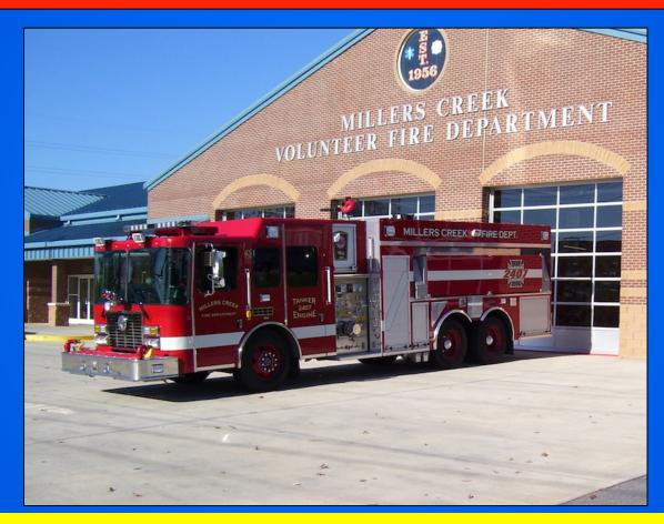
This engine/tanker is equipped with a Hale QMax 2,250 gpm pump but the rig is rated at 1,500 gpm. It also has no driver side discharges.
