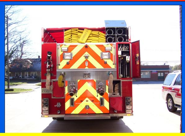
Besides the 2,000-ft split bed of 5-inch supply line, the engine/tanker also carries two, 10-ft and two, 18-ft sections of suction hose and has a preconnected portable master stream device and a pre-piped deck gun.
