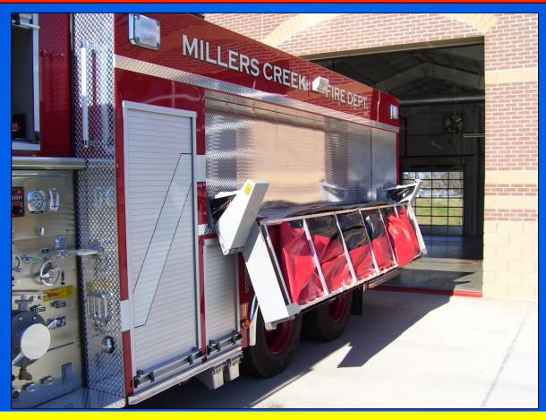
The unit carries a 3,000-gallon portable dump tank on the driver's side..
