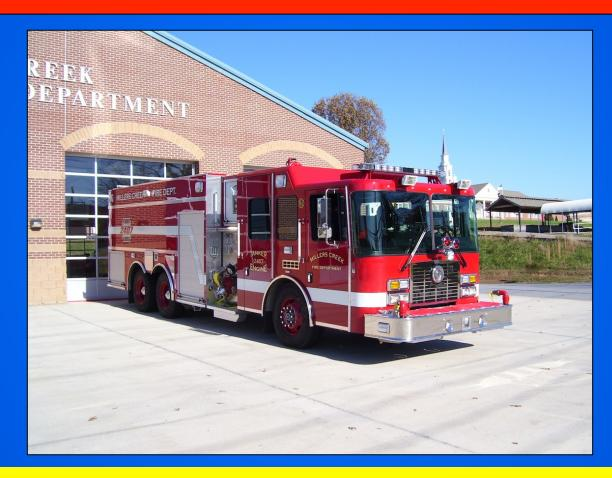
ET2407 has a 4-inch, high-flow discharge on the officer's side and carries a full complement of engine company equipment.
